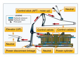
Figure 6-2. Hydromechanical flight control system.
