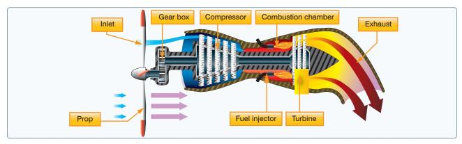
Figure 7-24. Turboprop engine.
