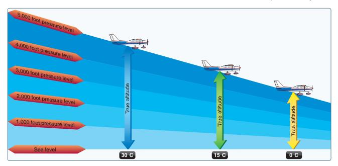
**Figure 8-3.** *Effects of nonstandard temperature on an altimeter.*
