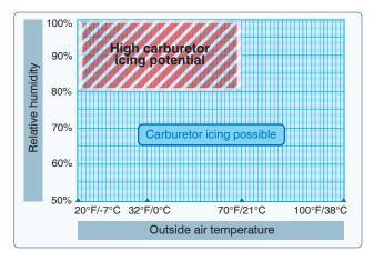
**Figure 7-12.** Although carburetor ice is most likely to form when the temperature and humidity are in ranges indicated by this chart, carburetor icing is possible under conditions not depicted.
