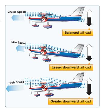
Figure 5-24. Effect of speed on downwash.
