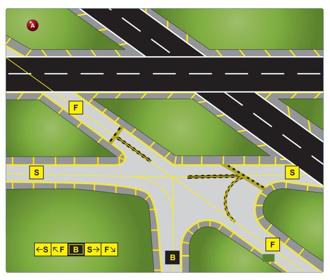
**Figure 14-20.** Orientation of signs is from left to right in a clockwise manner. Left turn signs are on the left and right turn on the right. In this view, the pilot is on Taxiway Bravo.
