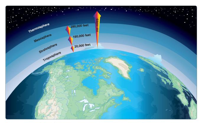
Figure 12-2. Layers of the atmosphere.
