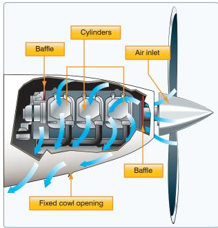
**Figure 7-19.** *Outside air aids in cooling the engine.*
