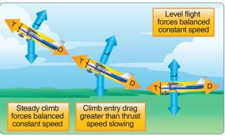
**Figure 5-37.** *Changes in speed during climb entry.*
