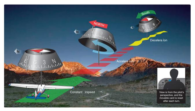
Figure 8-37. The effects of acceleration error.
