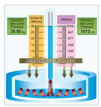
Figure 4-2. Standard sea level pressure.
