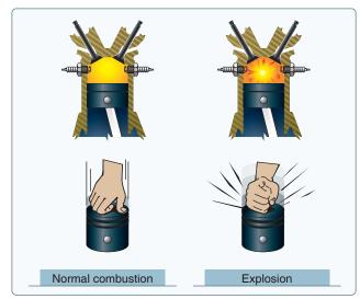
Figure 7-21. Normal combustion and explosive combustion.
