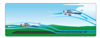
**Figure 5-16.** *Ground effect changes airflow.*
