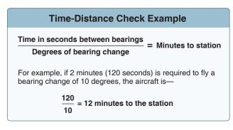
**Figure 16-33.** *Time-distance check example.*
