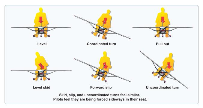
Figure 17-6. Sensations from centrifugal force.
