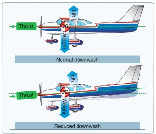
**Figure 5-25.** *Reduced power allows pitch down.*
