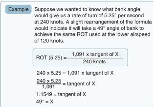
**Figure 5-58.** To achieve the same rate of turn of an aircraft traveling at 120 knots, an increase of bank angle is required.
