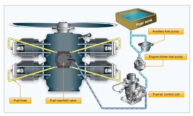
Figure 7-13. Fuel injection system.
