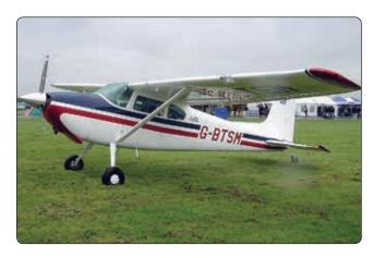
Figure 7-38. Tailwheel landing gear.
