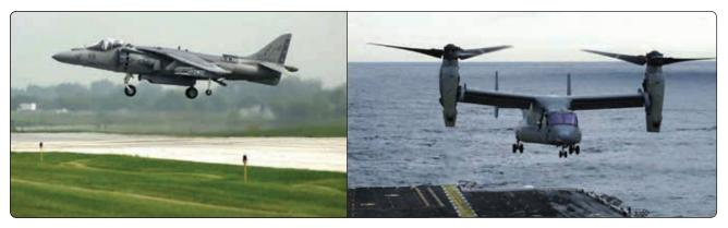
**Figure 5-4.** *Some aircraft have the ability to change the direction of thrust.*
