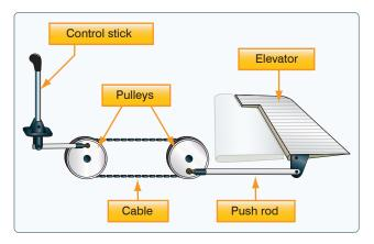
Figure 6-1. Mechanical flight control system.
