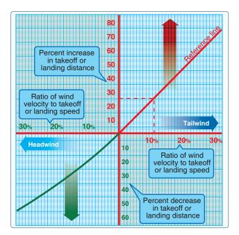
**Figure 11-19.** *Effect of wind on takeoff and landing.*
