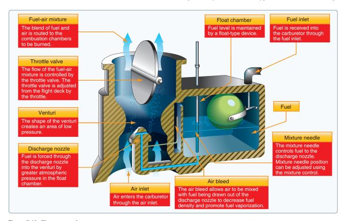
Figure 7-10. Float-type carburetor.
