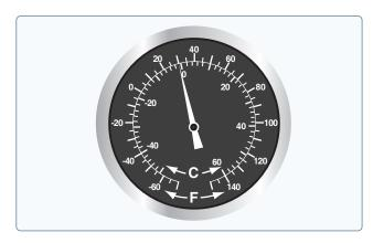
**Figure 8-39.** *Outside air temperature (OAT) gauge.*
