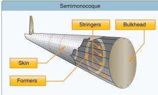
Figure 3-14. Semimonocoque and monocoque fuselage design.
