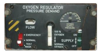
Figure 7-43. Oxygen system regulator.
