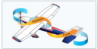
Figure 5-48. Corkscrewing slipstream.
