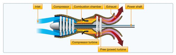
Figure 7-26. Turboshaft engine.
