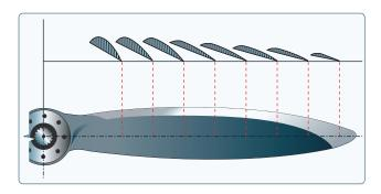
Figure 7-6. Changes in propeller blade angle from hub to tip.
