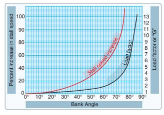
Figure 5-39. Increase in stall speed and load factor.
