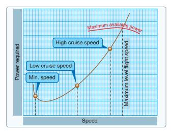
Figure 11-6. Power versus speed.
