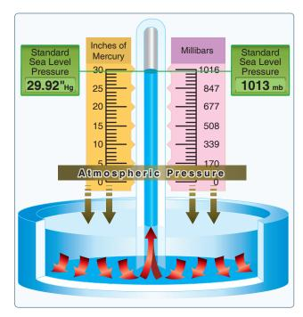
Figure 11-1. Standard sea level pressure.
