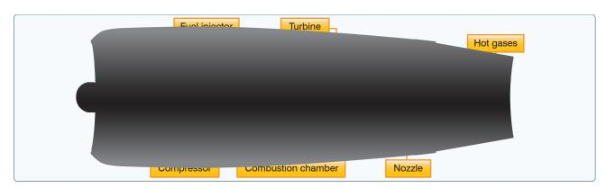
Figure 7-23. Turbojet engine.
