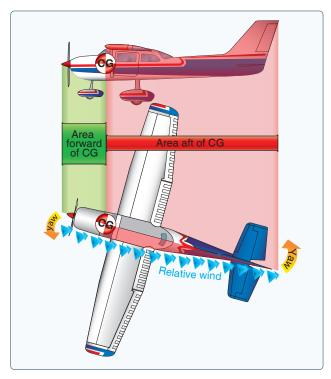
**Figure 5-32.** *Fuselage and fin for directional stability.*
