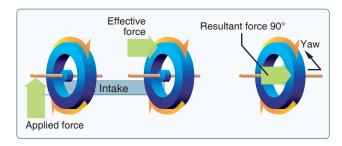
Figure 5-49. Gyroscopic precession.
