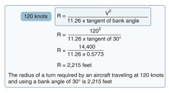
**Figure 5-59.** *Radius at 120 knots with bank angle of 30*°.
