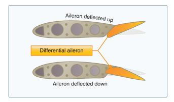
Figure 6-6. Differential ailerons.
