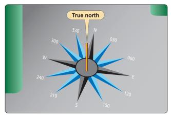
**Figure 8-34.** *Utilization of a compass rose aids compensation for deviation errors.*
