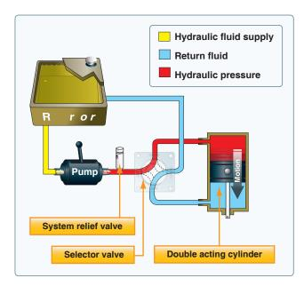
Figure 7-36. Basic hydraulic system.
