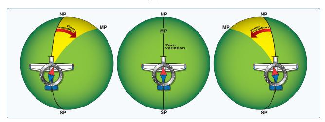
**Figure 16-10.** *Effect of variation on the compass.*
