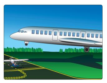
**Figure 14-51.** Do NOT cross a runway holding position marking without ATC clearance. If the tower is closed or you are operating from a non-towered airport, check both directions for conflicting traffic before crossing the hold position marking.
