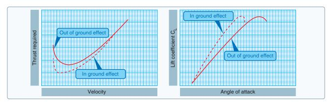
Figure 5-17. Ground effect changes drag and lift.
