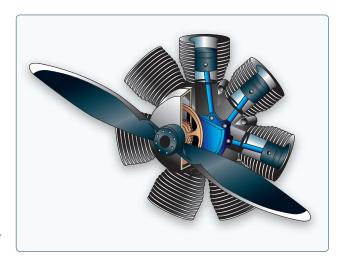
Figure 7-1. Radial engine.
