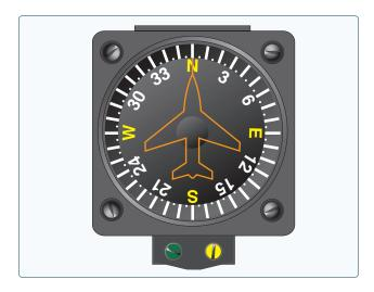
Figure 8-38. Vertical card magnetic compass.
