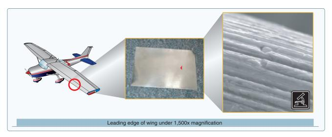
Figure 4-1. Microscopic surface of a wing.
