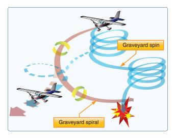
Figure 17-5. Graveyard spiral.
