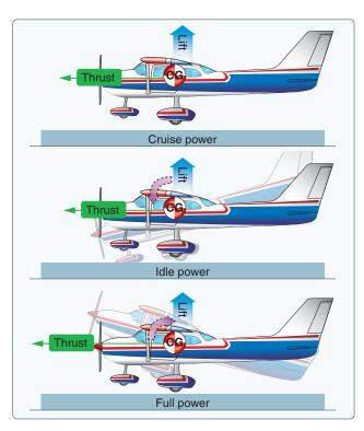
**Figure 5-27.** *Power changes affect longitudinal stability.*
