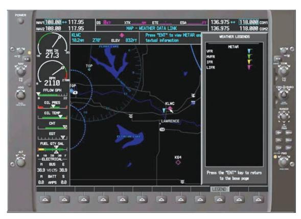
Figure 13-21. *Graphical METAR legend display*.
