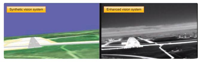
Figure 17-23. Synthetic and enhanced vision systems.
