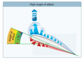
**Figure 4-7.** Pressure distribution on an airfoil and CP changes with AOA.
