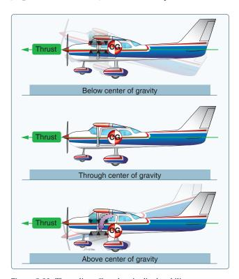
**Figure 5-26.** Thrust line affects longitudinal stability.
