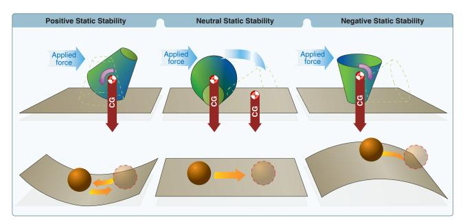
Figure 5-21. Types of static stability.
