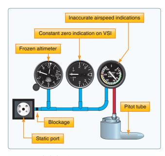
Figure 8-11. Blocked static system.
