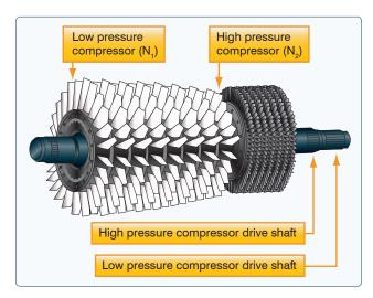
Figure 7-27. Dual-spool axial-flow compressor.
