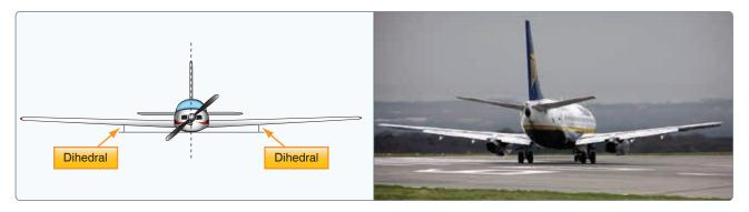
Figure 5-28. Dihedral is the upward angle of the wings from a horizontal (front/rear view) axis of the plane as shown in the graphic depiction and the rear view of a Ryanair Boeing 737.
