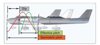
Figure 5-45. Propeller slippage.
