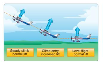
Figure 5-36. Changes in lift during climb entry.
