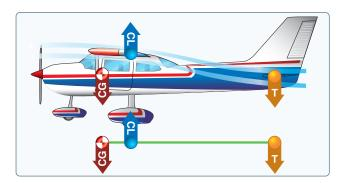
Figure 5-23. Longitudinal stability.
