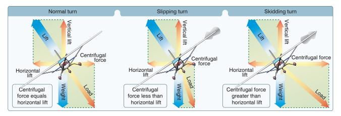
Figure 5-35. Normal, slipping, and skidding turns at a constant altitude.
