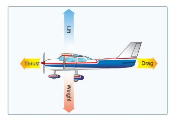
**Figure 5-1.** *Relationship of forces acting on an aircraft.*
