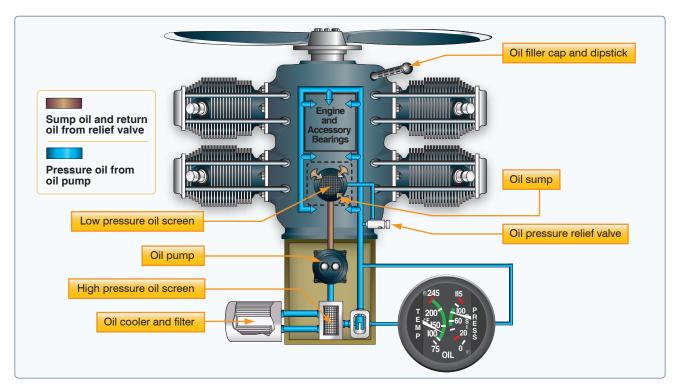
Figure 7-17. Wet-sump oil system.
