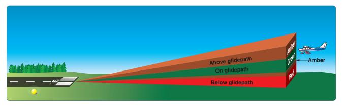
**Figure 14-31.** *Tri-color visual approach slope indicator.*
