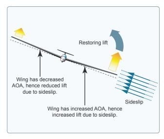
Figure 5-29. Sideslip causing different AOA on each blade.
