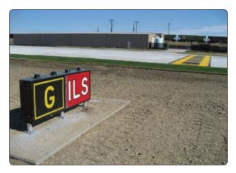
**Figure 14-24.** Instrument landing system (ILS) holding position sign and marking on Taxiway Golf.
