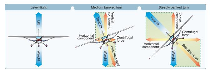
Figure 5-34. Forces during normal, coordinated turn at constant altitude.
