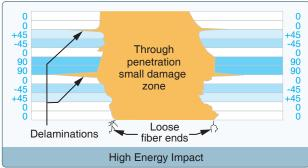
**Figure 3-16.** Impact energy affects the visibility, as well as the severity, of damage in composite structures. High and medium energy impacts, while severe, are easy to detect. Low energy impacts can easily cause hidden damage.
