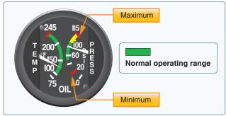
**Figure 9-3.** *Minimum, maximum, and normal operating range markings on oil gauge.*
