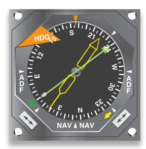
Figure 16-31. Radio magnetic indicator.
