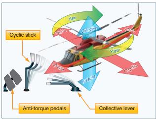
**Figure 6-3.** *Helicopter flight control system.*
