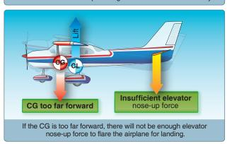
**Figure 3-3.** *Center of gravity (CG).*
