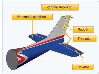
Figure 3-10. Empennage components.
