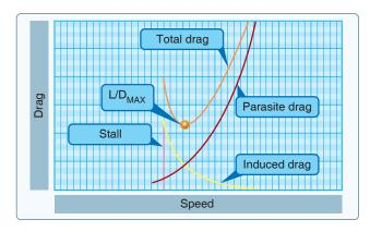
Figure 11-5. Drag versus speed.
