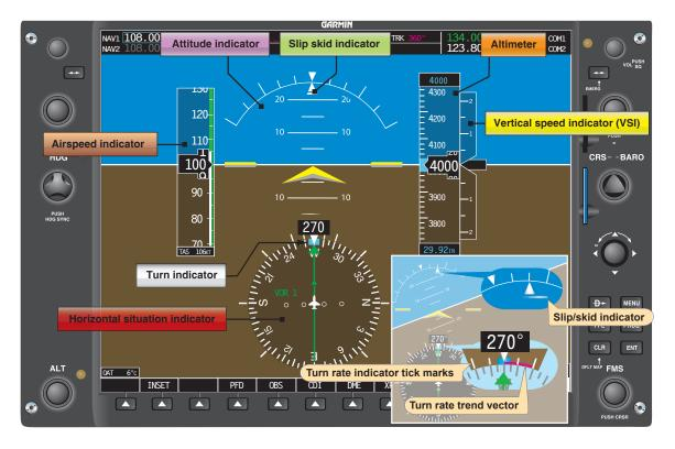
Figure 8-12. Primary flight display (PFD). Note that the actual location of indications vary depending on manufacturers.
