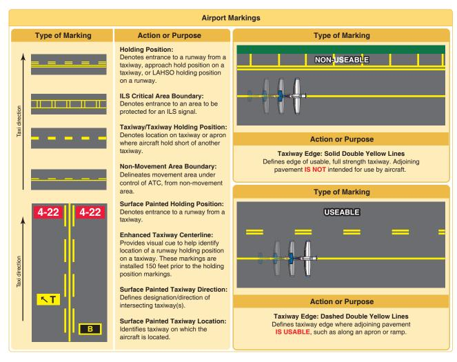
**Figure C-3.** *Samples and explanations of standard airport markings.*
