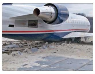
**Figure 14-57.** There have been several incidents where the EMAS has successfully arrested the aircraft.
