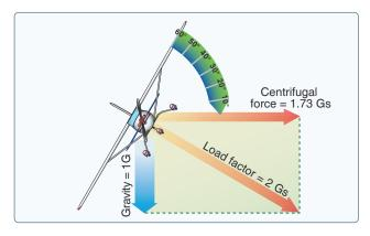
**Figure 5-52.** *Two forces cause load factor during turns.*
