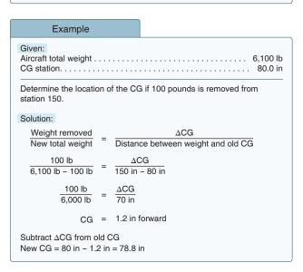
In the previous examples, the  $\triangle$ CG is either added or subtracted from the old CG. Deciding which to accomplish is best handled by mentally calculating which way the CG will shift for the particular weight change. If the CG is shifting aft, the  $\triangle$ CG is added to the old CG; if the CG is shifting forward, the  $\triangle$ CG is subtracted from the old CG.
