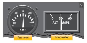
Figure 7-35. Ammeter and loadmeter.
