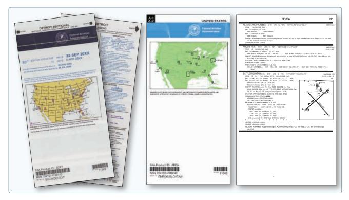
**Figure 1-18.** From left to right, a sectional VFR chart, IFR chart, and chart supplement U.S. (formerly Airport/Facility Directory) with a sample of a page from the supplement.
