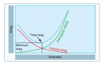
Figure 5-6. Drag versus speed.
