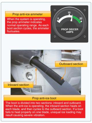
Figure 7-50. Prop ammeter and anti-ice boots.
