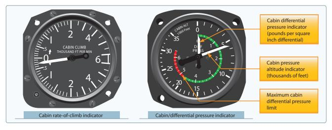
**Figure 7-42.** *Cabin pressurization instruments.*
