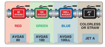
Figure 7-32. Aviation fuel color-coding system.
