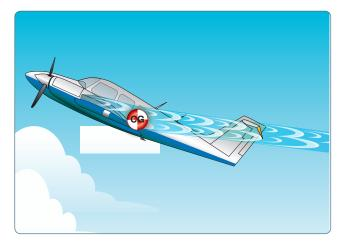
Figure 6-11. Aircraft with a T-tail design at a high AOA and an aft CG.
