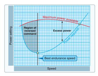
Figure 11-14. Power required curve.
