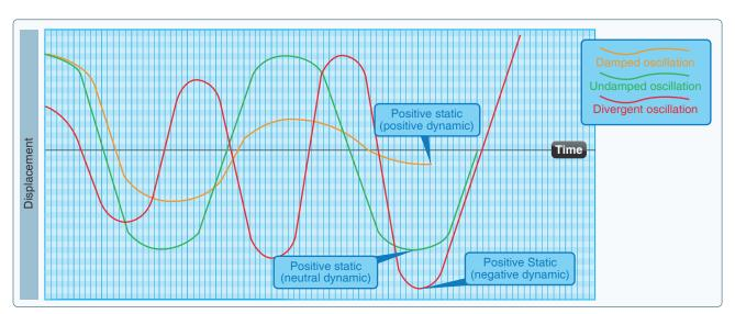
Figure 5-22. Damped versus undamped stability.
