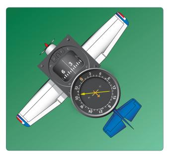
**Figure 16-37.** *ADF with fixed azimuth and magnetic compass.*
