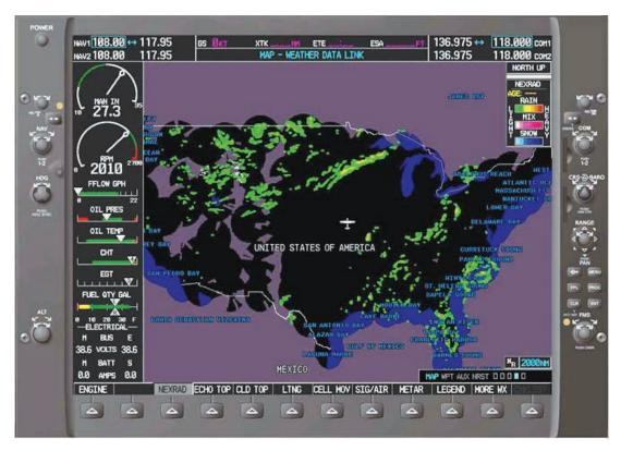
Figure 13-17. NEXRAD radar display.
