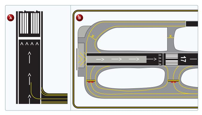
Figure 14-6. (A) Displaced runway threshold drawing. (B) Displaced threshold for Runway 17 at Albuquerque International Airport (ABQ).
