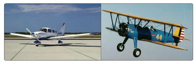
Figure 3-6. Monoplane (left) and biplane (right).
