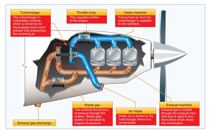
Figure 7-15. Turbocharger components.
