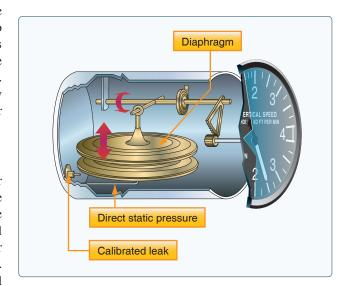
Figure 8-5. Vertical speed indicator (VSI).
