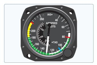
Figure 9-2. Multi-engine airspeed indicator.
