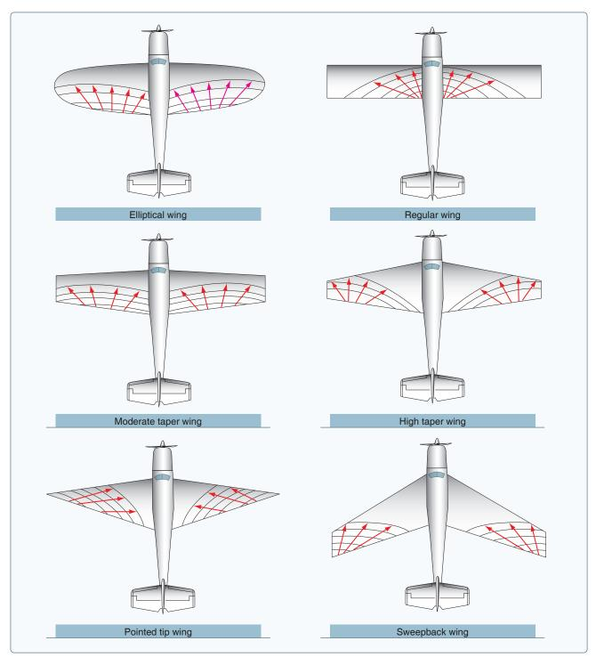
**Figure 5-33.** *Different types of wing planforms.*
