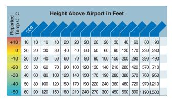
**Figure 8-4.** Look at the chart using a temperature of -10 °C and an aircraft altitude of 1,000 feet above the airport elevation. The chart shows that the reported current altimeter setting may place the aircraft as much as 100 feet below the altitude indicated by the altimeter.
