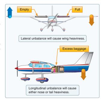
Figure 10-1. Lateral and longitudinal unbalance.
