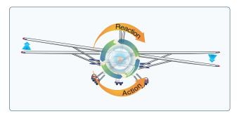
Figure 5-47. Torque reaction.
