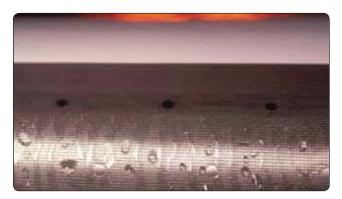
**Figure 7-49.** *TKS weeping wing anti-ice/deicing system.*
