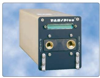
**Figure 8-15.** Teledyne's 90004 TAS/Plus Air Data Computer (ADC) computes air data information from the pitot-static pneumatic system, aircraft temperature probe, and barometric correction device to help create a clear picture of flight characteristics.
