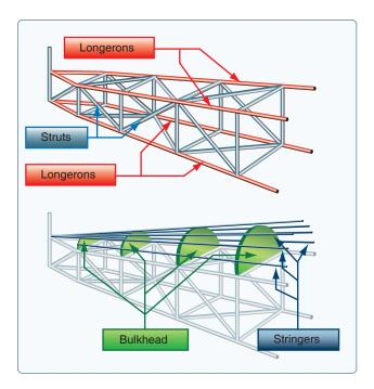
**Figure 3-5.** *Truss-type fuselage structure.*
