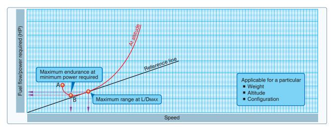
**Figure 11-11.** *Airspeed for maximum endurance.*
