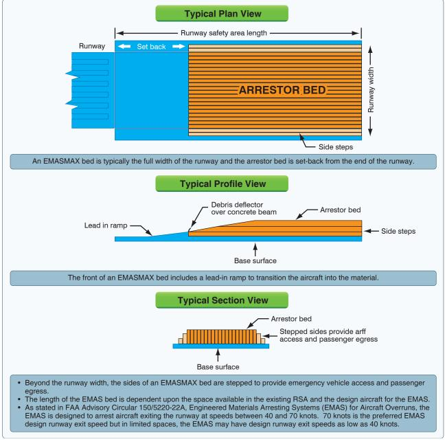
Figure 14-56. Diagram of an EMASMAX system.
