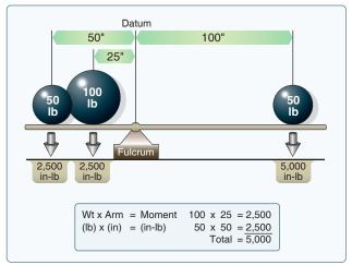
**Figure 10-4.** *Establishing a balance.*
