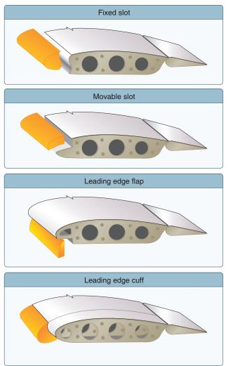
$\textbf{Figure 6-18.} \ \textit{Leading edge high lift devices}.$
