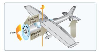
Figure 5-50. Raising tail produces gyroscopic precession.
