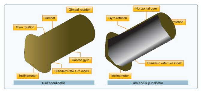
Figure 8-21. Turn indicators rely on controlled precession for their operation.
