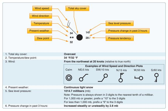
**Figure 13-11.** *Sample station model and weather chart symbols.*
