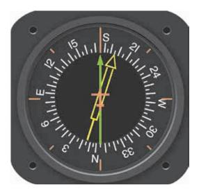
**Figure 8-30.** Driven by signals from a flux valve, the compass card in this RMI indicates the heading of the aircraft opposite the upper center index mark. The green pointer is driven by the ADF.
