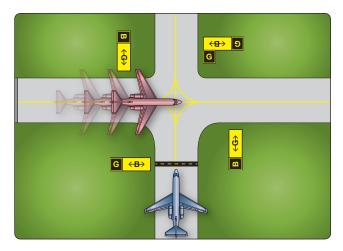
Figure 14-26. Holding position marking on a taxiway.
