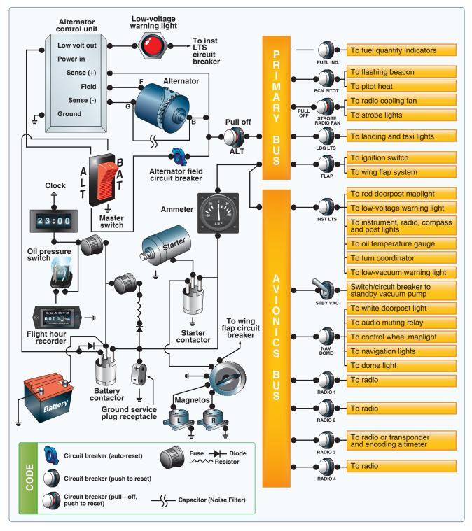
**Figure 7-34.** *Electrical system schematic.*
