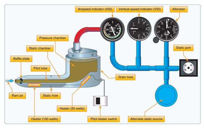
Figure 8-1. Pitot-static system and instruments.
