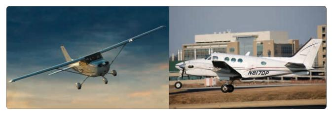
$\textbf{Figure 7-39.} \ \textit{Fixed (left) and retractable (right) gear airplanes}.$
