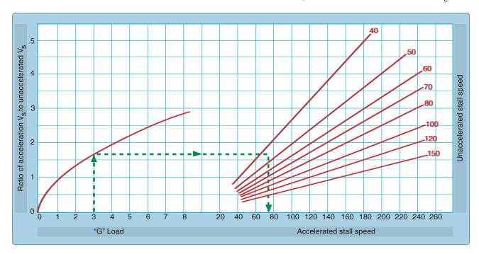
Figure 5-54. Load factor changes stall speed.
