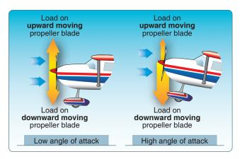
**Figure 5-51.** Asymmetrical loading of propeller (P-factor).
