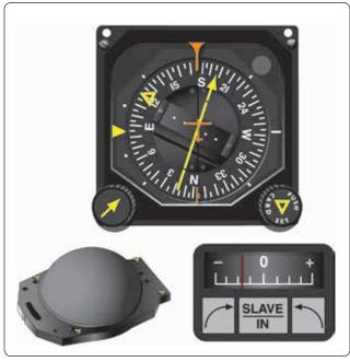
**Figure 8-29.** *Pictorial navigation indicator (HSI, top), slaving meter (lower right), and slaving control compensator unit (lower left).*
