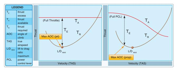
**Figure 11-8.** Comparison of maximum AOC between jet and propeller airplanes.
