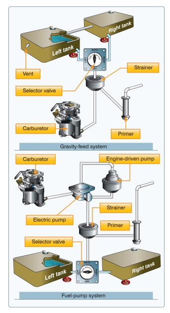
**Figure 7-30.** *Gravity-feed and fuel-pump systems.*
