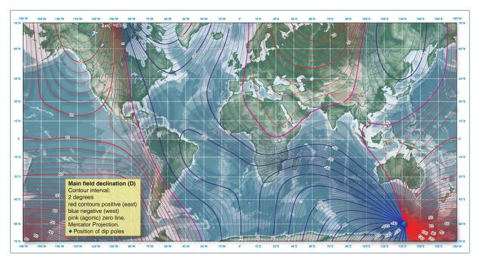
**Figure 8-33.** *Isogonic lines are lines of equal variation.*
