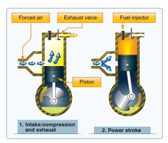
Figure 7-3. Two-stroke compression ignition.
