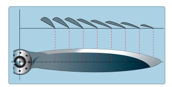
Figure 5-43. Airfoil sections of propeller blade.
