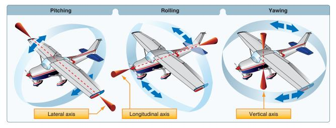
**Figure 5-18.** *Axes of an airplane.*
