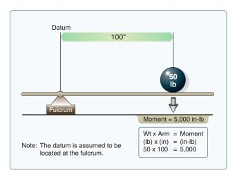
Figure 10-3. Determining moment.
