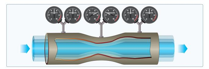
Figure 4-4. Air pressure decreases in a venturi tube.
