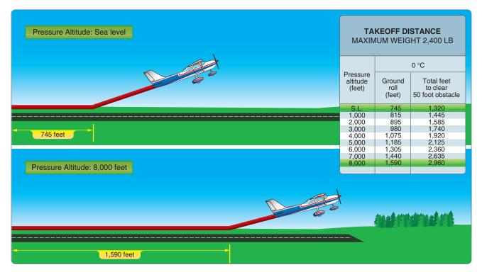
**Figure 12-9.** *Takeoff distances increase with increased altitude.*
