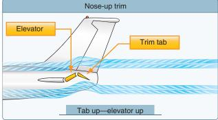
**Figure 6-20.** The movement of the elevator is opposite to the direction of movement of the elevator trim tab.
