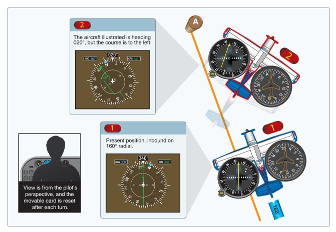
Figure 3-21. A comparison of navigation information as depicted on both analog and digital displays.
