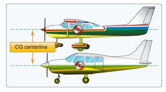
Figure 5-31. Keel area for lateral stability.
