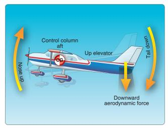
**Figure 6-10.** *The elevator is the primary control for changing the pitch attitude of an aircraft.*
