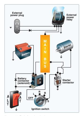
Figure 7-20. Typical starting circuit.
