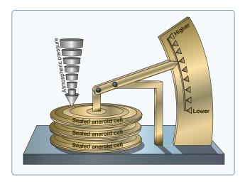
Figure 12-7. Aneroid barometer.
