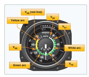
**Figure 8-8.** *Single engine airspeed indicator (ASI).*
