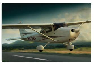
**Figure 7-37.** The landing gear supports the airplane during the takeoff run, landing, taxiing, and when parked.
