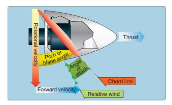
**Figure 5-44.** *Propeller blade angle.*
