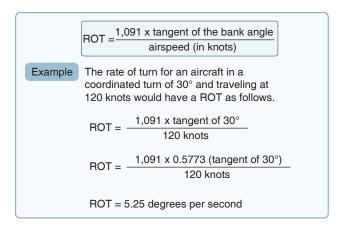
**Figure 5-56.** Rate of turn for a given airspeed (knots, TAS) and bank angle.
