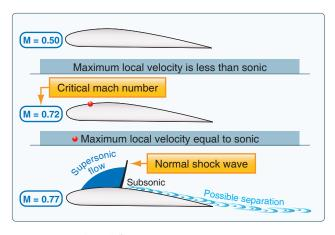
Figure 5-64. Wing airflow.
