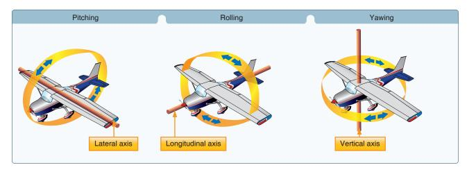
Figure 3-2. Illustrates the pitch, roll, and yaw motion of the aircraft along the lateral, longitudinal, and vertical axes, respectively.
