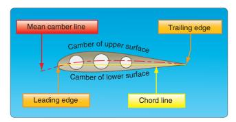
Figure 4-5. Typical airfoil section.
