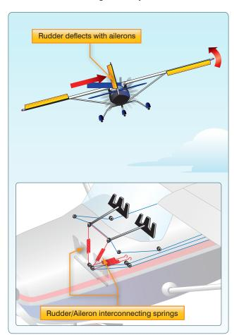
Figure 6-8. Coupled ailerons and rudder.
