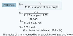
The radius of a turn required by an aircraft traveling at 240 knots using the same bank angle in Figure 4-51 is 8,861 feet. Speed is a major factor in a turn.
