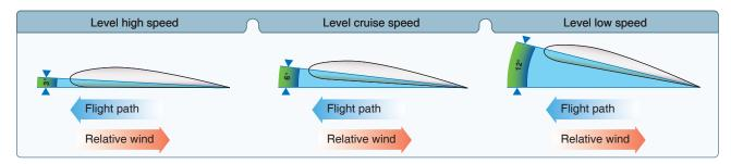
**Figure 5-3.** *Angle of attack at various speeds.*
