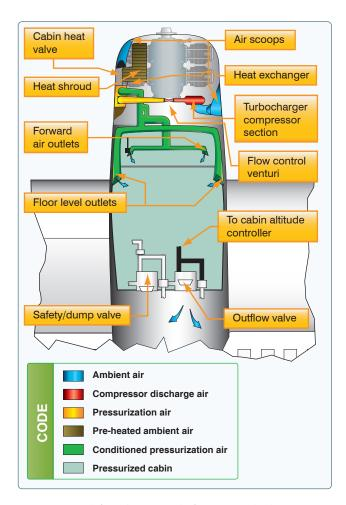
Figure 7-40. High performance airplane pressurization system.
