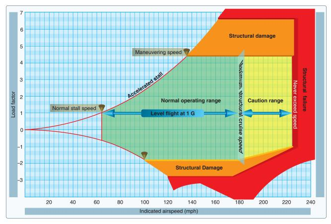
Figure 5-55. Typical Vg diagram.
