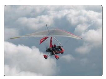
Figure 5-19. A weight-shift control aircraft.
