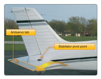
Figure 3-11. Stabilator components.
