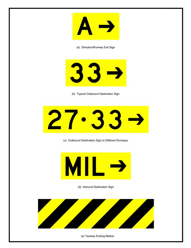
Figure 11. Examples of Direction Signs, Destination Signs, and Taxiway Ending Marker.
