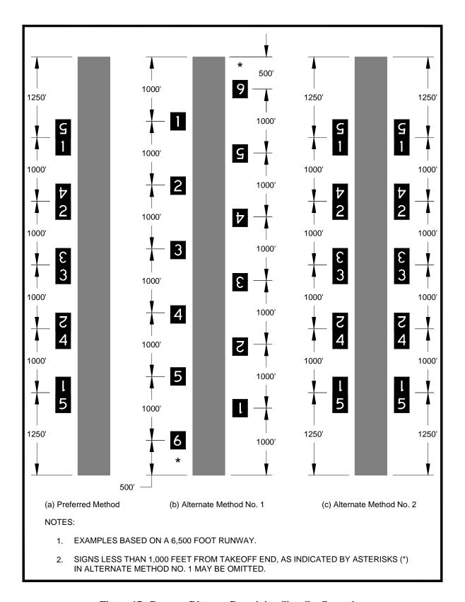
Figure 17. Runway Distance Remaining Sign Configurations.
