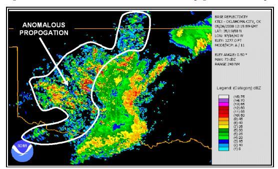
Figure 3-25. WSR-88D Weather Radar Anomalous Propagation (AP) Example
