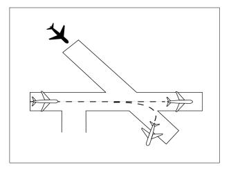
FIG 3-10-7 Intersecting Runway Separation
