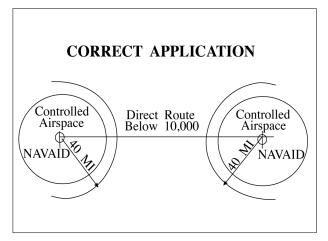
FIG 4–1–2 Application of Altitude and Distance Limitations [Application 2]
