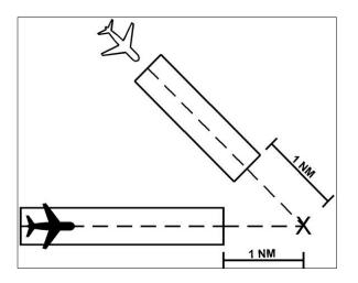
FIG 3-9-17 Intersecting Runway Separation
