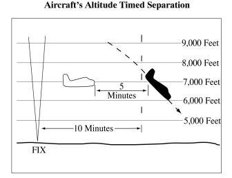
FIG 6-4-10 Climbing Through Another Aircraft's Altitude Timed Separation
