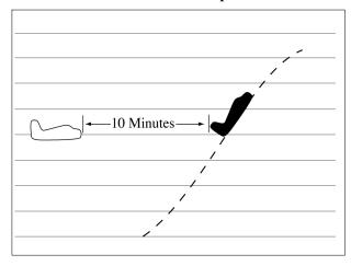
FIG 6-4-16 Descending Through Another Aircraft's Altitude Separation
