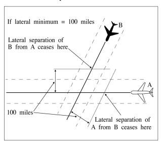
FIG 8–4–4 Separation Methods
