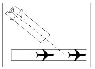
FIG 3-9-15 Intersecting Runway Separation
