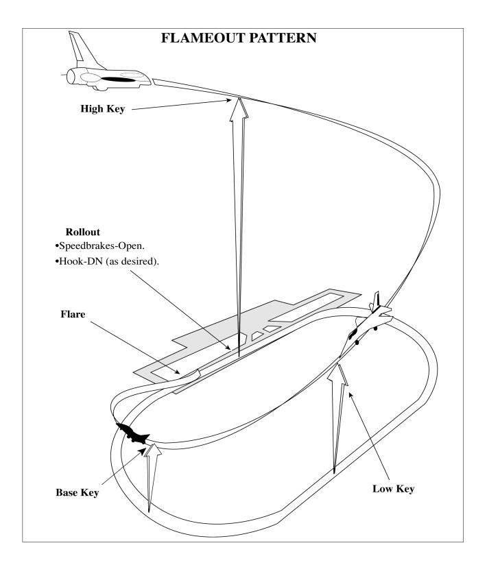
FIG 3-10-15 Simulated Flameout [2]
