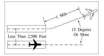
*FIG 5–8–3* Simultaneous Departures
