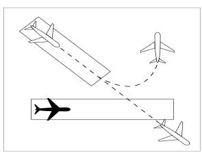
FIG 3-9-13 Intersecting Runway Separation
