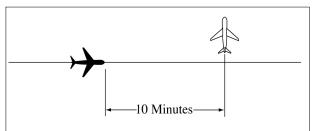
FIG 6–4–15 Climbing Through Another Aircraft's Altitude Separation
