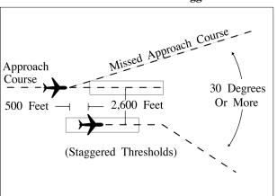
FIG 5-8-13 Parallel Thresholds are Staggered **c.** When nonintersecting runways diverge by 15 degrees or more and runway edges do not touch. (See FIG 5-8-14.)
