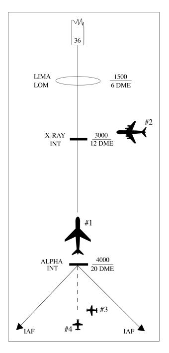
**1.** Aircraft 1 was vectored to the final approach course but clearance was withheld. It is now at 4,000 feet and established on a segment of the instrument approach procedure. "Seven miles from X-RAY. Cleared I-L-S runway three six approach." (See FIG 5–9–1.)
