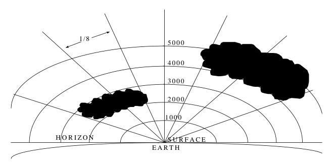
Figure 2-1. Few sky cover at 2,000 feet (2/8) and scattered sky cover at 4,000 feet (4/8). The summation of sky cover would be coded as FEW020 SCT040.
