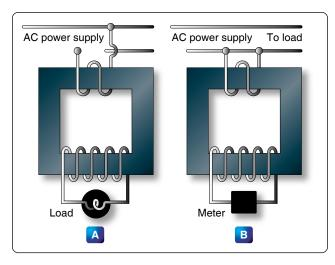
Figure 12-143. Voltage and current transformers.
