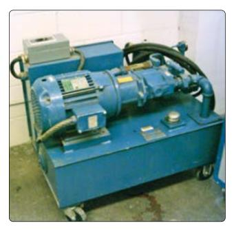
Figure 1-29. A portable hydraulic power unit.
