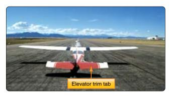
Figure 5-71. Elevator trim tab on a Cessna 182.
