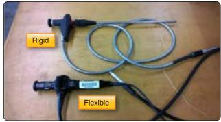
Figure 10-8. Rigid and flexible borescopes.
