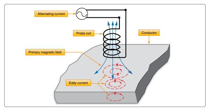
Figure 10-11. Generating an eddy current.
