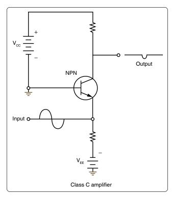
Figure 12-241. Simplified Class C amplifier circuit.
