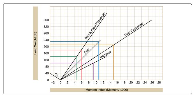
Figure 6-46. Example plots on a loading graph.
