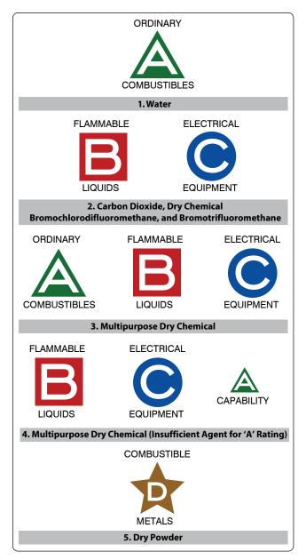
Figure 1-7. Typical extinguisher markings.
