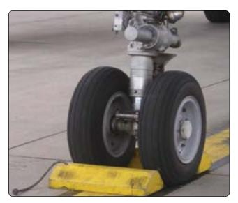
Figure 1-12. Wheels chocked fore and aft.
