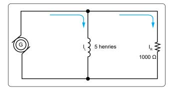
**Figure 12-138.** AC parallel circuit containing inductance and resistance.
