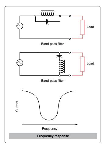
Figure 12-237. Band-stop filter.
