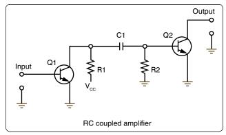
Figure 12-242. Simplified RC coupling circuit.
