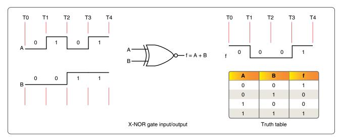
Figure 12-265. Standard Symbol for X-NOR gate.
