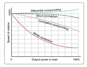
Figure 12-302. Load characteristics of DC motors.
