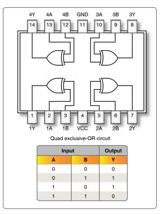
Figure 12-267. Small-scale integration schematic form.
