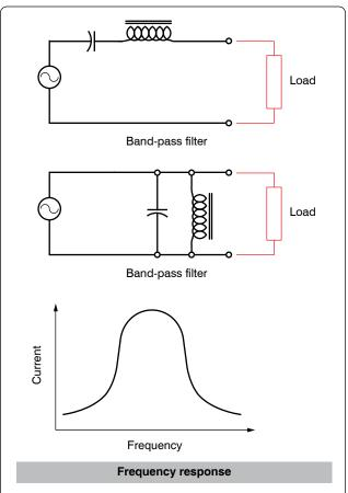
Figure 12-236. Band-pass filter.
