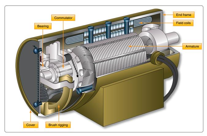
Figure 12-297. Cutaway view of practical DC motor.
