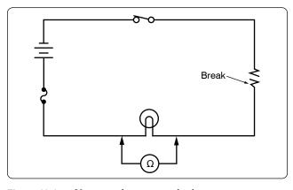
Figure 12-177. Using an ohmmeter to check a circuit component.
