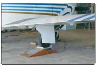
Figure 5-17. Ramp in use with a Mooney M20.
