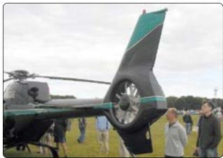
Figure 5-87. Fenestron on a Eurocopter Model 135.
