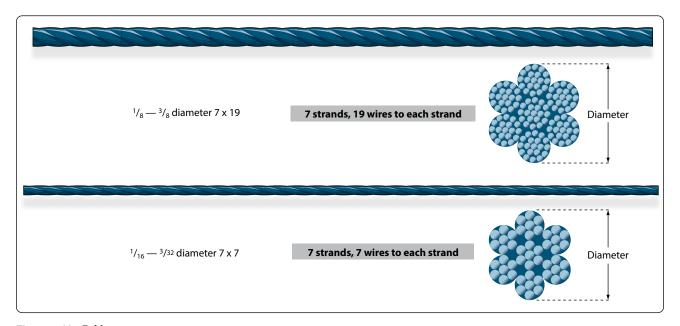
Figure 7-68. Cable cross-sections.
