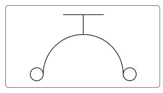
Figure 12-68. Schematic symbol for circuit breaker.
