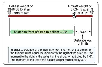
Figure 6-42. Ballast calculation as a first class lever.
