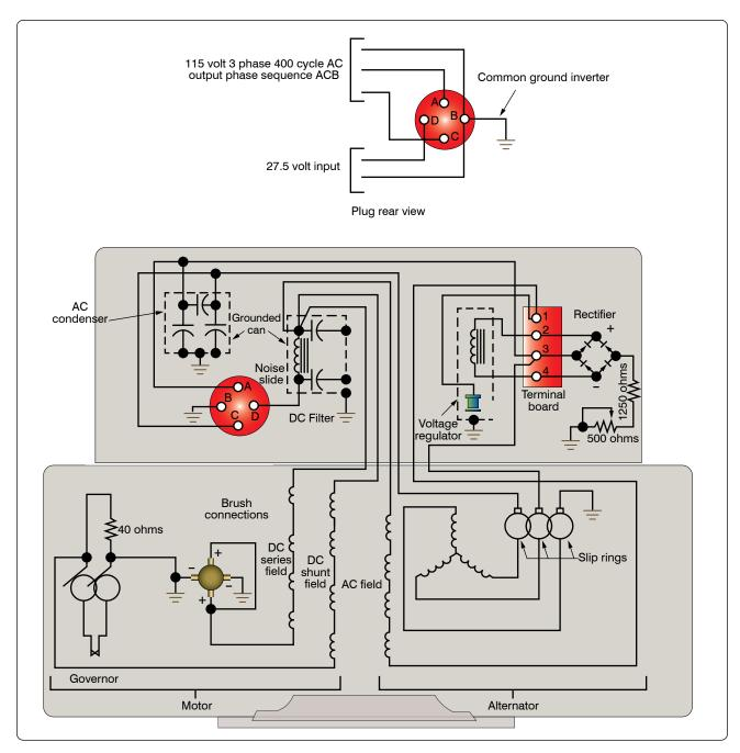
Figure 12-202. Internal wiring diagram of three-phase, revolving armature.
