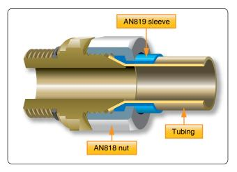
Figure 9-18. Flared tube fitting.
