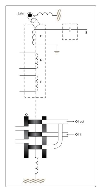
Figure 12-339. Overspeed circuit.
