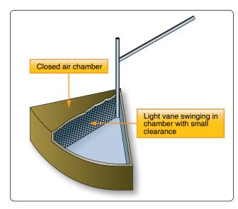
Figure 12-150. Air damping.
