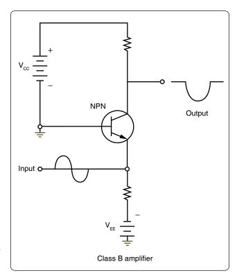
$\textbf{Figure 12-240.} \ \textit{Simplified Class B amplifier circuit.}$
