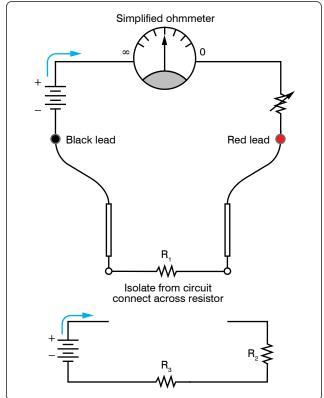
Figure 12-172. Meter adjustment.
