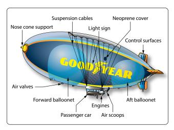
Figure 5-40. The Goodyear Airship and buoyancy.
