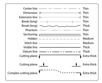
Figure 4-24. The meaning of lines.
