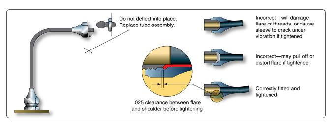
Figure 9-28. Correct and incorrect methods of tightening flared fittings.
