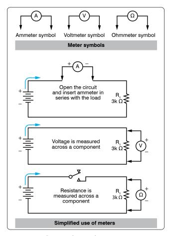
Figure 12-170. Current, voltage, and resistance measurement.
