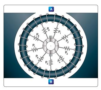
Figure 12-316. Preventive coils in AC series motor.
