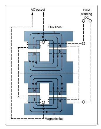
Figure 12-203. Diagram of basic inductor-type inverter.
