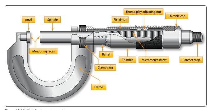
Figure 11-36. Outside micrometer parts.
