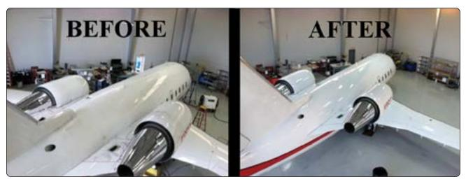
Figure 8-31. Protective paint finishes are the most effective means of preventing corrosion.
