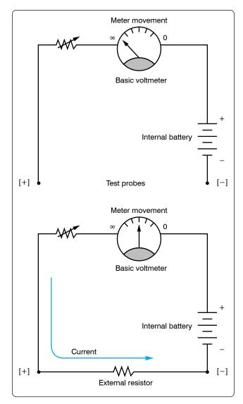
Figure 12-154. Basic ohmmeter.
