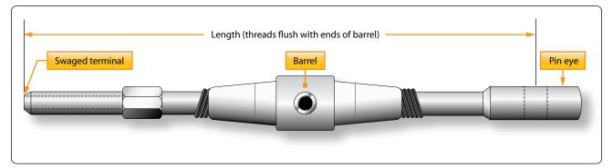
Figure 7-70. Typical turnbuckle assembly.
