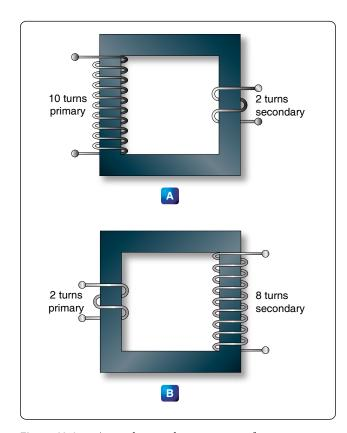
Figure 12-144. A step-down and a step-up transformer.
