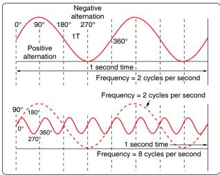
Figure 12-111. Frequency in cycles per second.
