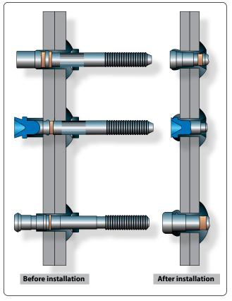
Figure 7-43. Self-plugging (mechanical lock) rivets.
