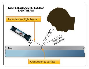
Figure 10-7. Using a flashlight to inspect for cracks.
