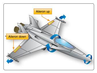
Figure 5-69. Aircraft performing an aileron roll.
