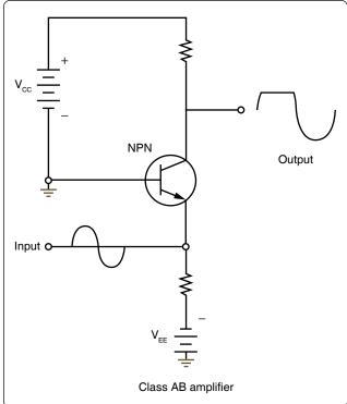
Figure 12-239. Simplified Class AB amplifier circuit.
