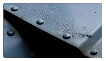
Figure 8-8. Filiform corrosion.
