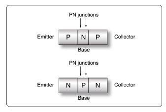
Figure 12-220. Transistor.
