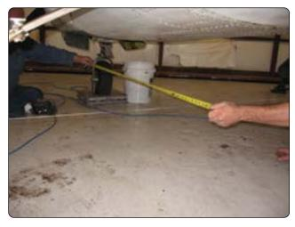
Figure 6-23. Measuring the nosewheel arm on an airplane.
