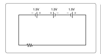
Figure 12-85. Voltage sources add algebraically; one source reversed.
