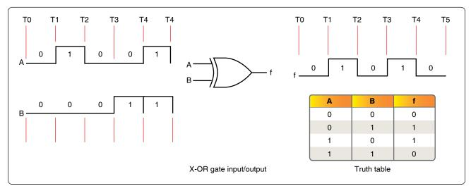
Figure 12-264. Standard symbol and truth table for X-OR gate.
