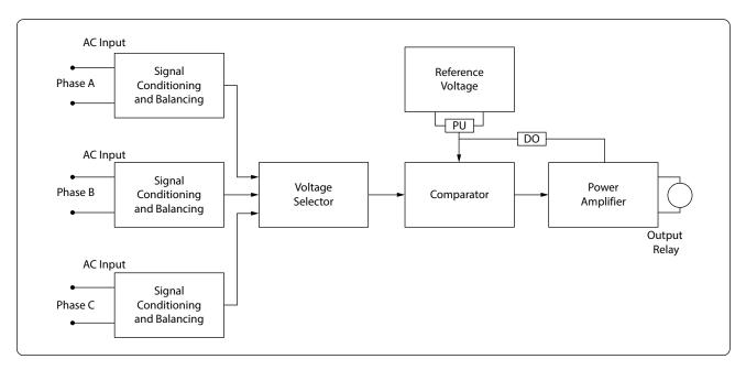
Figure 4-20. Block diagram.
