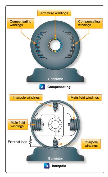
Figure 12-284. Simple two-pole generator with two interpoles.
