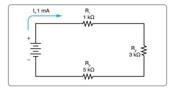
Figure 12-83. Example of three resistors in series.
