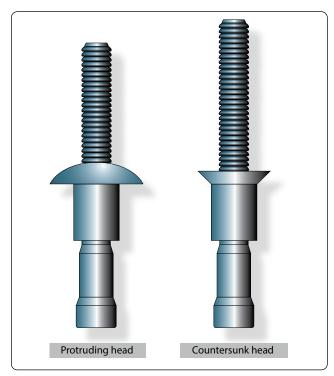
Figure 7-39. Self-plugging (friction lock) rivets.
