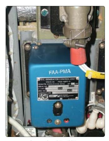
Figure 12-332. Generator Control Unit (GCU).
