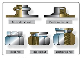
Figure 7-26. Self-locking nuts.
