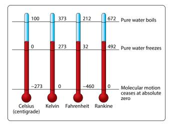
Figure 5-31. Comparison of temperature scales.
