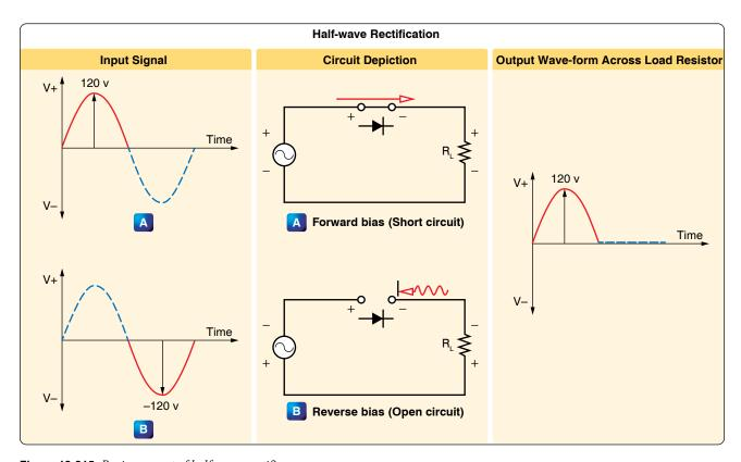
Figure 12-215. Basic concept of half-wave rectifier.
