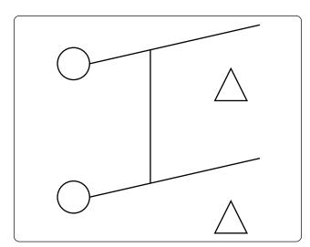
Figure 12-73. Double-pole, single-throw switch schematic symbol.
