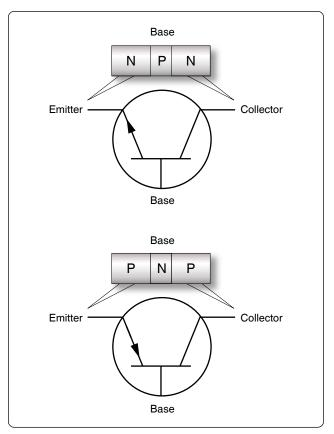
Figure 12-221. Two basic transistors with circuit symbols.
