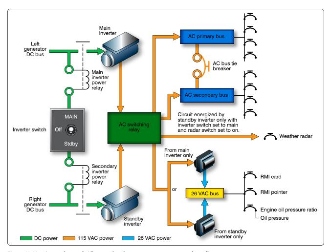
$\textbf{Figure 12-205.} \ \textit{A typical aircraft AC power distribution system using main and standby rotary inverters.} \\$
