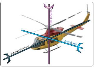
Figure 5-90. Three axes of rotation for a helicopter.
