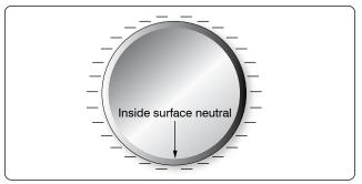
Figure 12-12. Charge on a hollow sphere.
