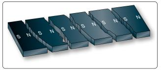
Figure 12-22. Magnetic poles in a broken magnet.
