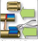
Locate length of hose to be cut off and slit cover with knife to wire braid, taking care to not damage underlying materials. After slitting cover, twist off with pair of pliers. (See note below.)
