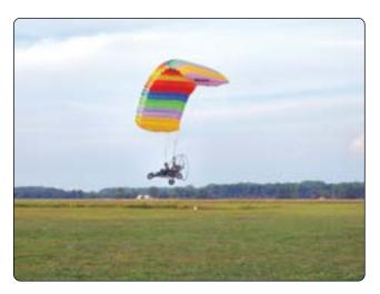
Figure 5-102. Powered parachute with the wing inflated.
