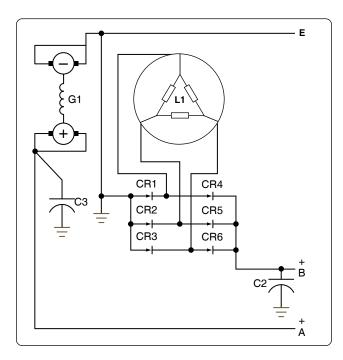
Figure 12-323. Wiring diagram of alternator-rectifier unit.
