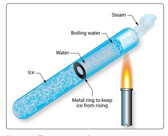
**Figure 5-28.** *Water as a poor conductor.*
