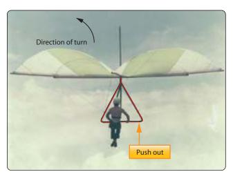
Figure 5-99. Direction of turn based on weight shift.
