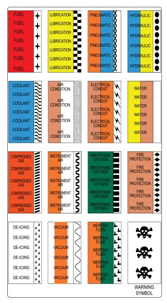
Figure 9-16. *Identification of aircraft fluid lines*.
