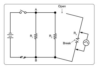
**Figure 12-185.** Opening a branch circuit to obtain an accurate ohmmeter reading.
