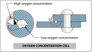
Figure 8-12. Oxygen concentration cell.
