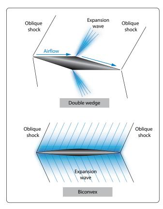
Figure 5-80. Double wedge and biconvex supersonic wing design.
