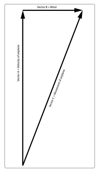
Figure 5-25. Vector analysis for airplane velocity and wind velocity.
