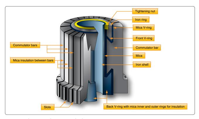
Figure 12-282. Commutator with portion removed to show construction.
