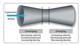
Figure 5-74. Supersonic airflow through a venturi.
