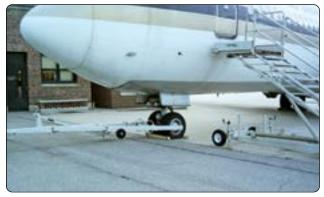
Figure 1-20. Example of a tow bar.
