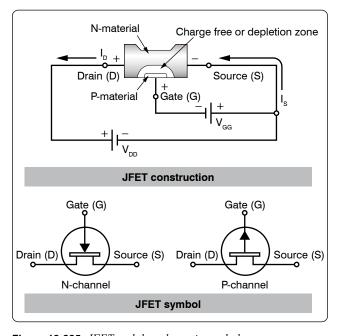
Figure 12-225. JFET and the schematic symbol.
