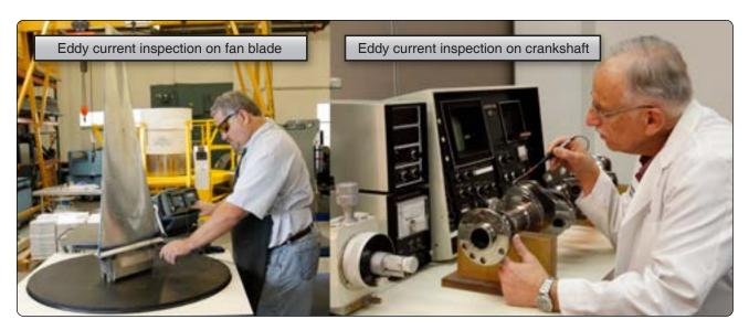
Figure 10-10. Eddy current inspection.
