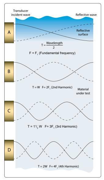
Figure 10-23. Conditions of ultrasonic resonance in a metal plate.
