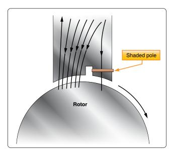
Figure 12-310. Diagram of a shaded pole motor.
