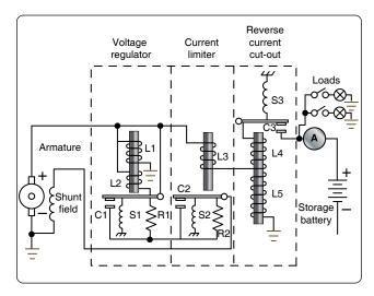
**Figure 12-330.** *Three unit regulator for variable speed generators.*
