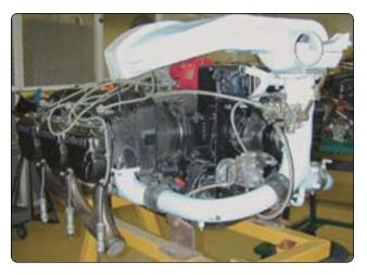
Figure 5-29. Aircraft piston engine cooled by convection.
