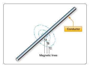
Figure 12-27. Expansion of magnetic field as current increases.
