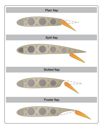
**Figure 5-73.** *Four types of wing flaps.*
