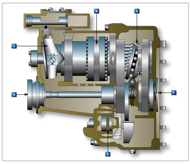
Figure 12-334. Cutaway of a hydraulic transmission.
