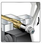
Screw nipple into socket using wrench on hex of nipple and leave .005" to .031" clearance between nipple hex and socket.
