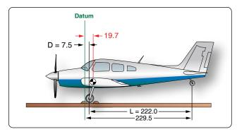
**Figure 6-31.** The datum of this tail wheel airplane is the wing root leading edge.
