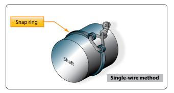
Figure 7-78. External type snap ring with safety wire installation.
