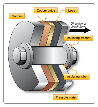
Figure 12-217. Copper oxide dry disk rectifier.
