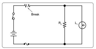
Figure 12-187. An open in the series portion of a series-parallel circuit.
