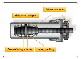
Figure 7-17. V-ring installation.
