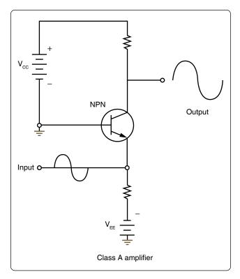
Figure 12-238. Simplified Class A amplifier circuit.
