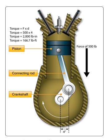
Figure 5-6. Piston engine and torque.
