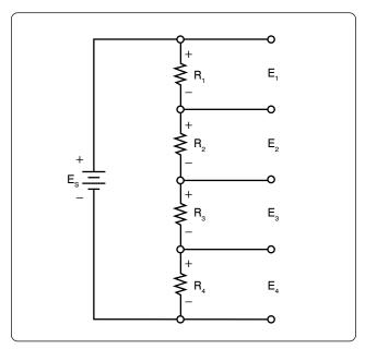
Figure 12-94. Four resistor voltage divider.
