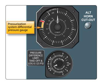
Figure 5-36. Differential pressure gauge.
