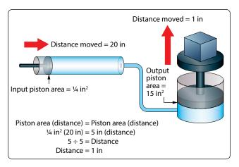
Figure 5-45. Piston movement in a hydraulic system.
