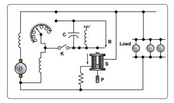
**Figure 12-328.** *Vibrating-type voltage regulator.*
