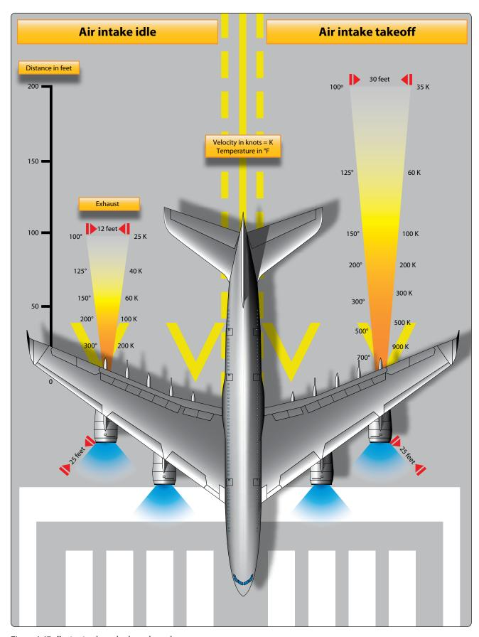
Figure 1-17. Engine intake and exhaust hazard areas.
