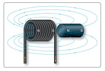
Figure 12-36. Solenoid with iron core.
