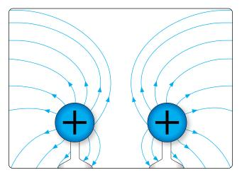
Figure 12-10. Field around two positively-charged bodies.
