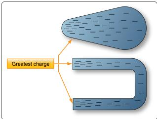
Figure 12-13. Charge on irregularly-shaped objects.
