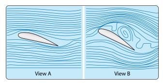
Figure 5-58. Wing boundary layer separation.
