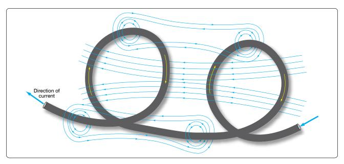
Figure 12-32. Magnetic field around a conductor with two loops.
