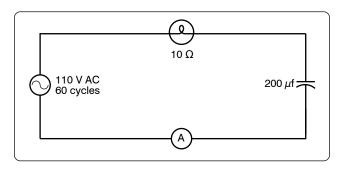
Figure 12-136. A circuit containing resistance and capacitance.
