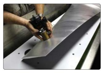
**Figure 10-25.** *Ultrasonic inspection of a composite structure.*
