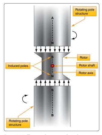
Figure 12-312. Illustrating the operation of a synchronous motor.
