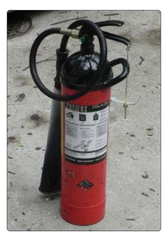
Figure 1-4. Carbon dioxide fire extinguisher.
