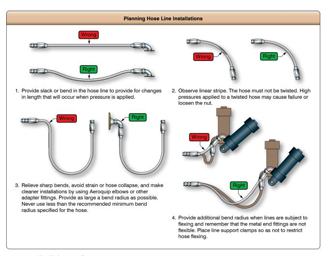
Figure 9-40. Flexible hose installation.
