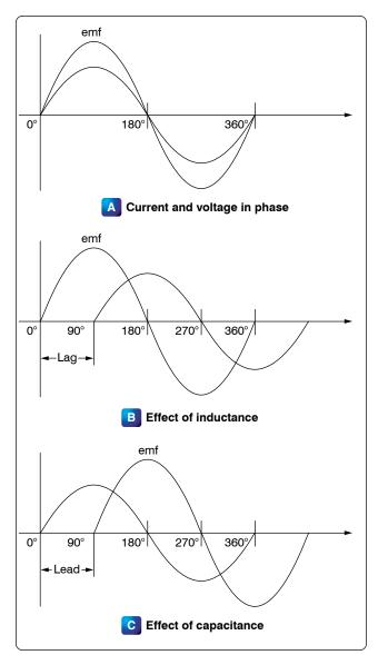
Figure 12-124. Phase of current and voltage.
