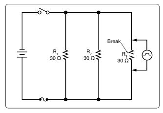
Figure 12-184. A misleading ohmmeter indication.
