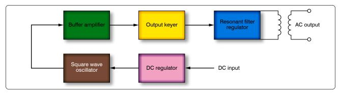
Figure 12-207. Regulated sine wave static inverter.
