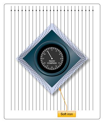
Figure 12-23. Magnetic shield.
