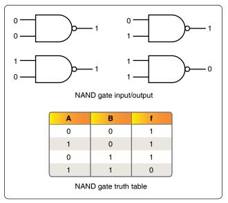
Figure 12-261. Two input NAND gate and corresponding truth table.
