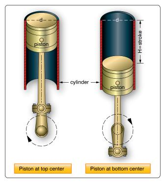
Figure 3-27. Cylinder displacement.
