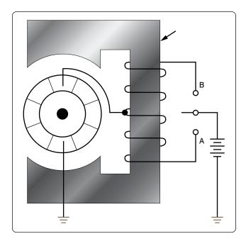
Figure 12-303. Split field series motor.
