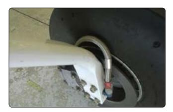
Figure 9-32. Flexible hose with stainless braid.
