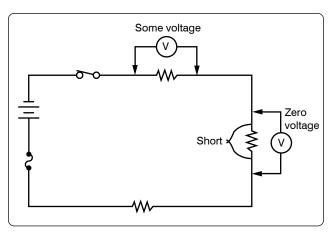
Figure 12-182. Voltmeter connected across resistors.
