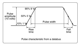
Figure 12-252. Non-ideal pulse and its characteristics.
