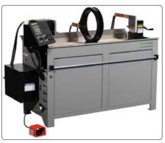
Figure 10-33. Fixed general-purpose magnetizing unit.
