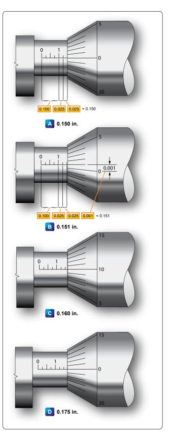
**Figure 11-38.** *Reading a micrometer.*
