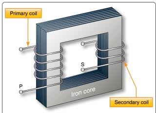
Figure 12-142. An iron-core transformer.
