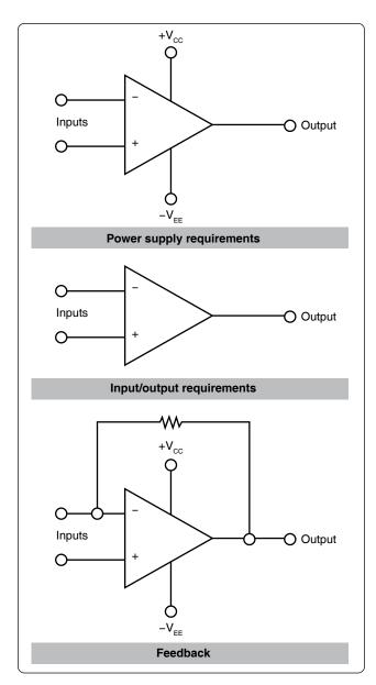
**Figure 12-246.** *Schematic symbol for the operational amplifier.*
