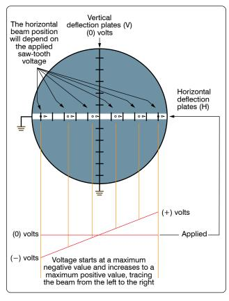
Figure 12-166. Saw-tooth applied voltage.
