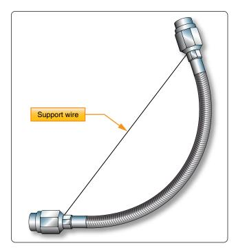
Figure 9-34. Suggested handling of preformed hose.
