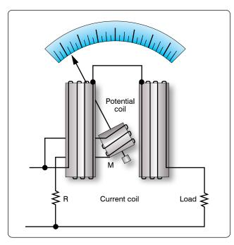
Figure 12-163. Simplified electrodynamometer wattmeter circuit.
