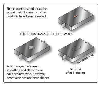
Figure 8-24. Blend of corrosion as a single depression.
