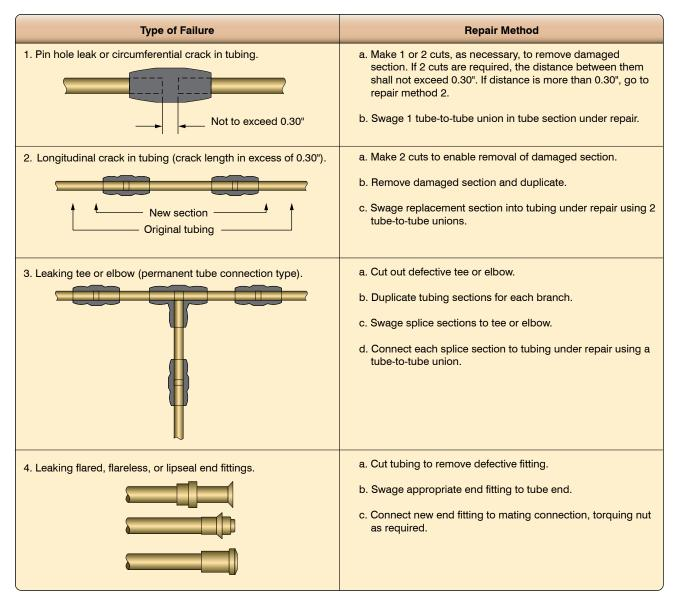
Figure 9-30. *Permaswage* TM repair.
