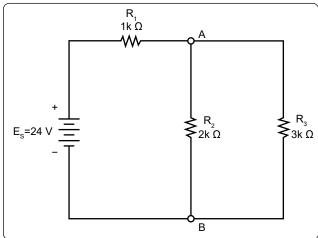
Figure 12-102. Determining total resistance.
