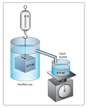
Figure 5-38. Example of buoyancy.
