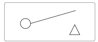
Figure 12-71. Single-pole, single-throw switch schematic symbol.
