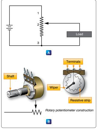
Figure 12-61. Potentiometer and schematic symbol.
