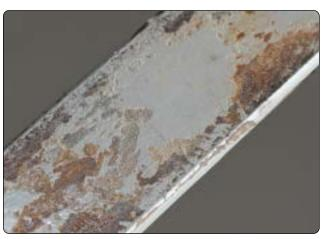
Figure 8-17. Fretting corrosion.
