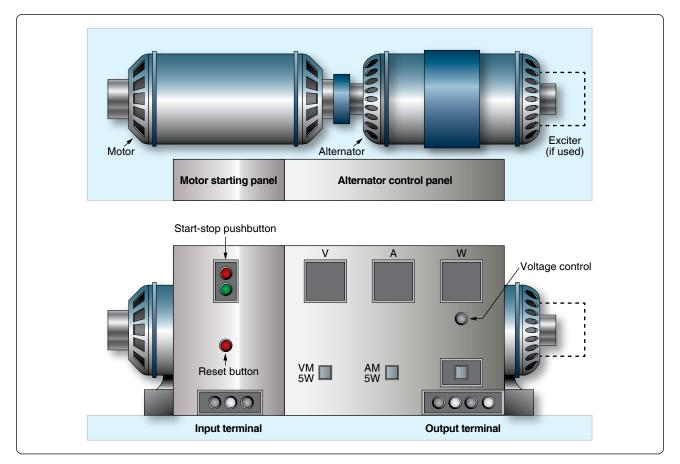
**Figure 12-326.** AC motor generator set for ground testing.
