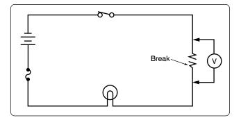
Figure 12-176. Voltmeter across a resistor in an open circuit.
