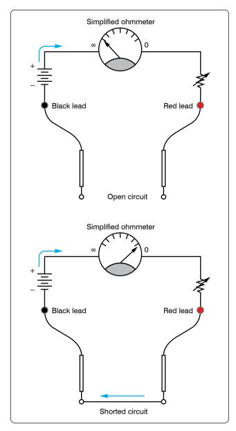
Figure 12-171. Meter configurations during adjustments.
