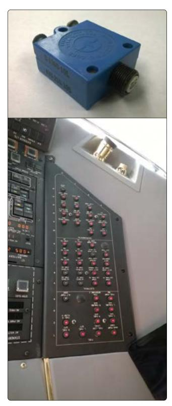
Figure 12-69. Circuit breaker assembly for aircraft electrical system.
