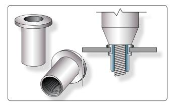
Figure 7-64. Internally-threaded rivet (Rivnut).
