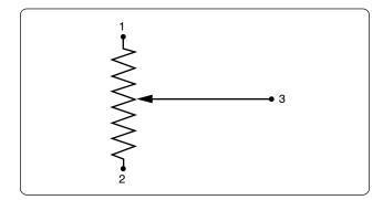
Figure 12-60. Potentiometer schematic symbol.
