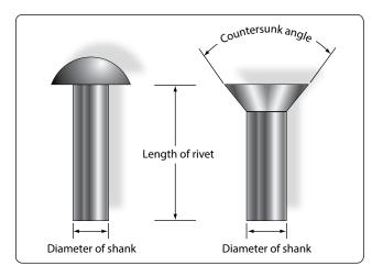
Figure 7-38. Methods of measuring rivets.
