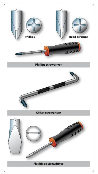
Figure 11-2. Typical screwdrivers.
