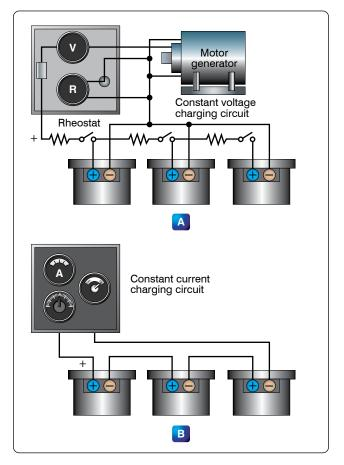
Figure 12-196. Battery charging methods.
