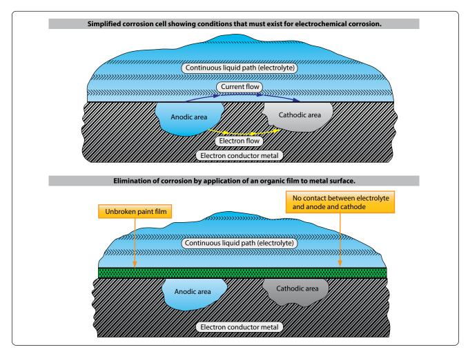
Figure 8-5. Electrochemical attack.
