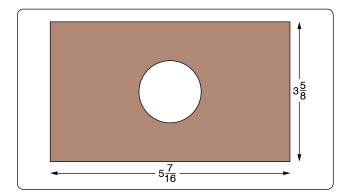
Figure 3-2. Center hole of the plate.
