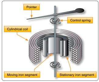
Figure 12-161. Moving iron vane meter.
