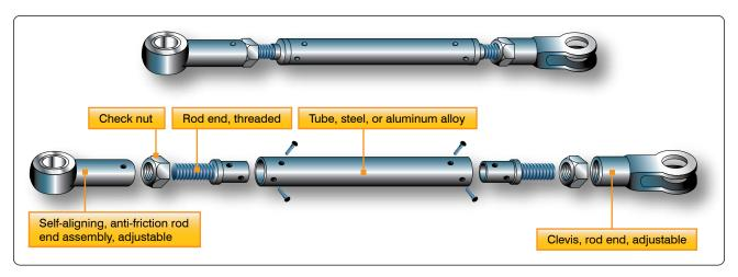
Figure 7-71. Push-pull tube assembly.
