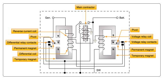
Figure 12-331. Differential generator control relay.
