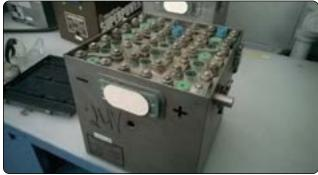
Figure 12-198. Nickel-Cadmium aircraft battery.
