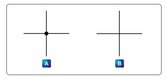
Figure 12-46. Connected wires.
