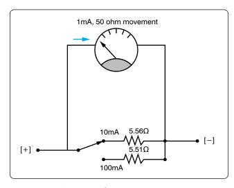
Figure 12-151. Ammeter with two ranges.
