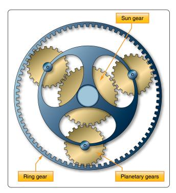
Figure 5-16. Planetary sun gear.
