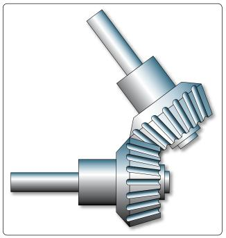
Figure 5-14. Bevel gears.
