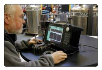
Figure 10-17. Ultrasonic inspection.
