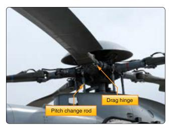
Figure 5-83. Eurocopter 725 main rotor head.
