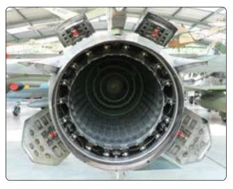
Figure 8-19. Exhaust nozzle area.
