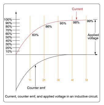
Figure 12-126. Inductor curve.
