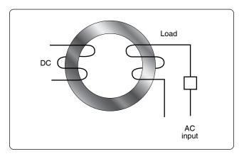
Figure 12-248. Saturable CORE reactor circuit.
