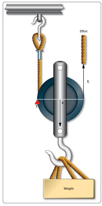
Figure 5-11. Single movable pulley.
