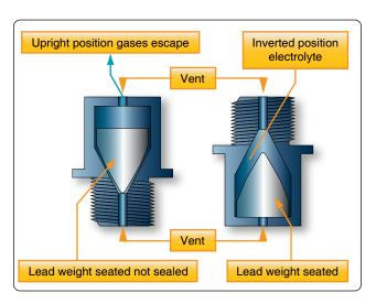
Figure 12-192. Nonspill battery vent plug.
