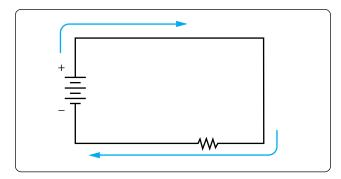
Figure 12-81. Simple DC circuit.
