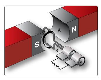
**Figure 12-270.** *Inducing minimum voltage in an elementary generator.*
