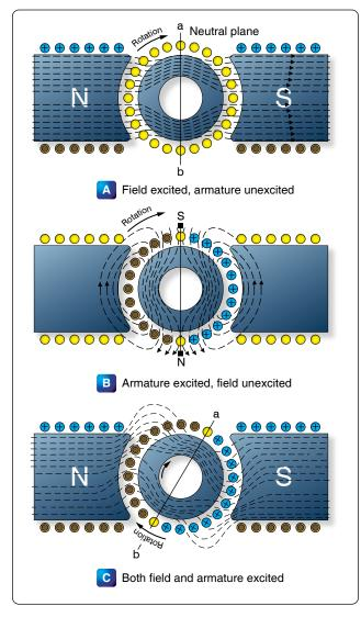
Figure 12-283. Armature reaction.
