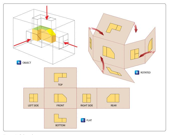
Figure 4-11. Orthographic projection.
