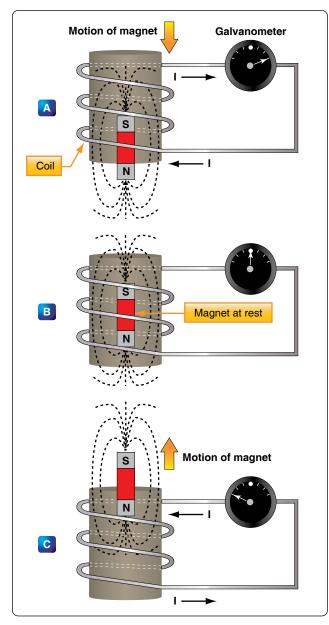
Figure 12-104. Inducing a current flow.
