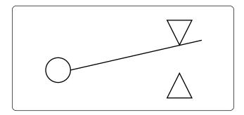
Figure 12-72. Single-pole, double-throw switch schematic symbol.
