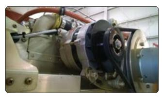
Figure 12-317. Belt driven alternator for small single-engine aircraft.
