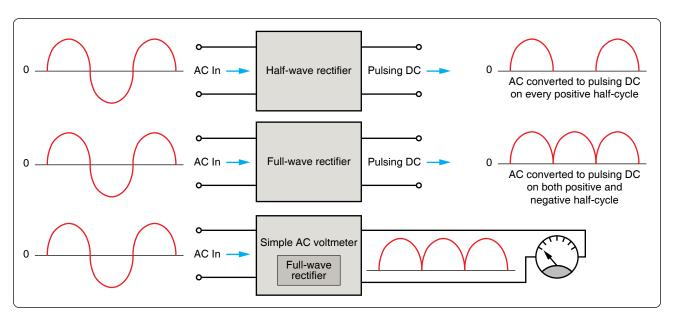
Figure 12-159. Simplified block diagram of AC meter.
