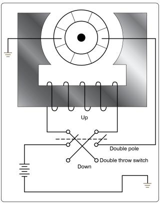
Figure 12-304. Switch method of reversing motor direction.
