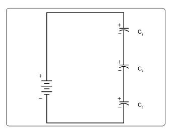
Figure 12-121. Simple series circuit.
