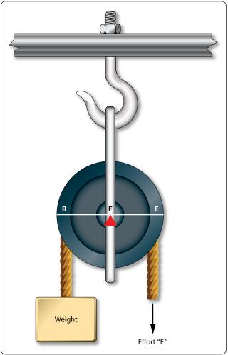
Figure 5-10. Single fixed pulley.
