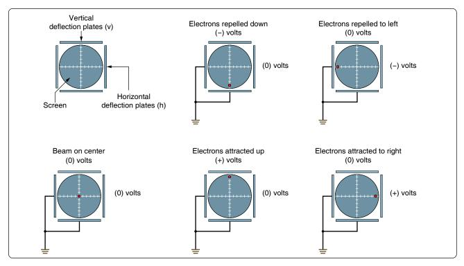
Figure 12-165. Possible plate voltage combinations and the resultant beam position.
