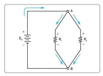
Figure 12-96. Basic parallel circuit.
