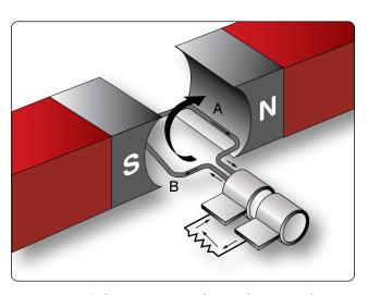
**Figure 12-271.** *Inducing maximum voltage in the opposite direction.*
