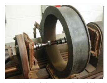
**Figure 10-30.** Longitudinal magnetization of camshaft (solenoid method).
