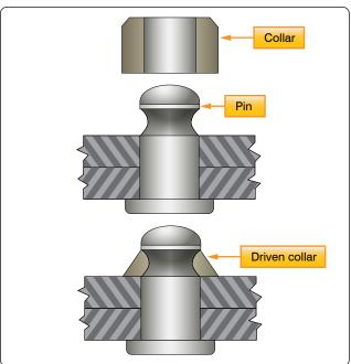
Figure 7-55. Pin (Hi-Shear) rivet.
