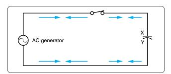
Figure 12-123. Capacitor in an AC circuit.
