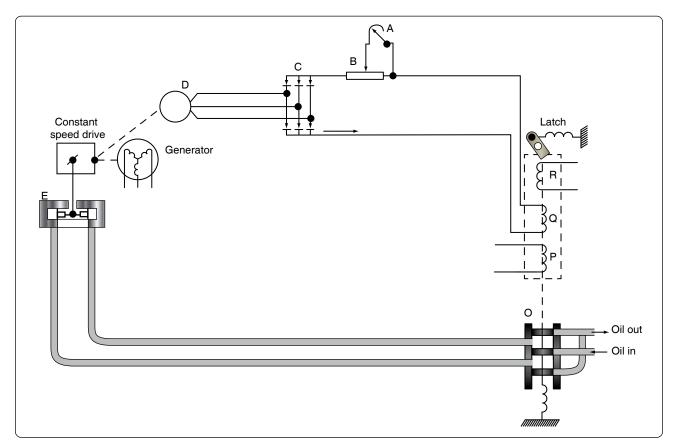
Figure 12-337. Electrical hydraulic control circuit.
