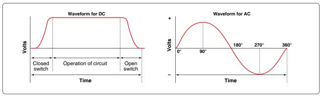
Figure 12-103. DC and AC voltage curves.
