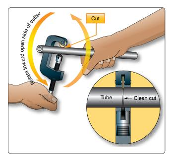
Figure 9-2. Tube cutting.
