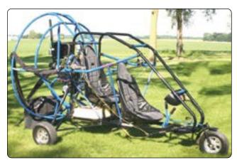
**Figure 5-103.** *Two seat powered parachute.*
