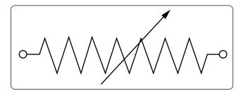
Figure 12-58. Rheostat schematic symbol.
