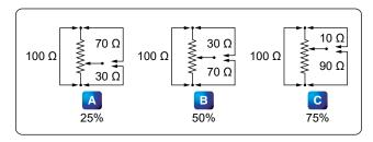
Figure 12-63. *Linear potentiometer schematic.*
