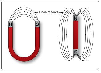
Figure 12-15. Magnetic field around magnets.
