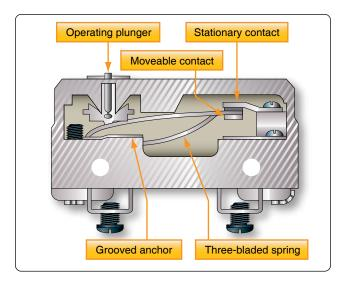
Figure 12-75. Cross-section of a microswitch.
