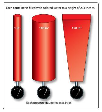
Figure 5-41. Fluid pressure based on column height.
