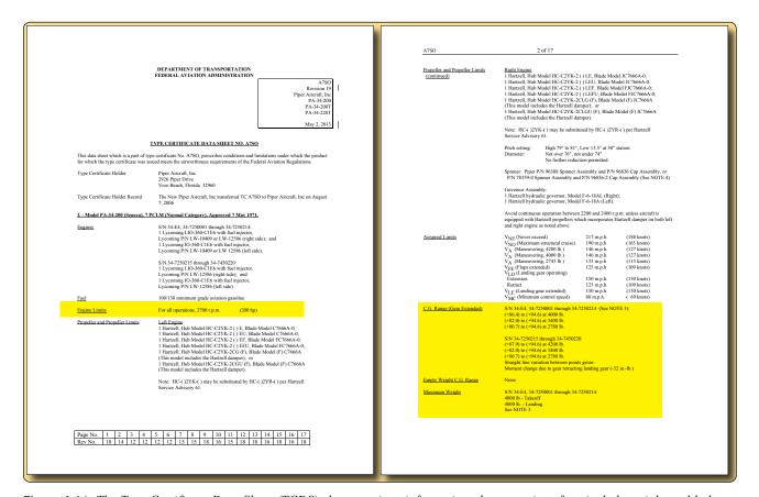
**Figure 6-14.** The Type Certificate Data Sheet (TCDS) shows various information about an aircraft to include weight and balance information.
