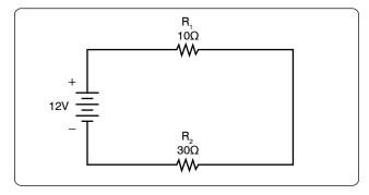
Figure 12-82. Simple DC circuit with additional resistor.
