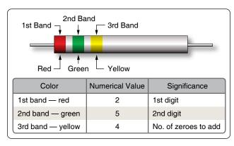
Figure 12-50. End-to-center band marking.
