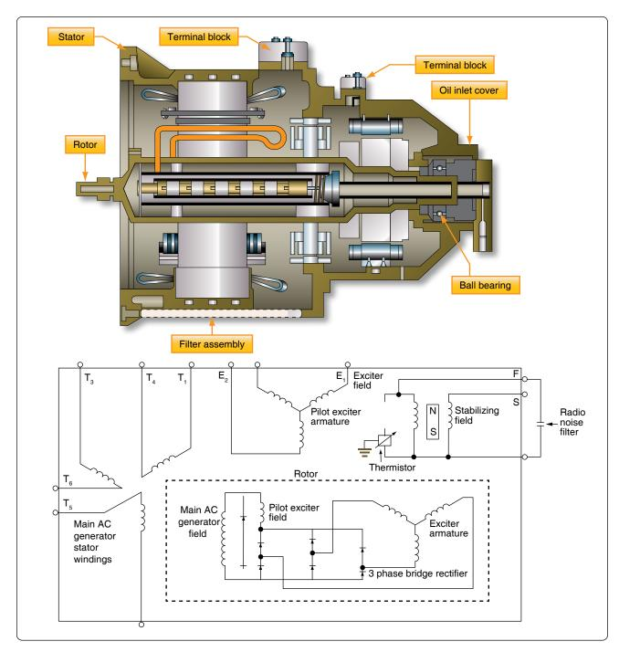
Figure 12-324. A typical brushless alternator.
