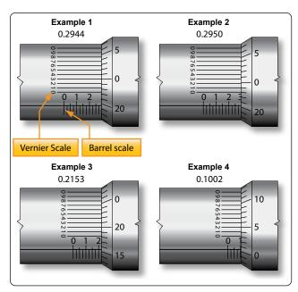
Figure 11-39. Vernier scale readings.
