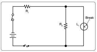
Figure 12-189. An open lamp in a series-parallel circuit.
