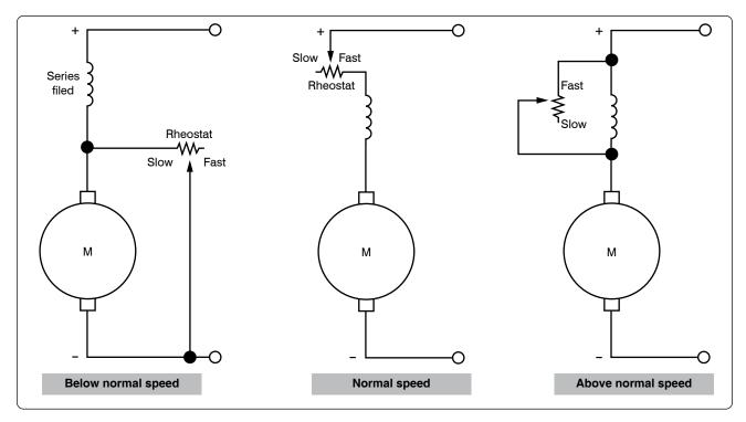
**Figure 12-306.** *Controlling the speed of a series DC motor.*
