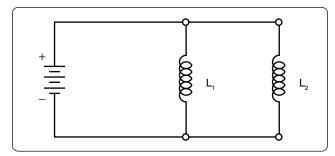
Figure 12-129. Two inductors in parallel.
