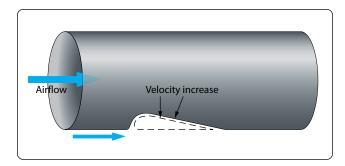
**Figure 5-56.** *Venturi with a superimposed wing.*
