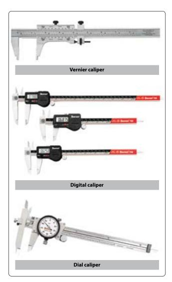
$\textbf{Figure 11-41.} \ Electronic \ and \ dial \ indicator \ slide \ calipers.$
