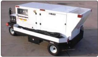
Figure 1-27. A mobile electrical power unit.
