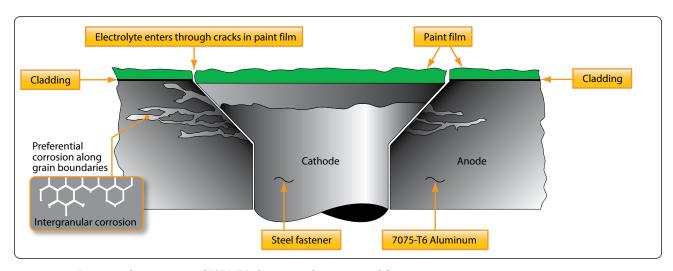
**Figure 8-14.** *Intergranular corrosion of 7075-T6 aluminum adjacent to steel fastener.*
