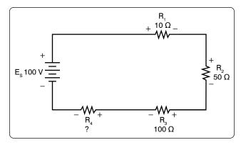
Figure 12-88. Determine the unknown voltage drop.
