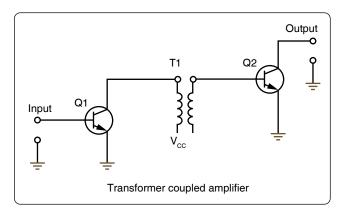
Figure 12-244. Simplified transformer coupling circuit.
