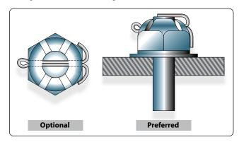
Figure 7-77. Cotter pin installation.
