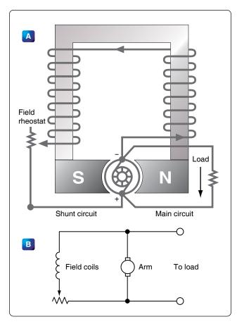
Figure 12-286. Shunt wound generator.
