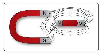
Figure 12-20. Bypassing flux lines.
