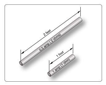
Figure 12-41. Resistance varies with length of conductor.
