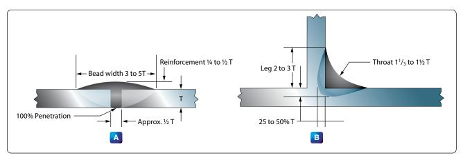
Figure 10-39. Butt weld (A) and fillet weld (B), showing width and depth of bead.
