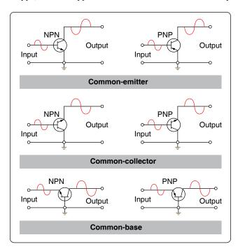
Figure 12-227. Transistor configurations (common-emitter, common-collector, common-base).
