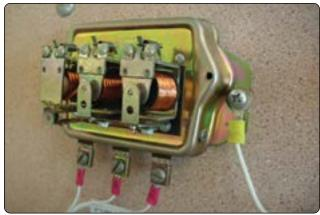
Figure 12-329. Three unit regulator.
