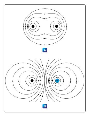
Figure 12-292. Fields surrounding parallel conductors.
