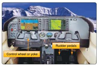
Figure 5-68. Cessna 182 control wheel and rudder pedals.
