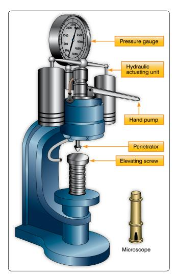
Figure 7-9. Brinell hardness tester.
