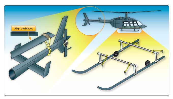
Figure 1-14. Securing helicopter blades and fuselage.
