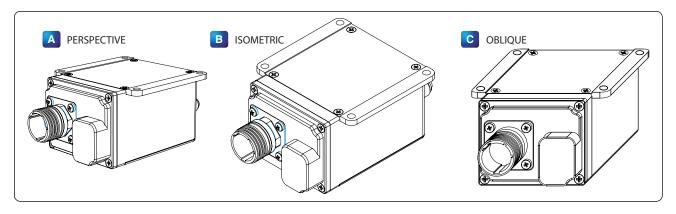
**Figure 4-16.** (A) Perspective, (B) isometric, and (C) oblique drawings.
