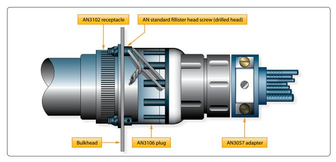
Figure 7-74. Safety wiring attachment for plug connectors.
