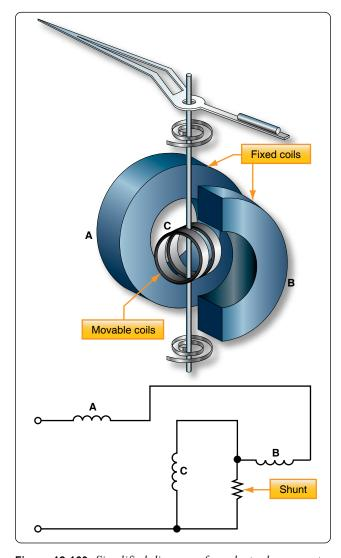
**Figure 12-160.** Simplified diagram of an electrodynamometer movement.
