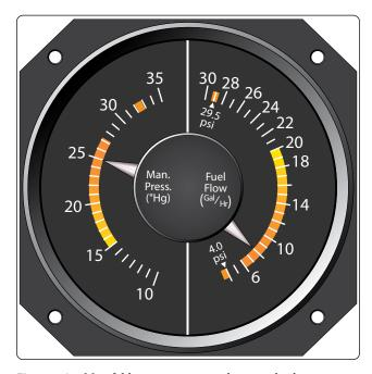
Figure 5-35. Manifold pressure gauge indicating absolute pressure.
