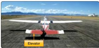
Figure 5-65. Elevator on a Cessna 182 provides pitch control.
