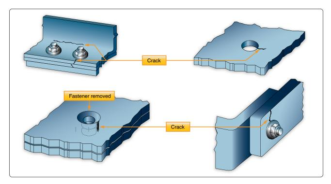
Figure 10-14. Typical surface cracks.
