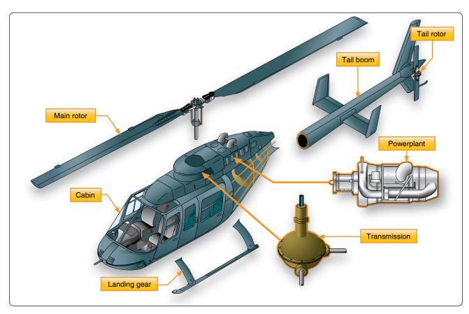
Figure 5-81. Main components of a helicopter.
