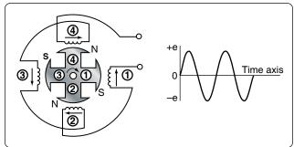
Figure 12-319. Single-phase alternator.
