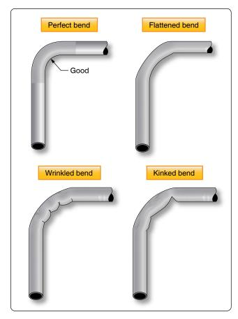
Figure 9-8. Correct and incorrect tubing bends.
