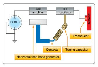
Figure 10-24. Block diagram of resonance thickness measuring system.
