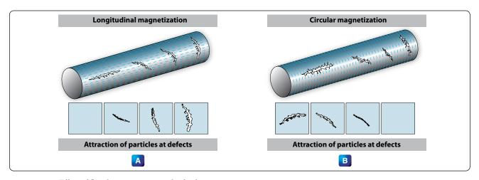
Figure 10-28. Effect of flux direction on strength of indication.
