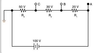
Figure 12-93. Voltage divider with changed ground.
