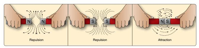
**Figure 12-21.** *Repulsion and attraction of magnet poles.*
