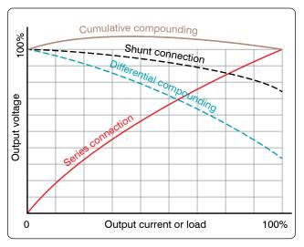
Figure 12-288. Generator characteristics.
