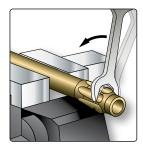
3. Place hose in vise and screw socket on hose counterclockwise.
