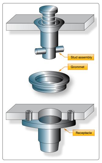
Figure 7-60. Camloc fastener.
