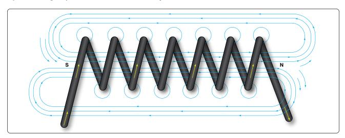
Figure 12-33. Magnetic field of a coil.
