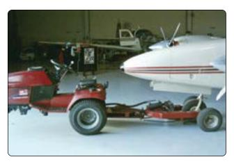
Figure 1-21. Typical smaller aircraft tow tractor.
