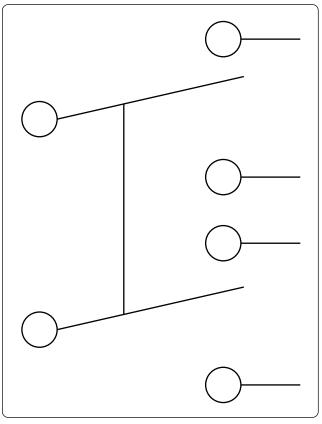
Figure 12-74. Double-pole, double-throw switch schematic symbol.
