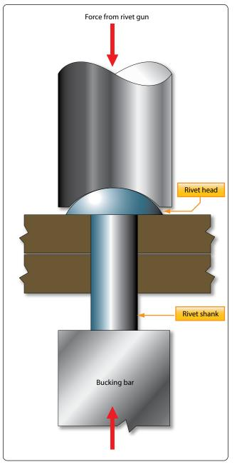
**Figure 5-19.** A rivet fastener and compression.
