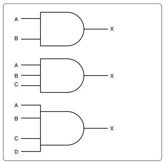
Figure 12-255. AND gate logic symbol.
