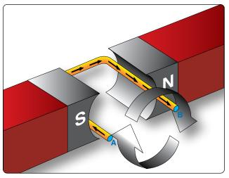
Figure 12-107. Voltage induced in a loop.
