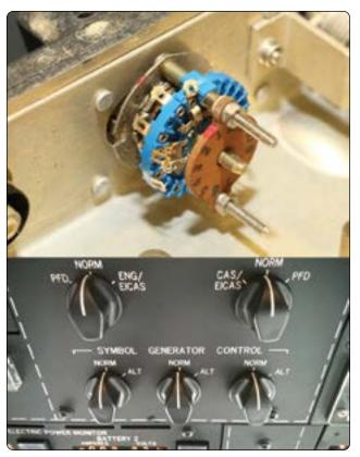
Figure 12-77. Rotary switches.
