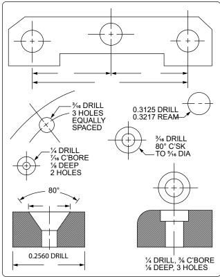
Figure 4-26. Dimensioning holes.
