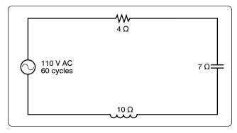
**Figure 12-137.** A circuit containing resistance, inductance, and capacitance.
