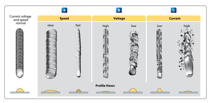
**Figure 10-38.** Examples of poor welds: too rapidly (A), improper penetration and cold laps (B), and irregular edges and considerable variation (C).
