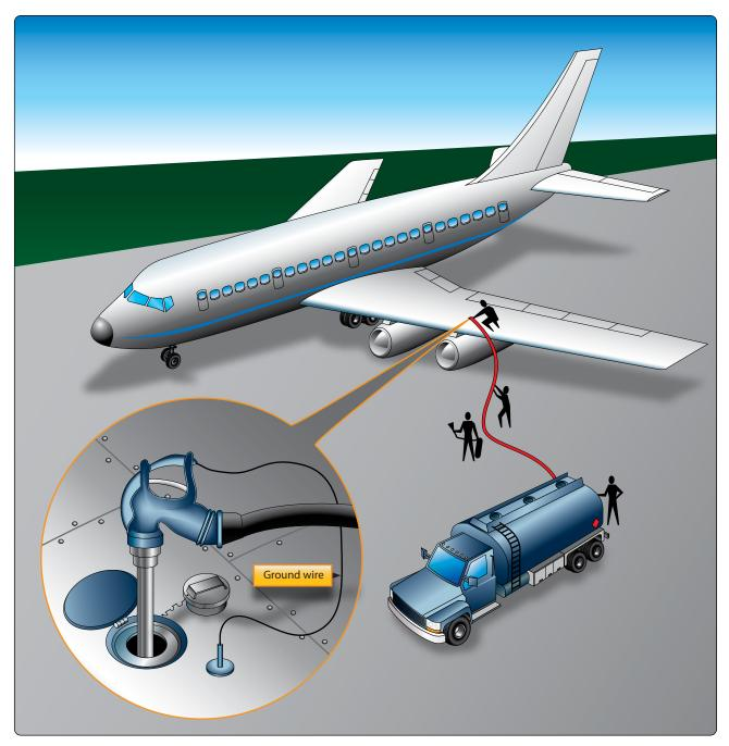
**Figure 1-32.** *Refueling an aircraft by the over-the-wing method.*
