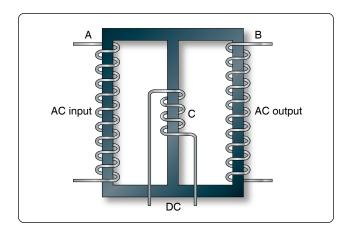
Figure 12-247. Magnetic amplifier circuit.
