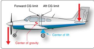
Figure 5-62. Longitudinal stability and balance.
