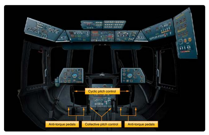
Figure 5-91. Helicopter cockpit controls.
