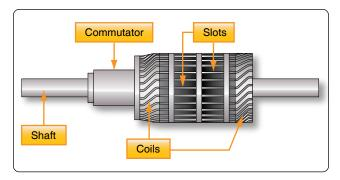
Figure 12-281. A drum-type armature.
