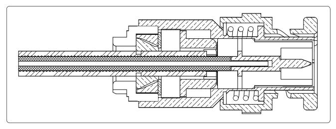
**Figure 4-6.** *Sectional view of a cable connector.*
