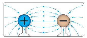
**Figure 12-9.** Direction of electric field around positive and negative charges.
