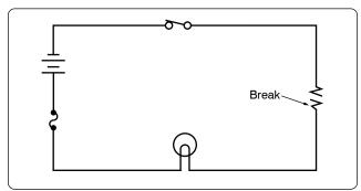
Figure 12-174. An open circuit.
