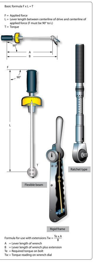
Figure 7-33. Common torque wrenches.
