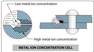
Figure 8-11. Metal ion concentration cell.
