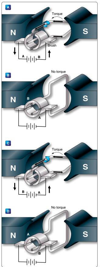
Figure 12-296. Basic DC motor operation.
