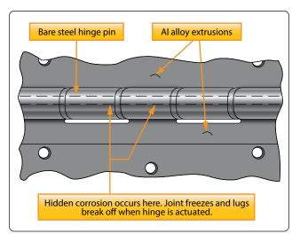
Figure 8-22. Hinge corrosion points.
