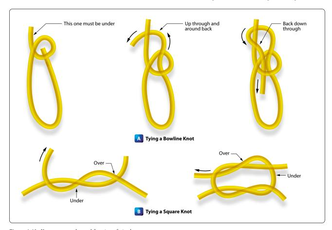
**Figure 1-10.** *Knots commonly used for aircraft tie-down.*
