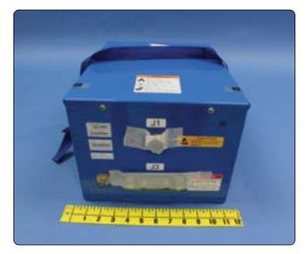
Figure 12-200. Boeing 787 lithium-ion battery.
