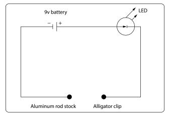
Figure 7-2. Wiring assembly schematic.
