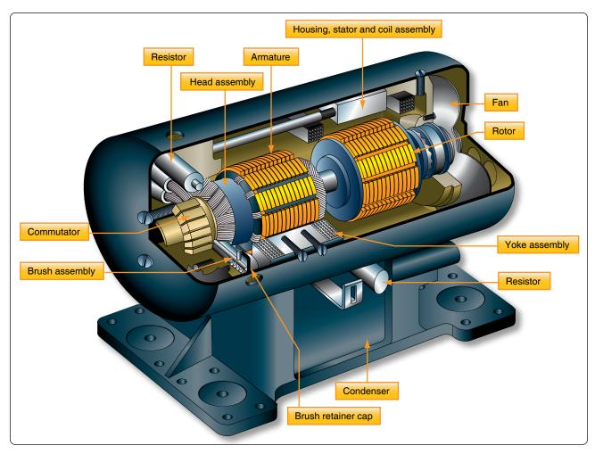
**Figure 12-204.** *Cutaway view of inductor-type rotary inverter.*
