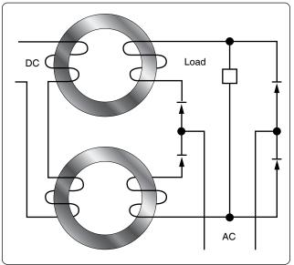
Figure 12-249. Self-saturating, full-wave magnetic amplifier.
