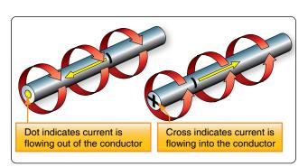
Figure 12-30. Direction of current flow in a conductor.
