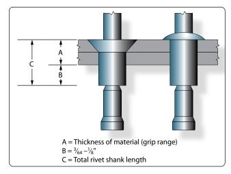
Figure 7-40. Determining length of friction lock rivets.
