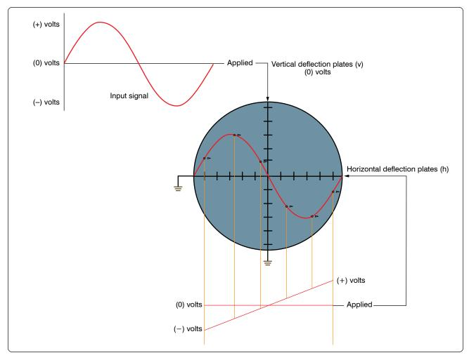
Figure 12-167. Sine wave voltage signal.
