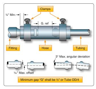
**Figure 9-31.** *Flexible fluid connection assembly.*
