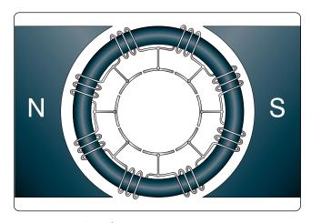
Figure 12-280. An eight-section, ring-type armature.
