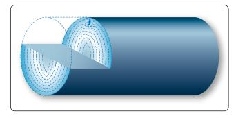
Figure 10-26. Flux leakage at transverse discontinuity.
