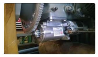
Figure 12-290. DC series starter motor.
