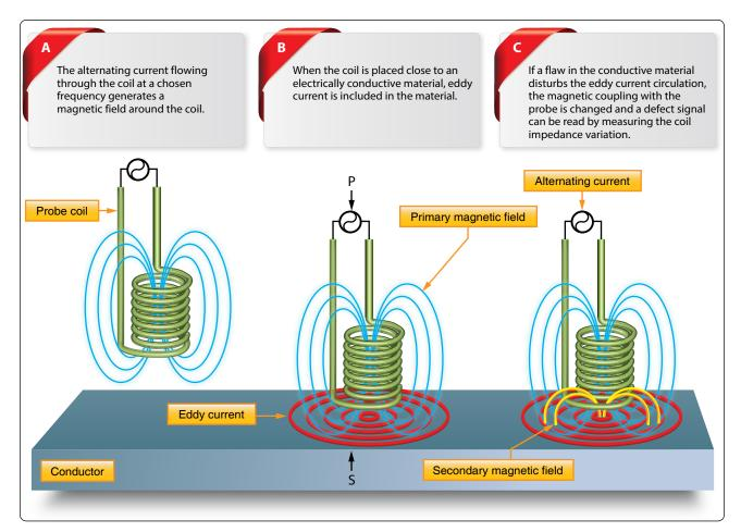
Figure 10-12. Detecting an eddy current.
