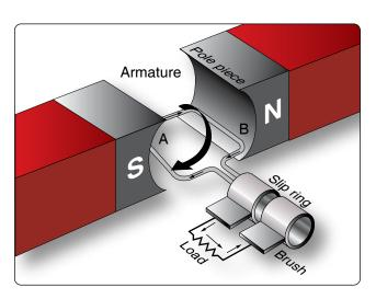
Figure 12-269. Inducing maximum voltage in an elementary generator.
