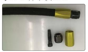
Figure 9-36. MS-type end fitting.
