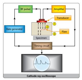
Figure 10-20. Block diagram of basic pulse-echo system.
