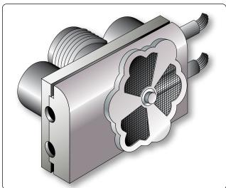
Figure 12-194. A battery quick-disconnect assembly.
