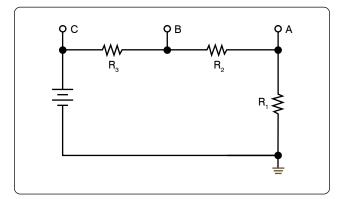
Figure 12-89. A voltage divider circuit.
