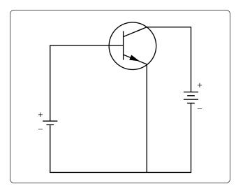
Figure 12-222. NPN transistor.
