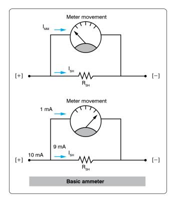
Figure 12-149. Basic meter drawing.
