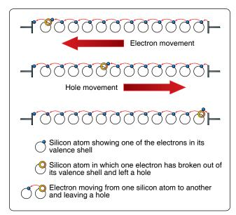
Figure 12-210. A hole moving through atoms.
