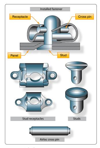
Figure 7-61. Airloc fastener.
