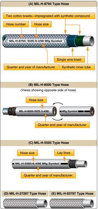
Figure 9-33. Hose identification markings.
