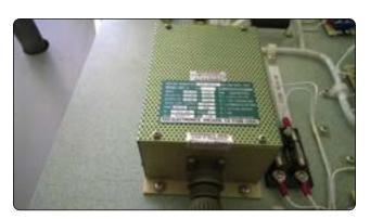
Figure 12-206. Static inverter.
