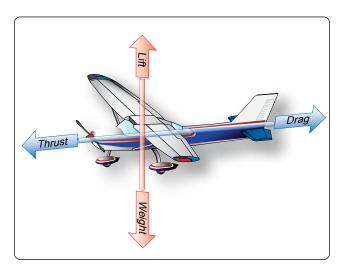
Figure 5-53. Four forces acting on an airplane.
