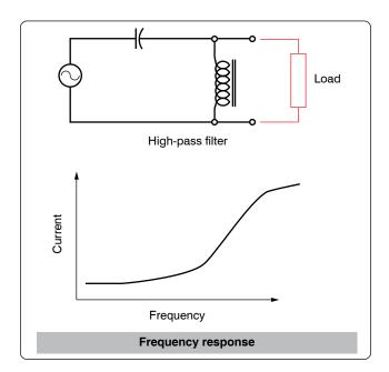
Figure 12-235. High-pass filter.
