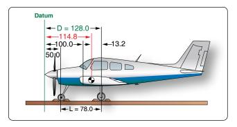
**Figure 6-29.** The datum is 100" forward of the wing root leading edge.
