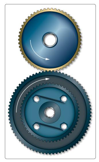
Figure 5-13. Spur gears.
