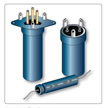
Figure 12-119. Electrolytic capacitors.
