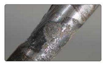
Figure 8-10. Dissimilar metal corrosion.
