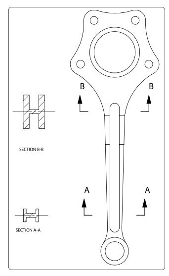
Figure 4-9. Removed sections.
