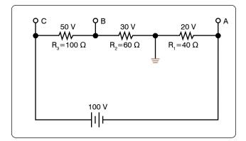
Figure 12-91. Positive and negative voltage on a voltage divider.
