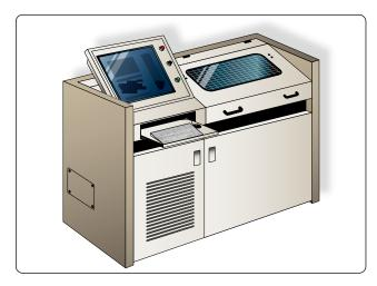
Figure 9-38. Hydraulic hose burst test stand.
