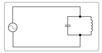
Figure 12-140. A parallel resonant circuit.
