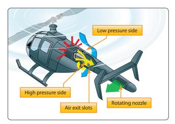
Figure 5-89. Airflow for a NOTAR.
