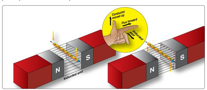
Figure 12-106. An application of the generator left-hand rule.
