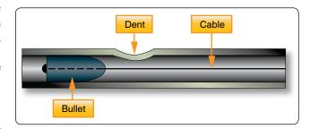
Figure 9-29. Dent removal using a bullet.
