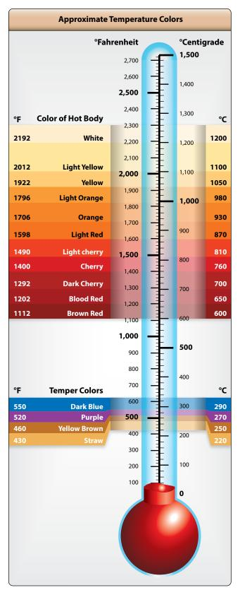
**Figure 7-5.** Temperature chart indicating conversion of Centigrade to Fahrenheit or vice versa, color temperature scale for hardening temperature range, and tempering temperature range.
