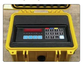
**Figure 6-19.** *M2000 platform scale digital indicator.*
