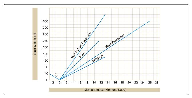
Figure 6-43. Aircraft loading graph.
