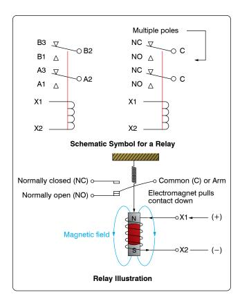
Figure 12-80. Basic relay.
