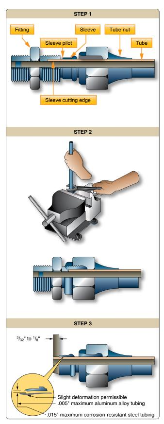
Figure 9-14. Presetting flareless tube assembly.
