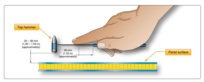
Figure 10-37. Tap testing using hammer.
