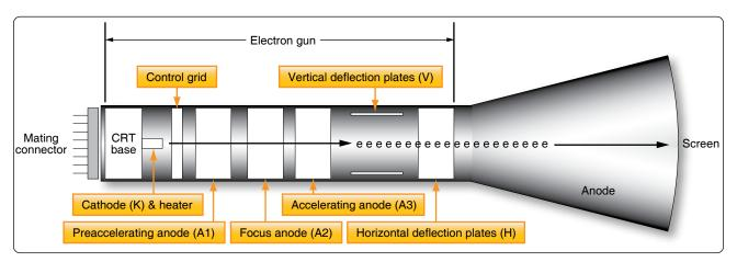
Figure 12-164. Basic components of the CRT with a block diagram.
