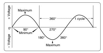
Figure 12-273. *Output of an elementary generator.*
