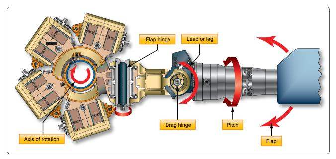
Figure 5-82. Fully articulated main rotor head.
