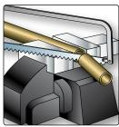
Place hose in vise and cut to desired length using fine tooth hacksaw or cut off wheel
