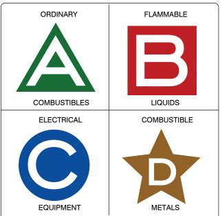
**Figure 1-8.** *Identification of fire extinguisher type location.*
