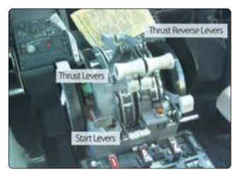
Figure 1-18. Turbofan engine control levers.
