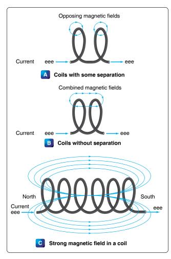
Figure 12-125. Many loops of a coil.
