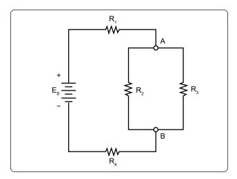
Figure 12-100. Series-parallel circuits.
