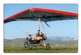
Figure 5-101. Weight-shift control aircraft landing.
