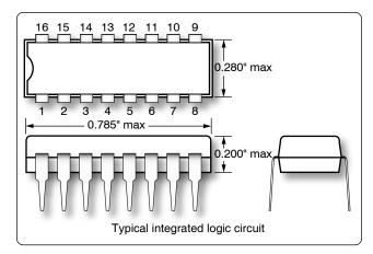
Figure 12-266. Integrated circuit.
