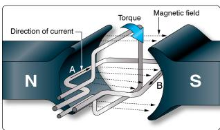
Figure 12-293. Developing a torque.
