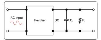
Figure 12-228. A capacitor used as a filter.
