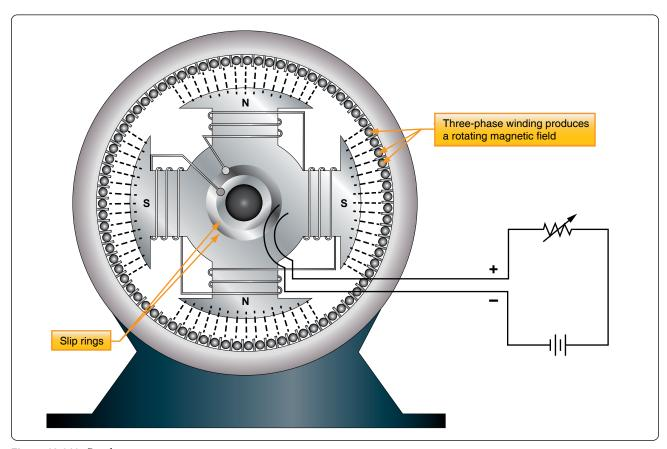
Figure 12-313. Synchronous motor.
