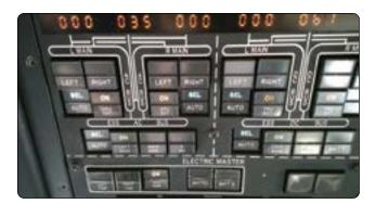
Figure 12-78. Lighted pushbutton switches.
