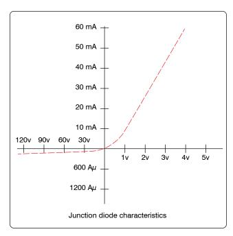
Figure 12-214. Diode biased in both directions.
