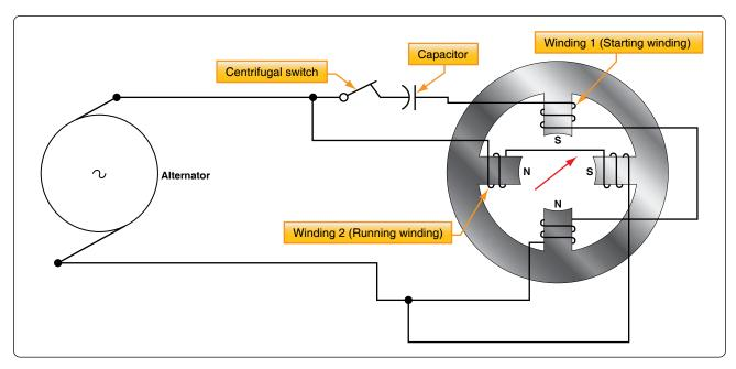
**Figure 12-311.** *Single-phase motor with capacitor starting winding.*
