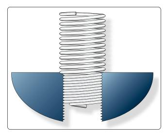
Figure 7-31. Helicoil insert.
