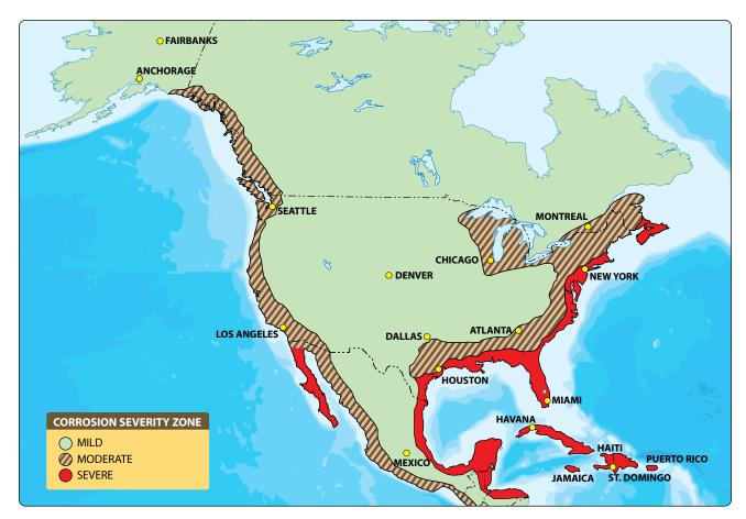
Figure 8-3. North America corrosion severity chart.
