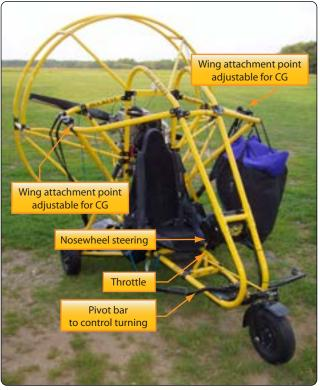
Figure 6-53. Powered parachute structure with wing attach points.
