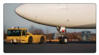
Figure 1-19. Example of a tow tractor.
