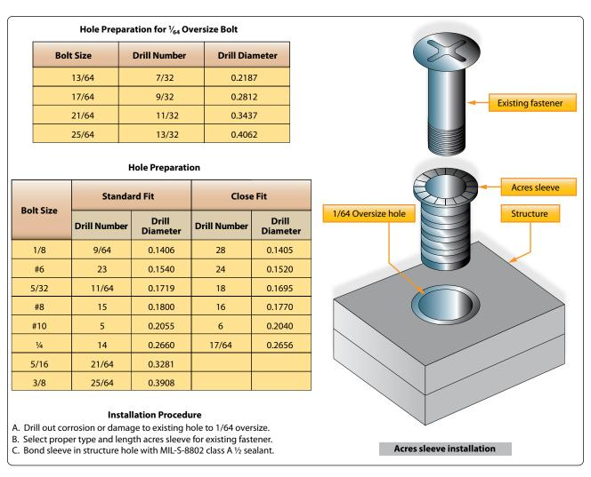
Figure 7-67. Acres sleeve identification, installation, and breakoff procedure.
