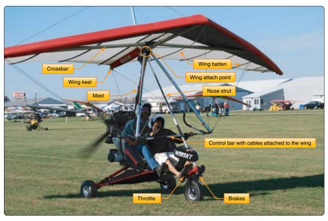
Figure 5-98. Weight-shift control aircraft getting ready for flight.
