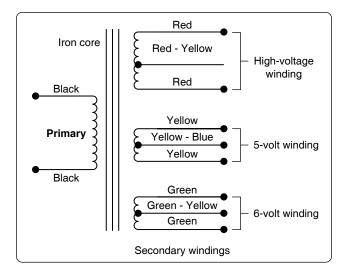
**Figure 12-146.** Schematic symbol for an iron-core power transformer.
