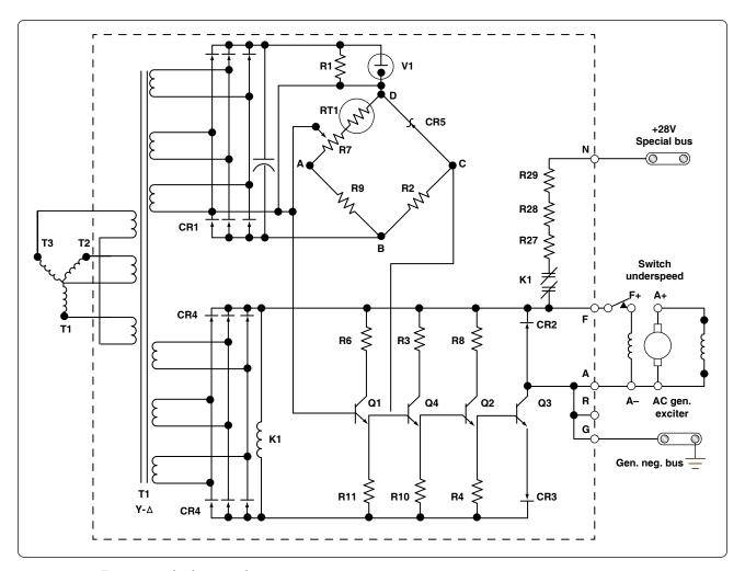
Figure 12-342. Transistorized voltage regulator.
