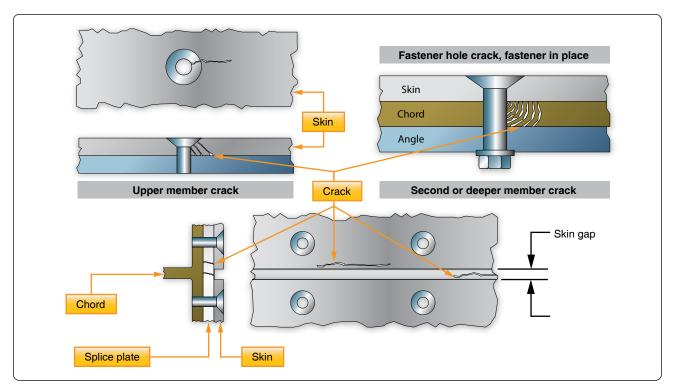
Figure 10-15. Typical subsurface cracks.
