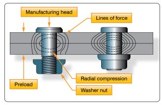
Figure 7-56. Taper-Lok special fasteners
