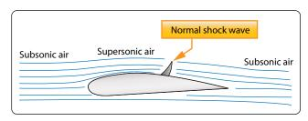
Figure 5-77. Normal shock wave.
