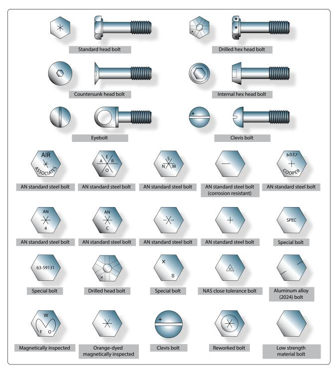
Figure 7-19. Aircraft bolt identification.
