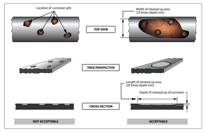
Figure 8-23. Blending or blending corrosion damage.
