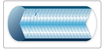
**Figure 10-27.** Flux leakage at longitudinal discontinuity.
