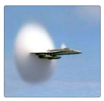
Figure 5-52. F-18 high-speed fly-by and a vapor cloud.
