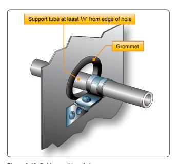
Figure 9-42. Rubber-cushioned clamp.
