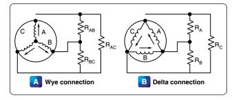
Figure 12-321. Wye and delta connected alternators.
