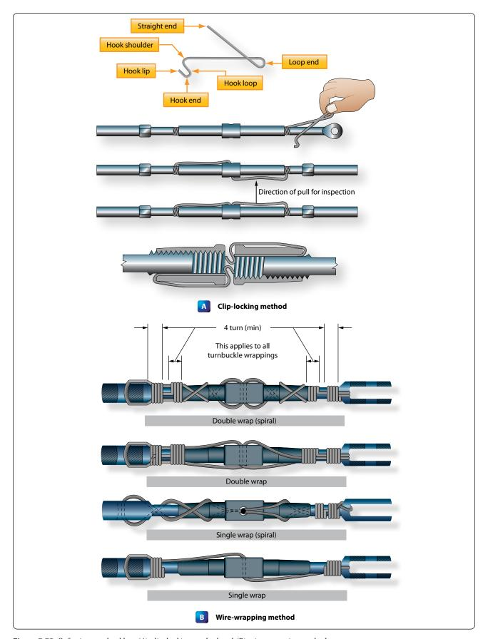
Figure 7-75. Safetying turnbuckles: (A) clip-locking method and (B) wire-wrapping method.
