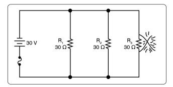
**Figure 12-186.** A shorted component causes the fuse to open.
