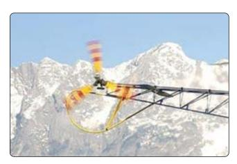
Figure 5-86. Aerospatiale helicopter tail rotor.
