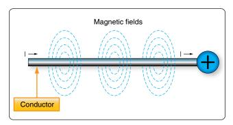
Figure 12-26. Magnetic field formed around a conductor in which current is flowing.
