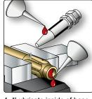
4. \*Lubricate inside of hose and nipple threads liberally.
