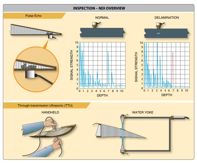
**Figure 10-19.** *Through-transmission and pulse echo indications.*
