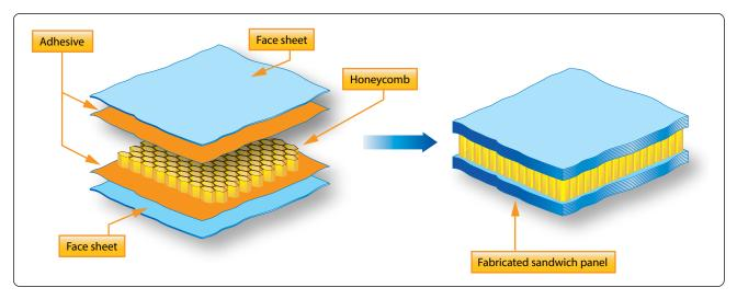
Figure 7-14. Sandwich structure.
