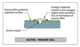
Figure 8-13. Active-passive cell.
