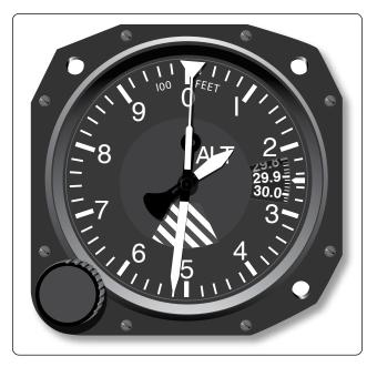
Figure 5-51. An airplane's altimeter is an aneroid barometer.
