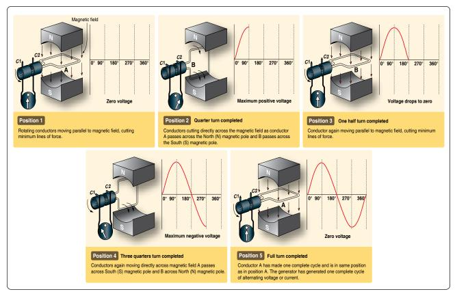
Figure 12-109. Generation of a sine wave.
