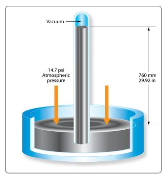
**Figure 5-33.** *Atmospheric pressure as inches of mercury.*
