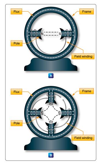
**Figure 12-278.** *A two-pole and a four-pole frame assembly.*
