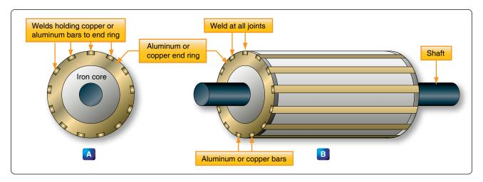
Figure 12-308. Squirrel cage rotor for an AC induction motor.
