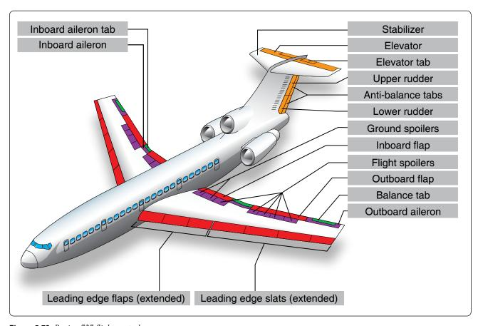
Figure 5-72. Boeing 727 flight controls.
