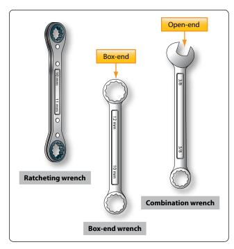
Figure 11-7. Ratcheting, box-end, and combination wrenches.
