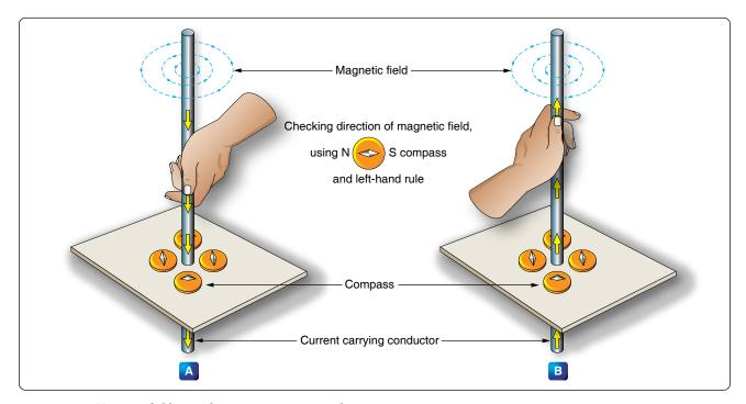
**Figure 12-28.** *Magnetic field around a current-carrying conductor.*
