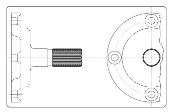
Figure 4-13. Symmetrical object with exterior half view.
