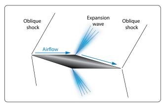
Figure 5-78. Supersonic airfoil with oblique shock waves and expansion waves.
