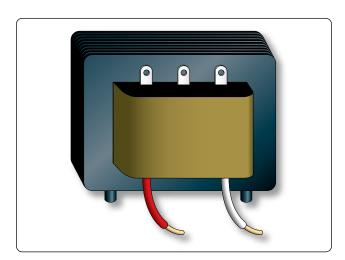
Figure 12-145. Power supply transformer.
