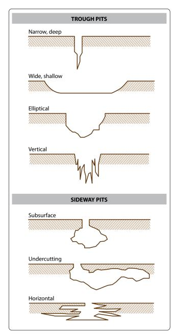
Figure 8-9. Types of pitting corrosion.
