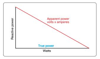
Figure 12-141. Power relations in AC circuit.
