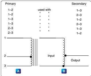
Figure 12-148. Autotransformers.
