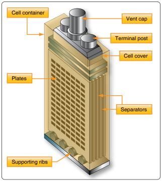
Figure 12-191. Lead-acid cell construction.
