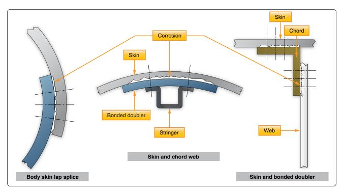
Figure 10-16. Typical structural corrosion.
