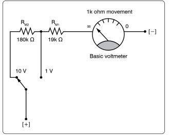
Figure 12-153. Two range voltmeter.
