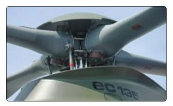
Figure 5-85. Eurocopter Model 135 rigid rotor system.
