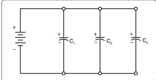
Figure 12-122. Simplified parallel circuit.
