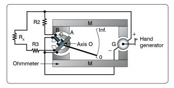
Figure 12-158. Simplified megger circuit.
