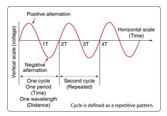
Figure 12-110. Cycle of voltage.
