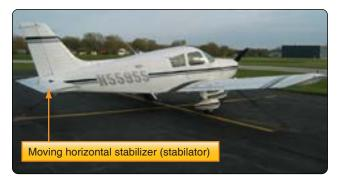
**Figure 5-66.** Moving horizontal stabilizer, known as a stabilator, on a Piper Cherokee Cruiser PA-28-140 provides pitch control.
