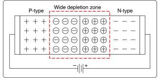
Figure 12-213. Reversed diode.
