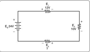
Figure 12-87. Determine the unknown voltage drop.
