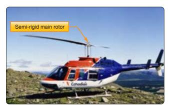
Figure 5-84. Bell Jet Ranger with semi-rigid main rotor.
