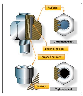
Figure 7-27. Stainless steel self-locking nut.
