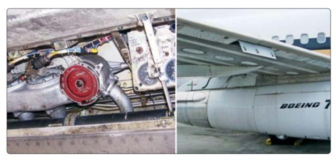
Figure 1-33. Single point refueling station of a large aircraft.
