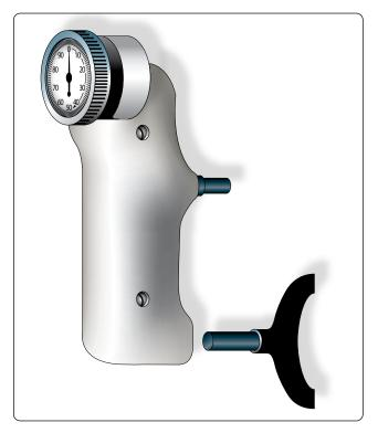
**Figure 7-12.** *Barcol portable hardness tester.*
