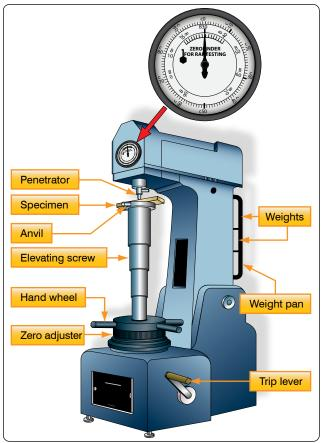
Figure 7-10. Rockwell hardness tester.
