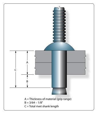
Figure 7-42. Determining length of pull-thru rivets.
