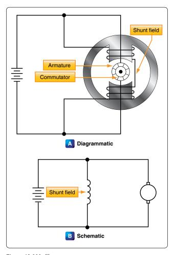
Figure 12-300. Shunt motor.
