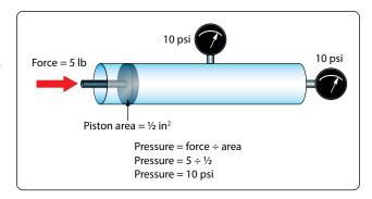
Figure 5-43. Pressure created in a hydraulic system.
