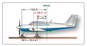
Figure 6-30. The datum is aft of the main wheels at the wing trailing edge.
