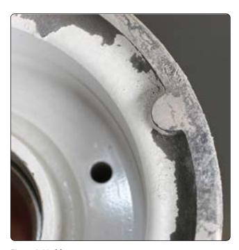
Figure 8-29. Magnesium corrosion.
