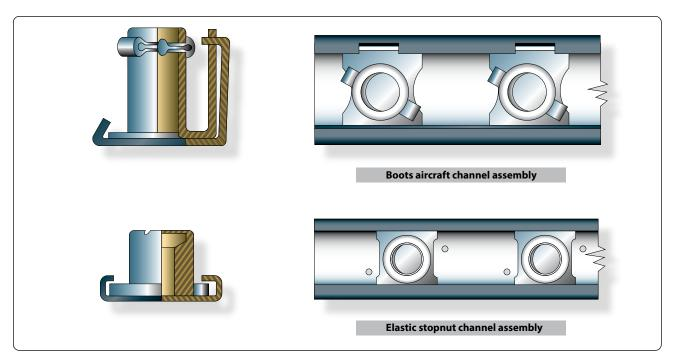
Figure 7-29. Self-locking nut bases.
