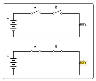
Figure 12-256. Simplified diagram of the AND logic.
