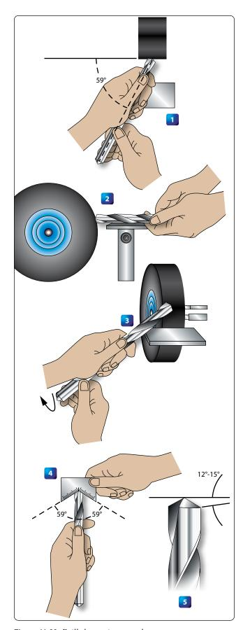
Figure 11-22. Drill sharpening procedures.
