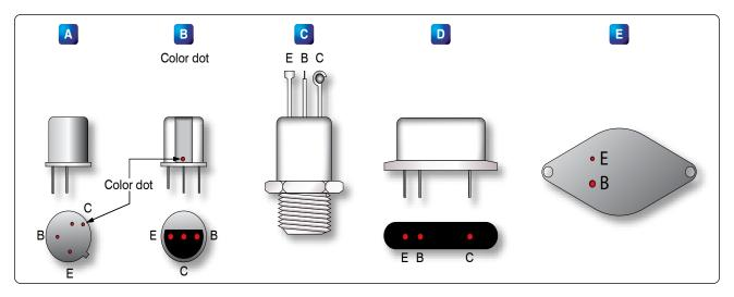
Figure 12-224. Common transistor lead identifications.
