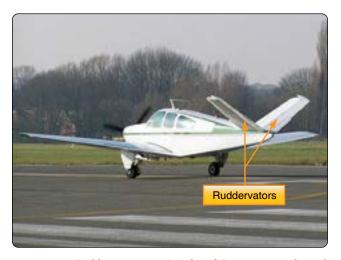
Figure 5-67. Ruddervators on a Beechcraft Bonanza provide pitch control.
