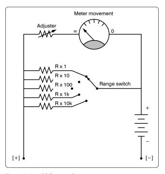
Figure 12-157. Multirange ohmmeter.
