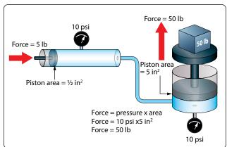
Figure 5-44. Output force created in a hydraulic system.
