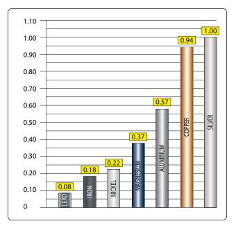
Figure 5-27. Conductivity of various metals.
