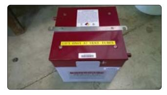
Figure 12-199. Sealed battery.
