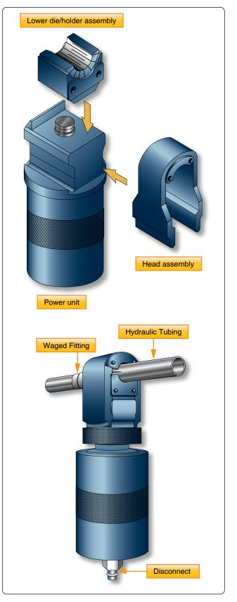
Figure 9-24. Swaged fitting tooling.
