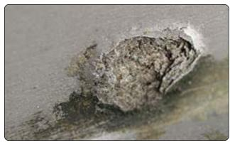
Figure 8-15. Exfoliation corrosion.
