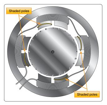
Figure 12-309. Shaded pole induction motor.
