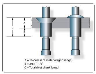
Figure 7-50. Determining rivet length.
