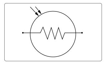
Figure 12-66. Photoconductive cell schematic symbol component.
