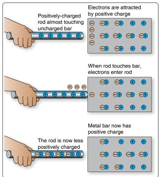
Figure 12-7. Charging by contact.
