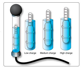
Figure 12-195. Hydrometer (specific gravity readings).
