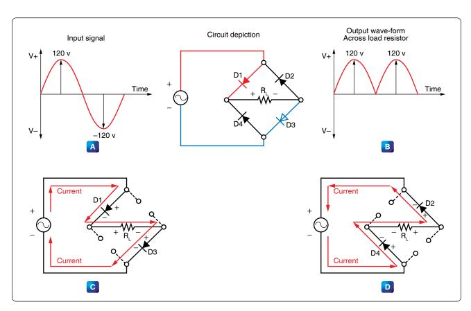
Figure 12-216. Full-wave bridge rectifier.
