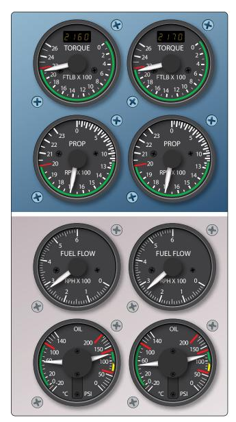
Figure 1-15. Typical examples of turboprop instruments.
