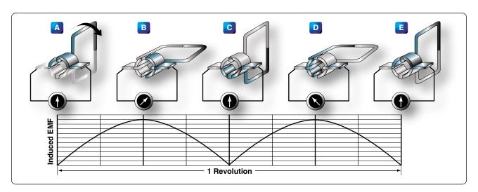
**Figure 12-275.** *Operation of a basic DC generator.*
