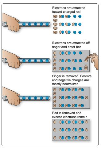
Figure 12-8. Charging a bar by induction.
