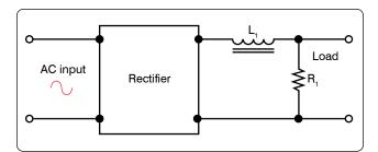
Figure 12-230. An inductor used as a filter.
