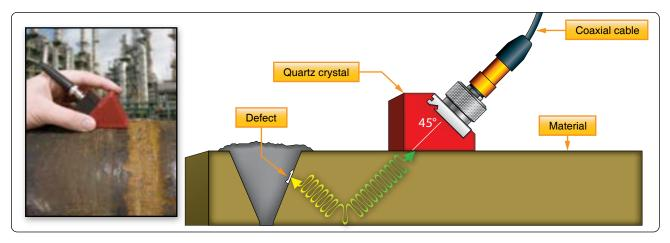
Figure 10-22. Pulse-echo angle beam testing.
