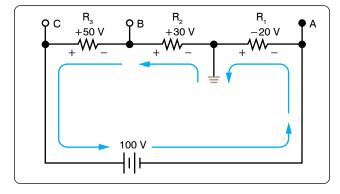
Figure 12-92. Current flow through a voltage divider.
