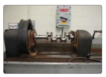
Figure 10-29. Circular magnetization of a crankshaft.
