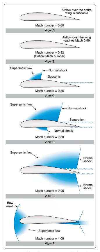
**Figure 5-79.** *Airflow with progressively greater Mach numbers.*
