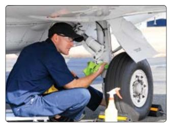
Figure 8-20. The landing gear area should be cleaned and inspected more frequently than other areas.
