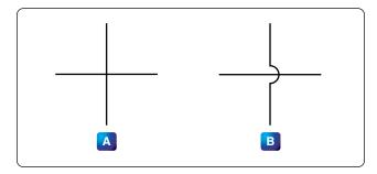
Figure 12-45. Unconnected crossover wires.
