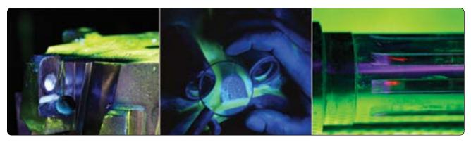
Figure 10-9. Dye penetrant inspection.
