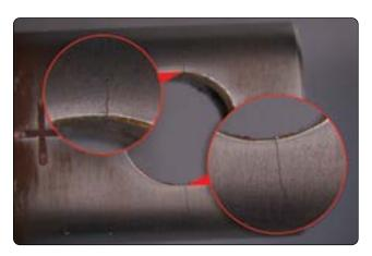
**Figure 10-31.** Fatigue crack on the bottom end fitting of a Hydrosorb shock absorber.
