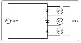
Figure 12-233. Stacking diodes in a circuit.
