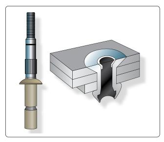
Figure 7-45. Wiredraw CherryLOCK® rivet.
