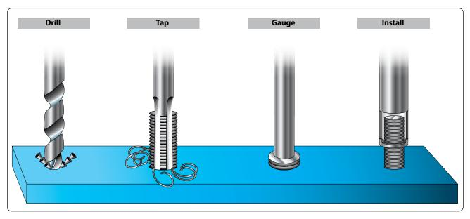
Figure 7-32. Helicoil installation.
