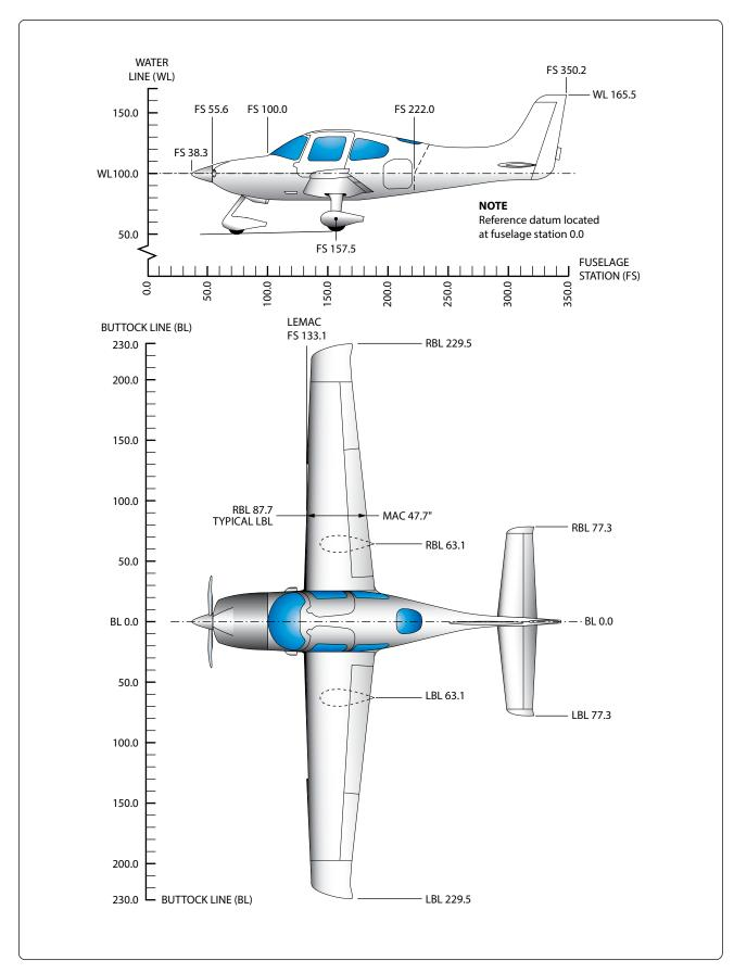
Figure 4-10. Station numbers and location identification on aircraft.
