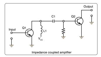
Figure 12-243. Simplified impedance coupling circuit.
