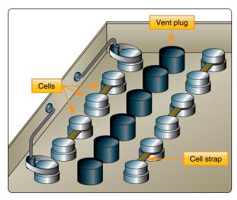
Figure 12-193. Connection of storage battery.
