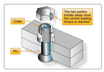
Figure 7-57. HI- $TIGUE^{TM}$  special fasteners.
