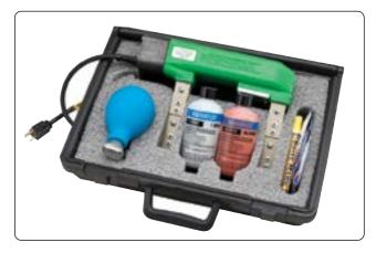
Figure 10-34. Portable magnetic particle inspection equipment.
