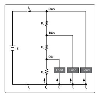
Figure 12-90. A typical voltage divider.
