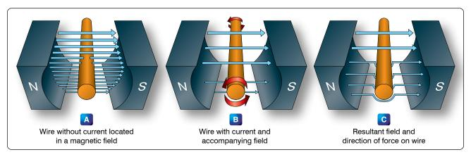
Figure 12-291. Force on a current carrying wire.
