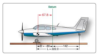
**Figure 6-32.** The datum is aft of the main wheels, at the intersection of the wing trailing edge and the fuselage.
