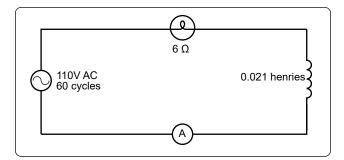
Figure 12-135. A circuit containing resistance and inductance.
