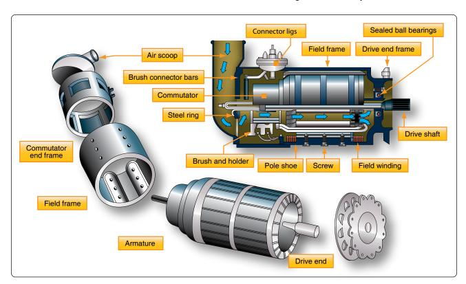
Figure 12-277. Typical 24-volt aircraft generator.
