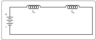
Figure 12-128. Two inductors in series.
