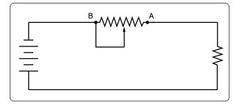
Figure 12-59. Rheostat connected in series.
