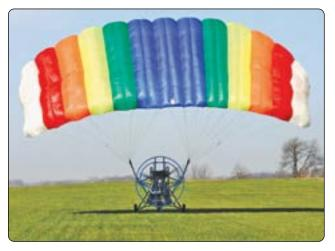
Figure 5-104. Powered parachute wing trailing edge.
