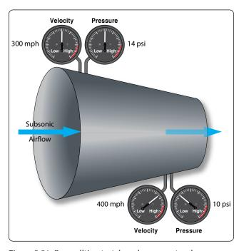
**Figure 5-54.** Bernoulli's principle and a converging duct.
