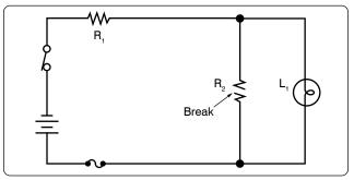
Figure 12-188. An open in the parallel portion of a series-parallel circuit
