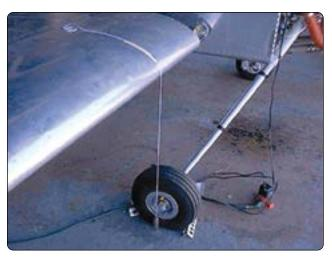
Figure 6-22. Plumb bob dropped from a wing leading edge.
