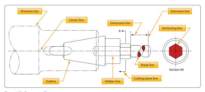
Figure 4-25. Correct use of lines.
