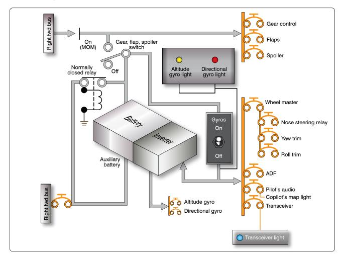
Figure 12-208. Auxiliary battery system using static inverter.
