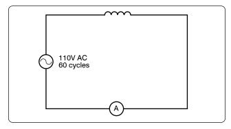
Figure 12-130. AC circuit containing inductance.
