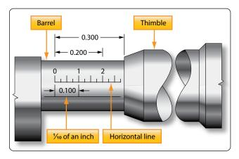
$\textbf{Figure 11-37}. \ \textit{Micrometer measurements}.$
