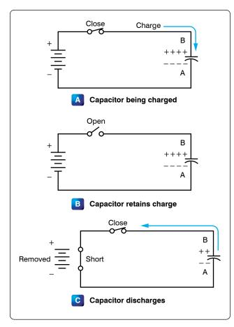
Figure 12-114. Capacitors in direct current.
