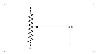
**Figure 12-62.** *Potentiometer wired to function as rheostat.*
