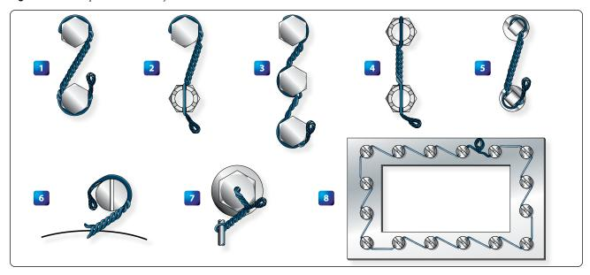
Figure 7-72. Safety wiring methods.
