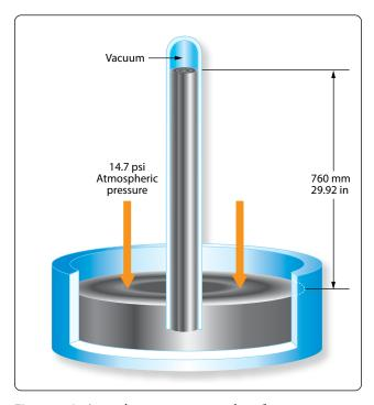
Figure 5-50. Atmospheric pressure as inches of mercury.
