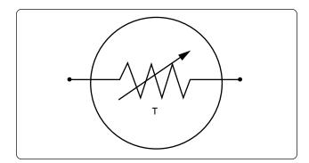
Figure 12-65. Schematic symbol for thermistor.
