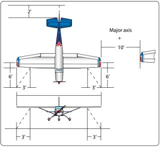
Figure 1-9. Diagram of tiedown dimensions.
