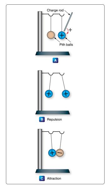
Figure 12-6. Reaction of like and unlike charges.
