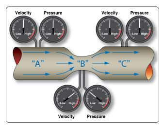
Figure 5-46. Bernoulli's principle and a venturi.
