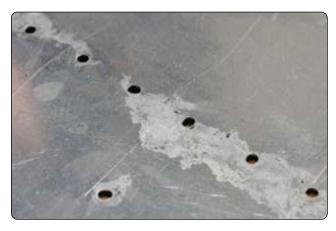
Figure 8-7. Surface corrosion.
