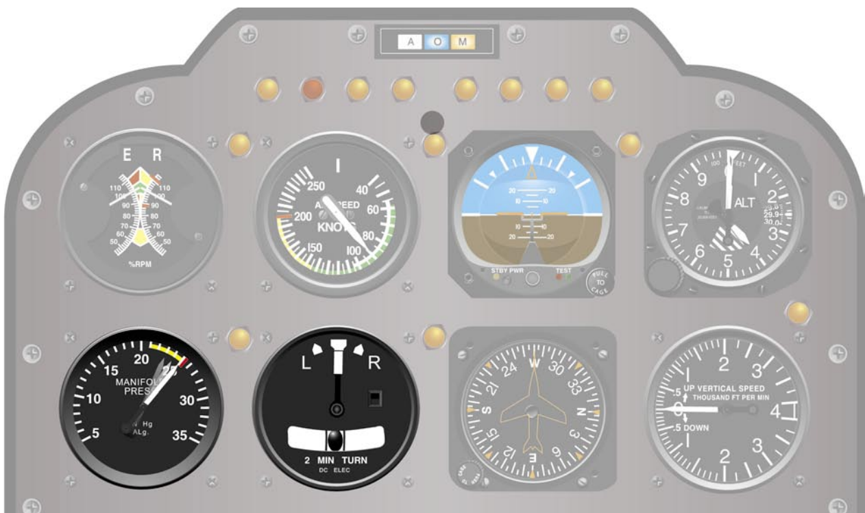
Figure 6-6. Coordinated flight is indicated by centering of the ball.
