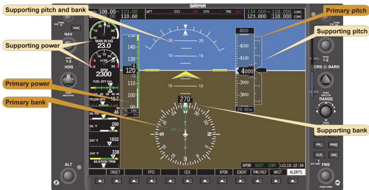
Figure 5-57. Straight-and-Level Flight (Normal Cruising Speed).
