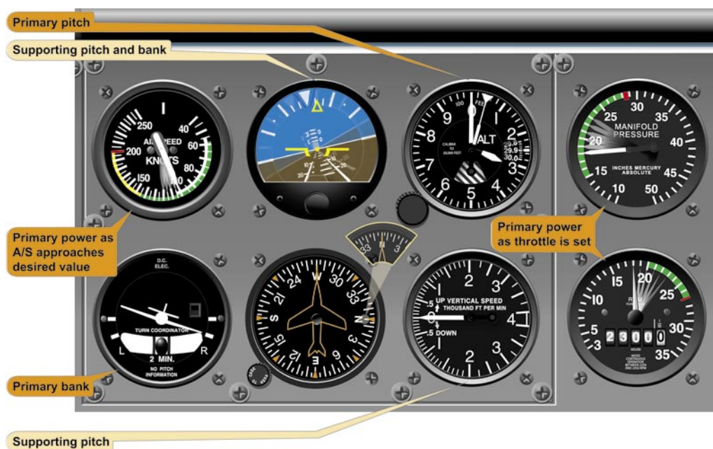
Figure 5-38. Change of Airspeed During Turn.
