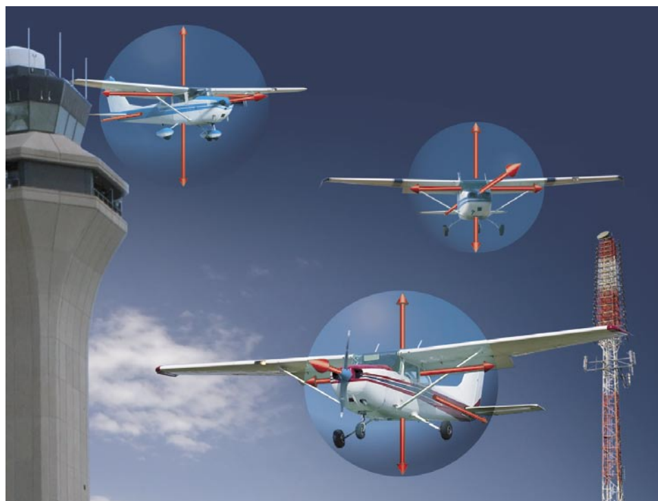
Figure 3-48. Aircraft equipped with Automatic Dependent Surveillance—Broadcast (ADS-B) continuously broadcast their identification, altitude, direction, and vertical trend. The transmitted signal carries significant information for other aircraft and ground stations alike. Other ADS-equipped aircraft receive this information and process it in a variety of ways. It is possible that in a saturated environment (assuming all aircraft are ADS equipped), the systems can project tracks for their respective aircraft and retransmit to other aircraft their projected tracks, thereby enhancing collision avoidance. At one time, there was an Automatic Dependent Surveillance—Addressed (ADS-A) and that is explained in the Pilot's Handbook of Aeronautical Knowledge.
