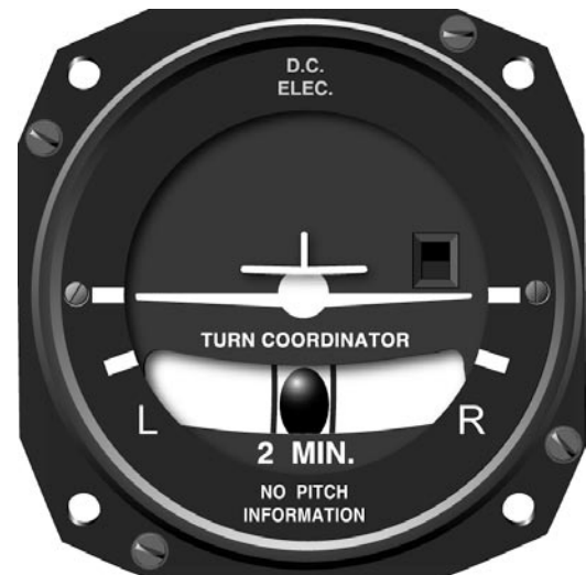
Figure 3-35. A turn coordinator senses rotation about both roll and yaw axes.
