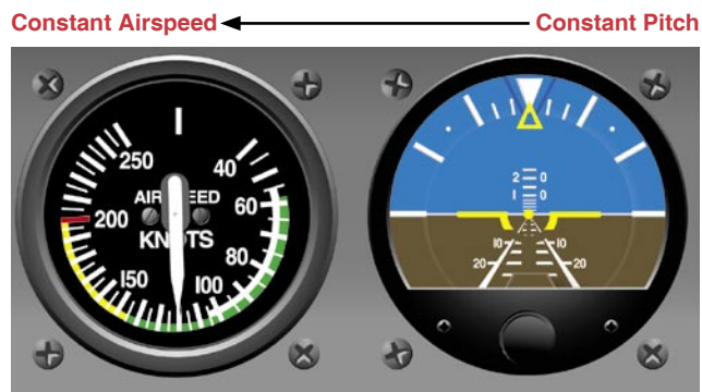
Figure 5-13. Constant Power Plus Constant Pitch Equals Constant Speed.
