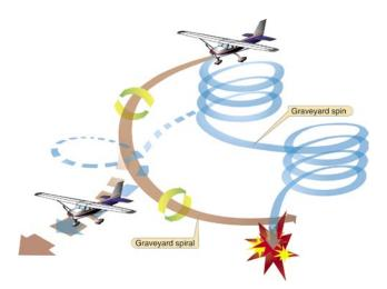
Figure 16-5. Graveyard spiral.
