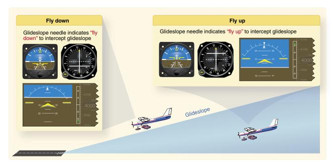
**Figure 2-22.** Analog and digital indications for glideslope interception.
