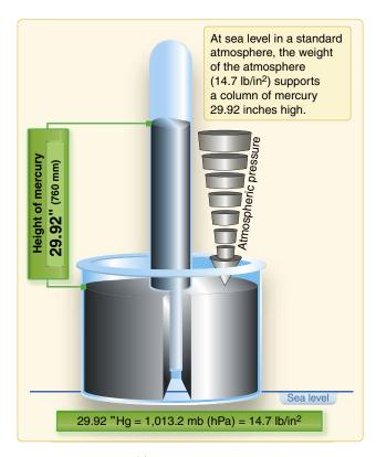
Figure 11-6. Mercurial barometer.
