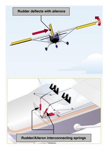
**Figure 5-8.** *Coupled ailerons and rudder.*
