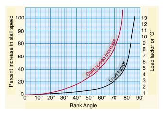
Figure 4-33. Increase in stall speed and load factor.
