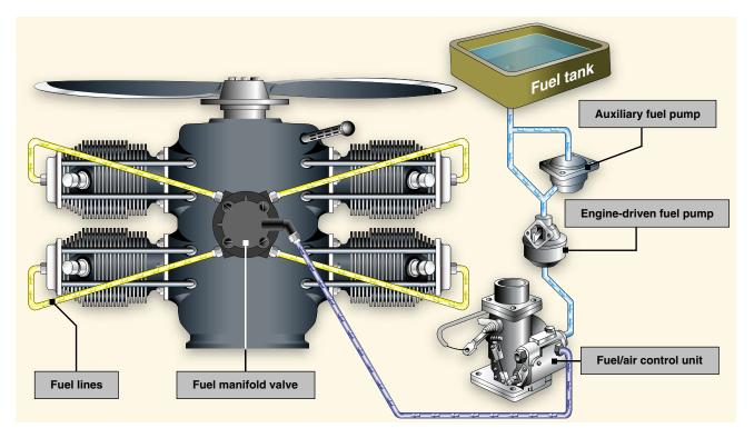
Figure 6-13. Fuel injection system.
