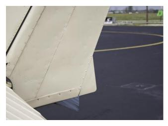
**Figure 5-22.** A ground adjustable tab is used on the rudder of many small airplanes to correct for a tendency to fly with the fuselage slightly misaligned with the relative wind.
