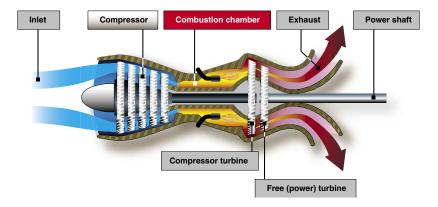
Figure 6-26. Turboshaft engine.
