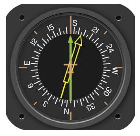
**Figure 7-30.** Driven by signals from a flux valve, the compass card in this RMI indicates the heading of the aircraft opposite the upper center index mark. The green pointer is driven by the ADF.
