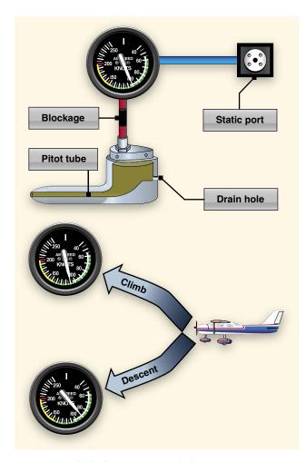
Figure 7-10. Blocked pitot system with clear static system.
