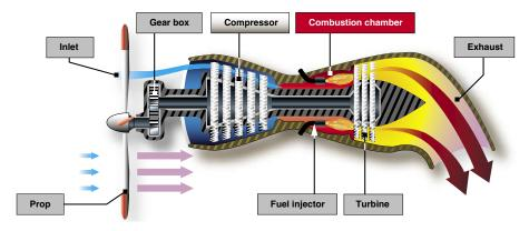
Figure 6-24. Turboprop engine.
