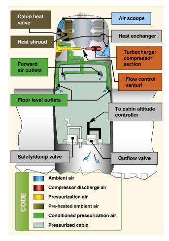
**Figure 6-40.** *High performance airplane pressurization system.*
