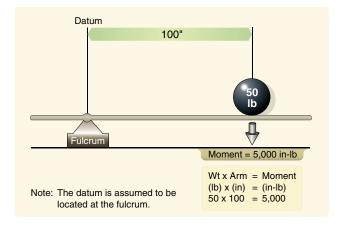
Figure 9-3. Determining moment.
