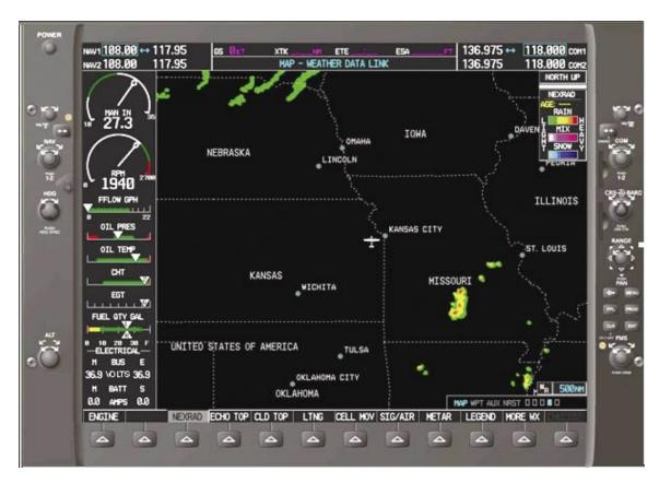
**Figure 12-24.** NEXRAD radar display (500 mile range). The individual color gradients can be easily discerned and interpreted via the legend in the upper right corner of the screen. Additional information can be gained by pressing the LEGEND soft key, which displays the legend page.
