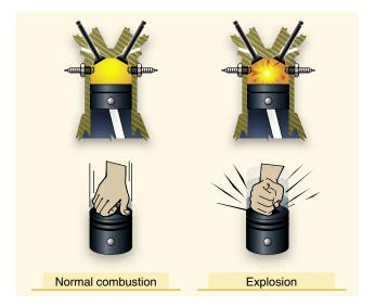
Figure 6-21. Normal combustion and explosive combustion.
