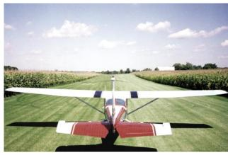
Figure 10-15. An aircraft's performance depends greatly on the runway surface.
