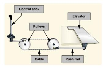
Figure 5-1. Mechanical flight control system.
