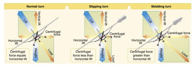
Figure 4-29. Normal, slipping, and skidding turns.
