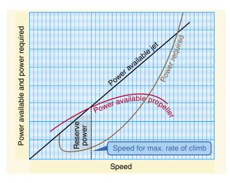
Figure 10-8. Power versus climb rate.
