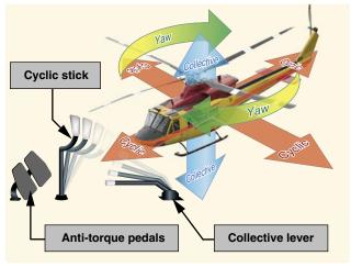
Figure 5-3. Helicopter flight control system.
