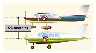
Figure 4-26. Keel area for lateral stability.
