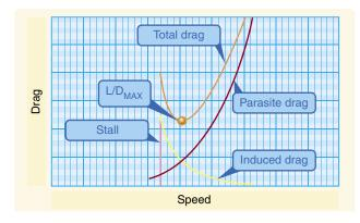
Figure 10-5. Drag versus speed.
