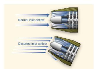
**Figure 6-28.** Comparison of normal and distorted airflow into the compressor section.
