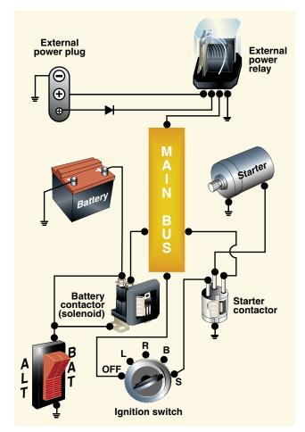
Figure 6-20. Typical starting circuit.
