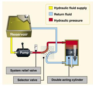
Figure 6-36. Basic hydraulic system.
