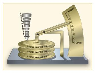
Figure 11-7. Aneroid barometer.
