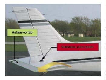
Figure 2-11. Stabilator components.
