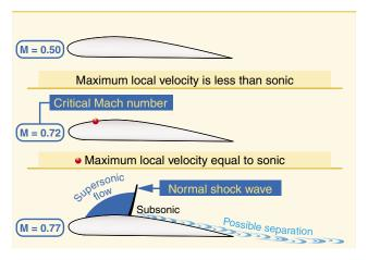
Figure 4-56. Wing airflow.
