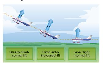
Figure 4-30. Changes in lift during climb entry.
