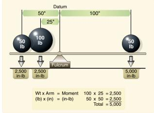
Figure 9-4. Establishing a balance.
