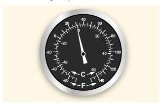
**Figure 7-38.** *Outside air temperature (OAT) gauge.*
