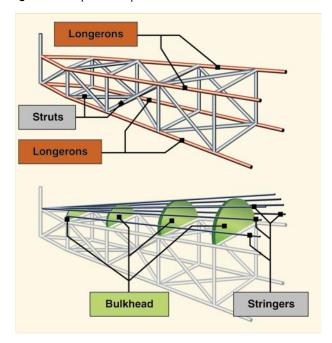
Figure 2-5. Truss-type fuselage structure.
