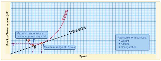
Figure 10-10. Airspeed for maximum endurance.
