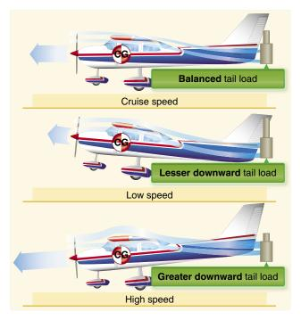
Figure 4-21. Effect of speed on downwash.
