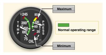
**Figure 8-3.** *Minimum, maximum, and normal operating range markings on oil gauge.*
