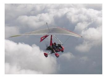
Figure 4-16. A weight-shift control aircraft.
