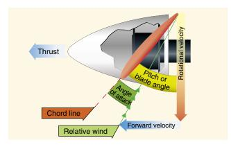
Figure 4-36. Propeller blade angle.
