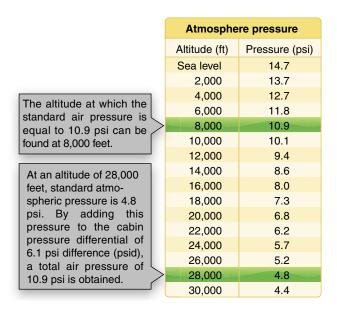
Figure 6-41. Standard atmospheric pressure chart.
