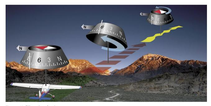
Figure 7-36. Effects of acceleration error.
