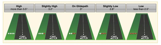
Figure 13-8. Precision approach path indicator.
