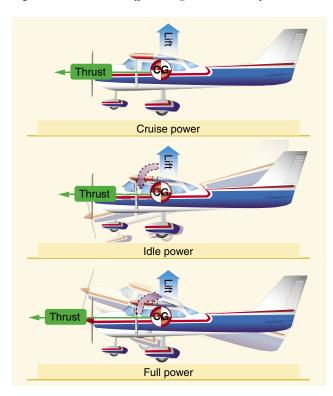
**Figure 4-24.** *Power changes affect longitudinal stability.*
