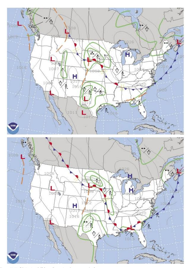
Figure 12-20. 36- (top) and 48-hour (bottom) surface prognostic chart.
