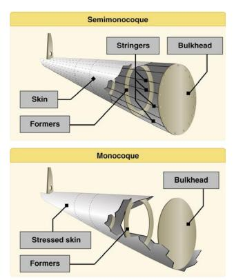
Figure 2-14. Semimonocoque and monocoque fuselage design.
