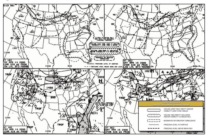
Figure 12-19. Significant weather prognostic chart and legend (inset).
