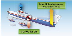
If the CG is too far aft, there might not be enough elevator nosedown force at the low stall airspeed to get the nose down for recovery.
