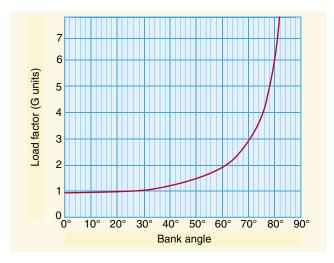
Figure 4-45. Angle of bank changes load factor.
