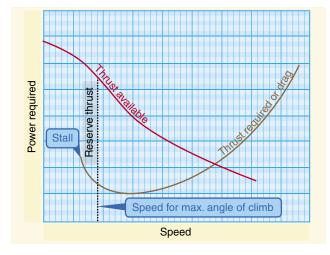
Figure 10-7. Thrust versus climb angle.
