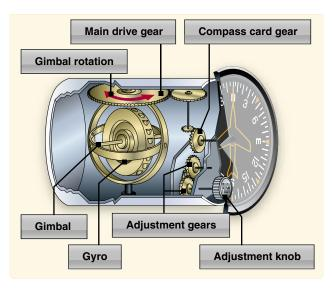
**Figure 7-25.** A heading indicator displays headings based on a 360° azimuth, with the final zero omitted. For example, "6" represents 060°, while "21" indicates 210°. The adjustment knob is used to align the heading indicator with the magnetic compass.
