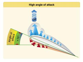
**Figure 3-8.** Pressure distribution on an airfoil and CP changes with AOA.
