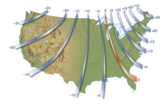
**Figure 7-32.** *Isogonic lines are lines of equal variation.*
