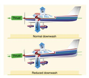
Figure 4-22. Reduced power allows pitch down.
