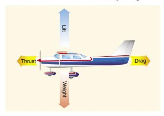
Figure 4-1. Relationship of forces acting on an airplane.
