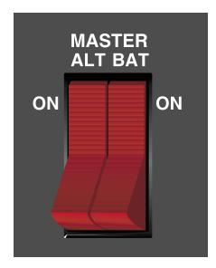
**Figure 6-33.** On this master switch, the left half is for the alternator and the right half is for the battery.
