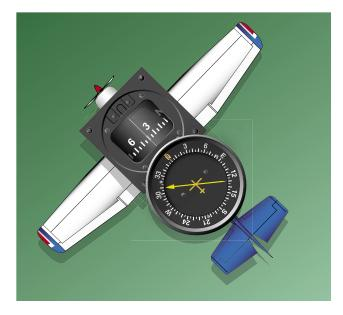
**Figure 15-36.** *ADF with fixed azimuth and magnetic compass.*
