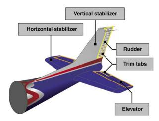
Figure 2-10. Empennage components.
