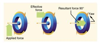
Figure 4-41. Gyroscopic precession.
