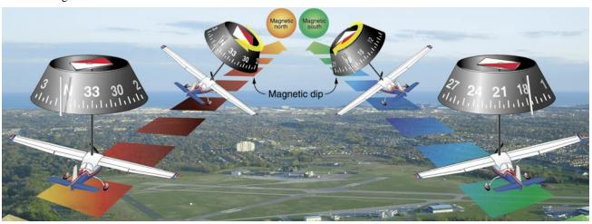
Figure 7-35. Northerly turning error.
