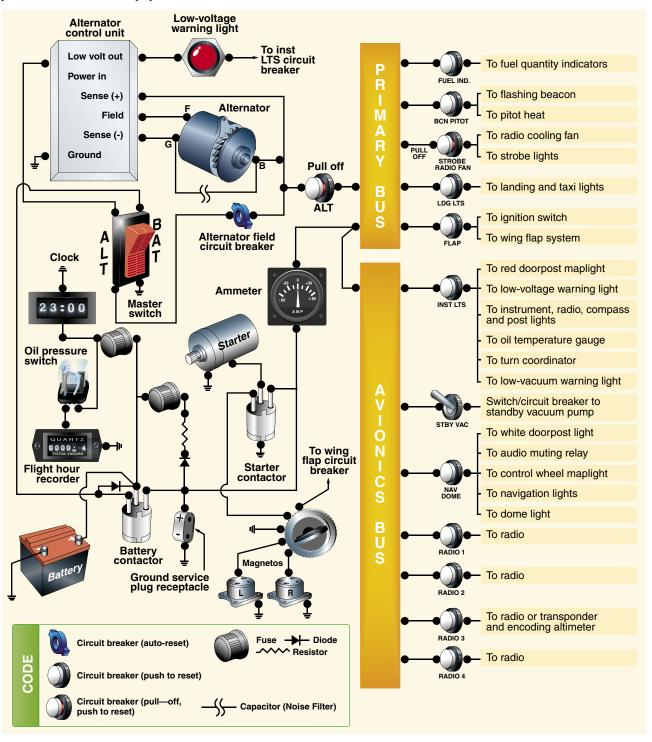
Figure 6-34. *Electrical system schematic*.
