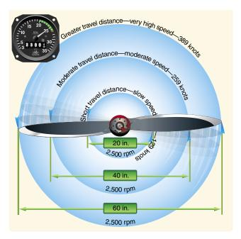
**Figure 4-38.** *Propeller tips travel faster than the hub.*
