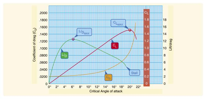
Figure 4-9. Lift coefficients at various angles of attack.
