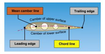
Figure 3-6. Typical airfoil section.
