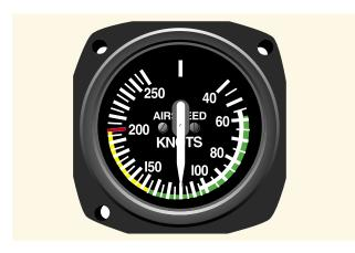
Figure 8-1. Single-engine airpseed indicator.
