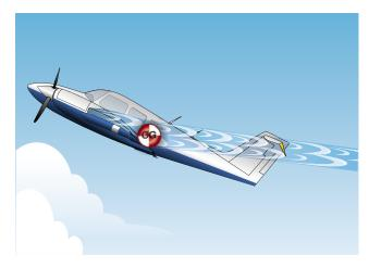
**Figure 5-11.** Airplane with a T-tail design at a high AOA and an aft CG.
