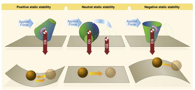
Figure 4-18. Types of static stability.
