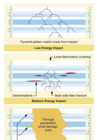
Figure 2-16. Impact energy affects the visibility, as well as the severity, of damage in composite structures. High and medium energy impacts, while severe, are easy to detect. Low energy impacts can easily cause hidden damage.
