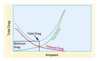
Figure 4-8. Drag versus speed.
