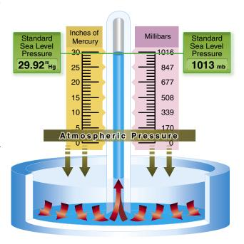
Figure 10-1. Standard sea level pressure.
