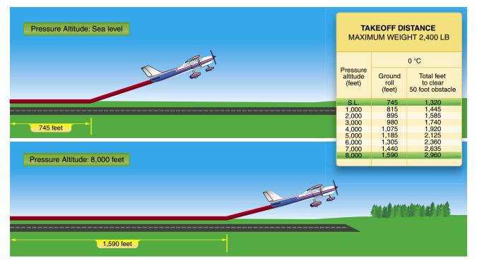
Figure 11-9. Takeoff distances increase with increased altitude.
