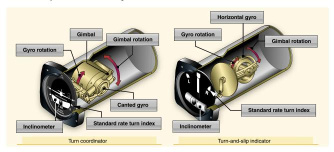
Figure 7-21. Turn indicators rely on controlled precession for their operation.
