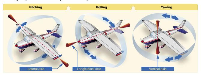
Figure 4-15. Axes of an airplane.
