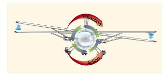
Figure 4-39. Torque reaction.
