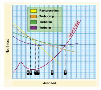
Figure 6-29. Engine net thrust versus aircraft speed and drag. Points
