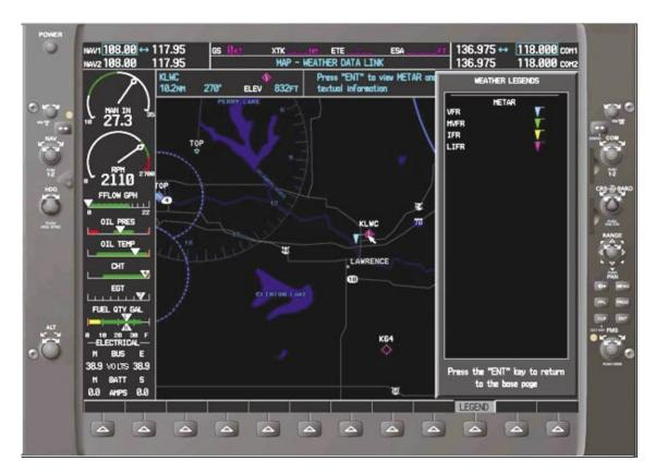
Figure 12-27. Graphical METAR legend display.
