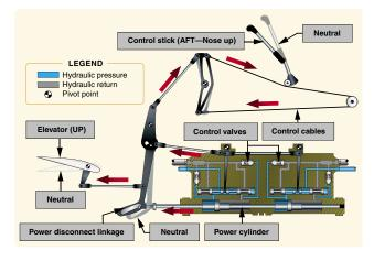
**Figure 5-2.** *Hydromechanical flight control system.*
