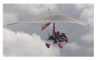
**Figure 2-9.** Weight-shift control aircraft use the shifting of weight for control.
