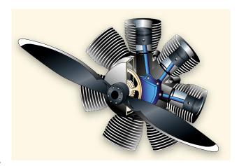
Figure 6-1. Radial engine.
