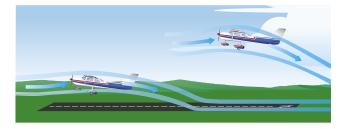
Figure 4-13. Ground effect changes airflow.
