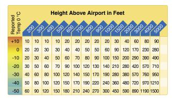
**Figure 7-4.** Look at the chart using a temperature of -10 °C and the aircraft altitude is 1,000 feet above the airport elevation. The chart shows that the reported current altimeter setting may place the aircraft as much as 100 feet below the altitude indicated by the altimeter.
