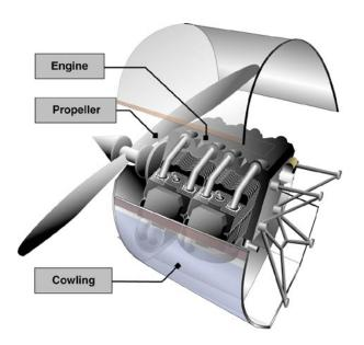
Figure 2-13. Engine compartment.
