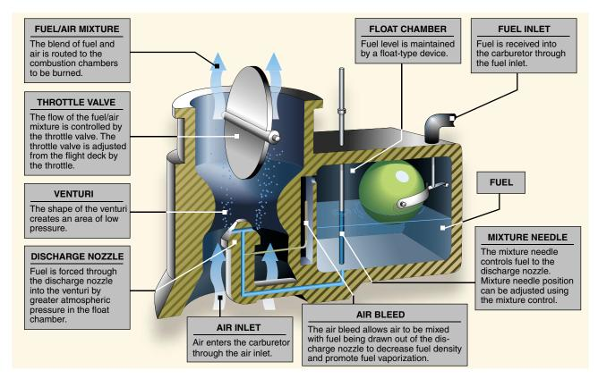
Figure 6-10. Float-type carburetor.
