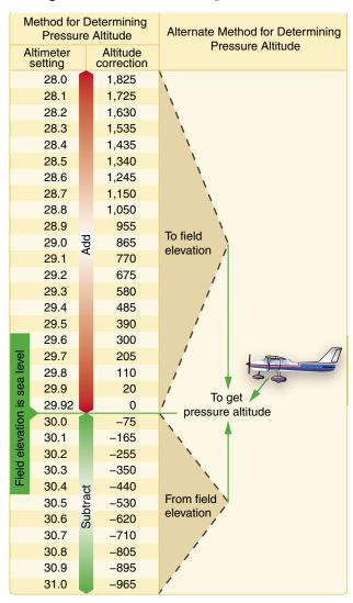
**Figure 10-3.** Field elevation versus pressure. The aircraft is located on a field which happens to be at sea level. Set the altimeter to the current altimeter setting (29.7). The difference of 205 feet is added to the elevation or a PA of 205 feet.
