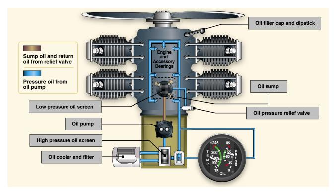
Figure 6-17. Wet-sump oil system.
