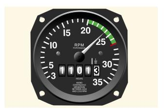
**Figure 6-8.** *Engine rpm is indicated on the tachometer.*
