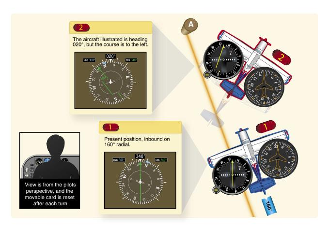
**Figure 2-21.** A comparison of navigation information as depicted on both analog and digital displays.
