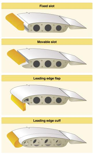
**Figure 5-18.** *Leading edge high lift devices.*
