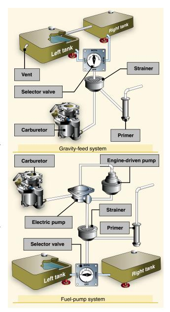
**Figure 6-30.** *Gravity-feed and fuel-pump systems.*
