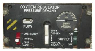
Figure 6-43. Oxygen system regulator.
