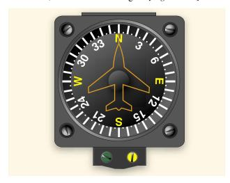
Figure 7-37. Vertical card compass.
