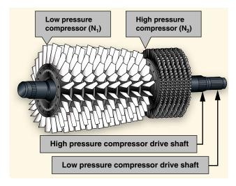
Figure 6-27. Dual-spool axial-flow compressor.
