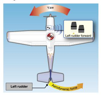
Figure 5-15. The effect of left rudder pressure.
