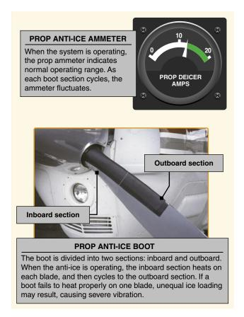
**Figure 6-49.** *Prop ammeter and anti-ice boots.*
