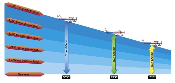
**Figure 7-3.** *Effects of nonstandard temperature on an altimeter.*
