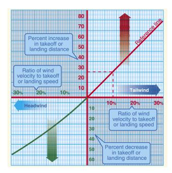
Figure 10-18. Effect of wind on takeoff and landing.
