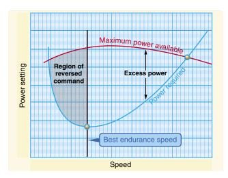
Figure 10-13. Power required curve.
