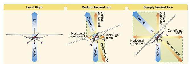
Figure 4-28. Forces during normal coordinated turn.
