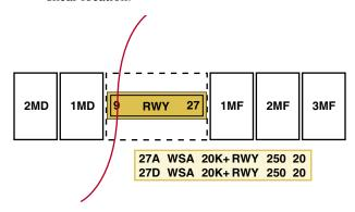
**Figure 12-7.** Example of what the controller sees on the ribbon display in the tower cab.
