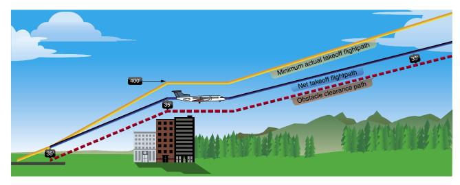
**Figure 10-37.** *Takeoff obstacle clearance.*
