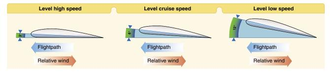
Figure 4-3. Angle of attack at various speeds.
