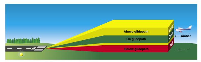
Figure 13-9. Tri-color visual approach slope indicator.
