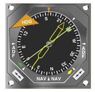
Figure 15-31. Radio magnetic indicator.
