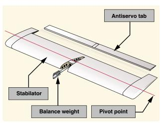
**Figure 5-13.** The stabilator is a one-piece horizontal tail surface that pivots up and down about a central hinge point.
