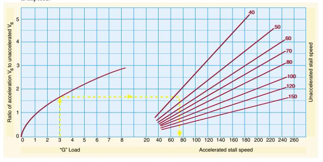
Figure 4-46. Load factor changes stall speed.
