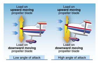
Figure 4-43. Asymmetrical loading of propeller (P-factor).
