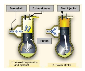
Figure 6-3. Two-stroke compression ignition.
