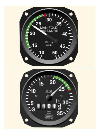
**Figure 8-4.** *Manifold pressure gauge (top) and tachometer (bottom).*
