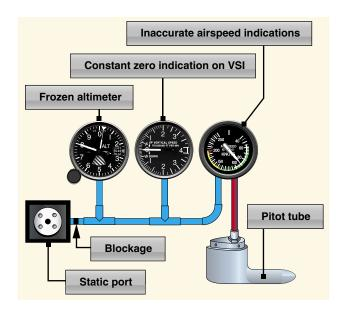
Figure 7-11. Blocked static system.
