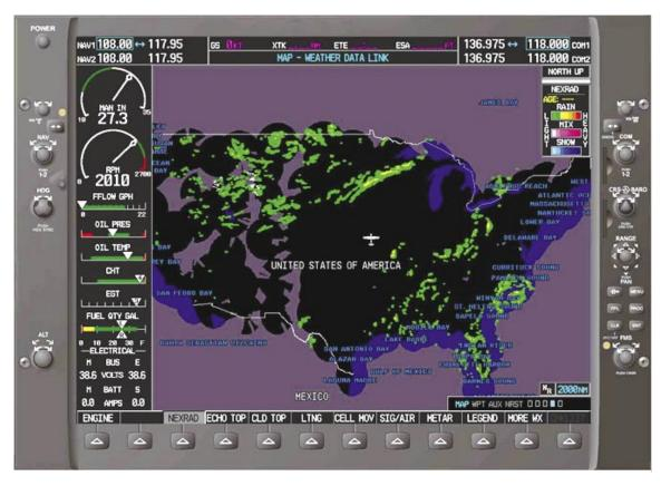
Figure 12-23. NEXRAD radar display.
