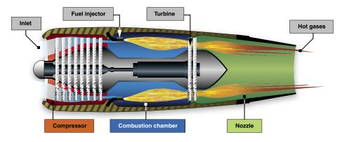
Figure 6-23. Turbojet engine.
