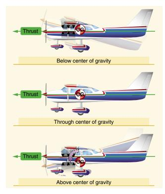
Figure 4-23. Thrust line affects longitudinal stability.
