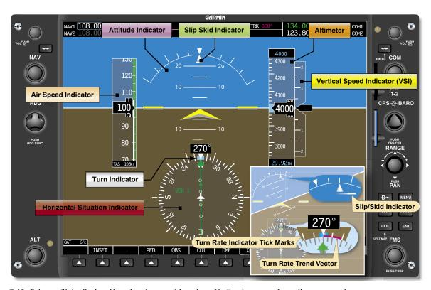
Figure 7-12. Primary flight display. Note that the actual location of indications vary depending on manufacturers.
