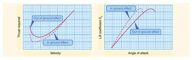
Figure 4-14. Ground effect changes drag and lift.
