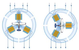
**Figure 7-28.** The current in each of the three pickup coils changes with the heading of the aircraft.
