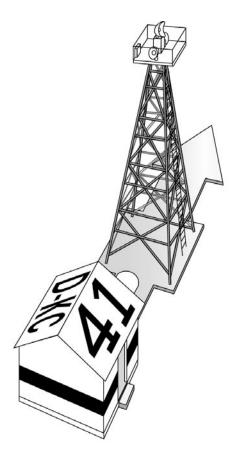
Figure 1-7. A standard airway beacon tower.
