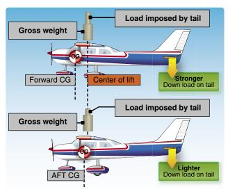
**Figure 4-55.** *Effect of load distribution on balance.*
