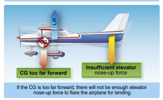
Figure 2-3. Center of gravity (CG).
