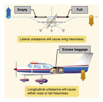
Figure 9-1. Lateral and longitudinal unbalance.
