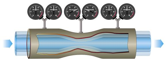
Figure 3-5. Air pressure decreases in a venturi tube.
