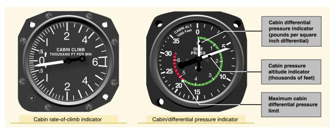
Figure 6-42. Cabin pressurization instruments.
