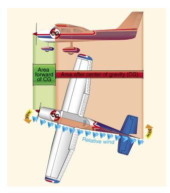
Figure 4-27. Fuselage and fin for vertical stability.
