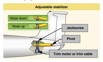
**Figure 5-23.** *Some airplanes, including most jet transports, use an adjustable stabilizer to provide the required pitch trim forces.*
