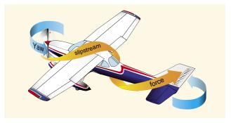
Figure 4-40. Corkscrewing slipstream.
