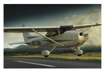
**Figure 6-37.** The landing gear supports the airplane during the takeoff run, landing, taxiing, and when parked.
