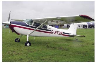
Figure 6-38. Tailwheel landing gear.
