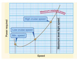
Figure 10-6. Power versus speed.
