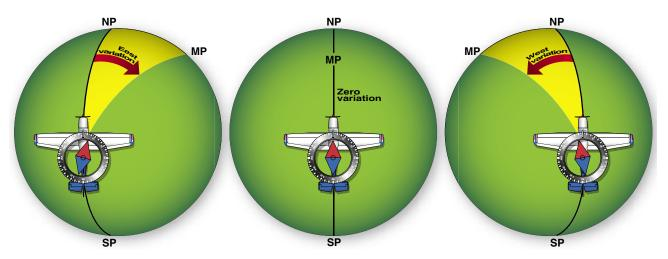
Figure 15-10. Effect of variation on the compass.
