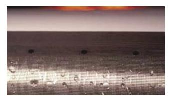
**Figure 6-48.** *TKS weeping wing anti-ice/deicing system.*
