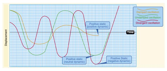
Figure 4-19. Damped versus undamped stability.
