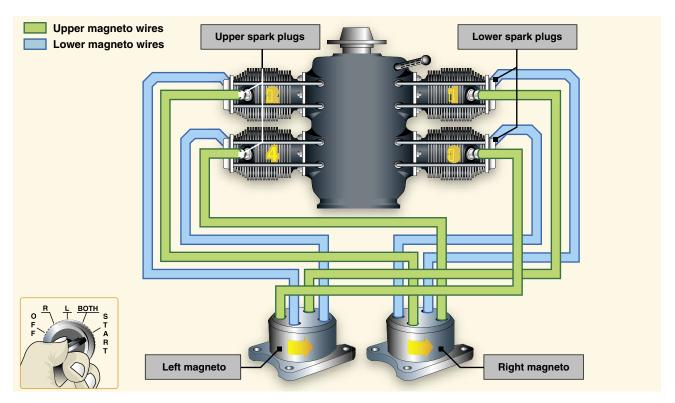
Figure 6-16. Ignition system components.
