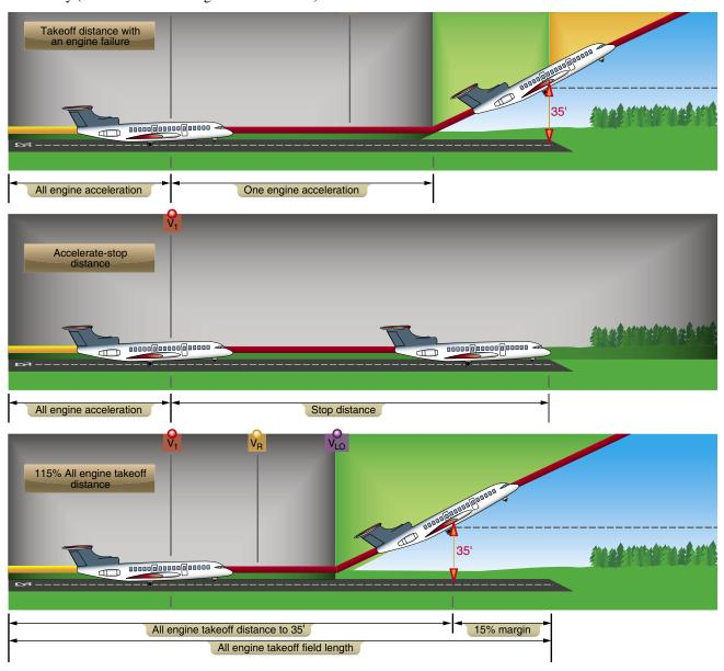
Figure 10-34. Minimum required takeoff.
