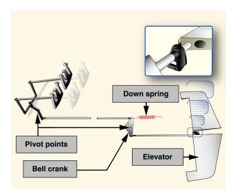
**Figure 5-12.** When the aerodynamic efficiency of the horizontal tail surface is inadequate due to an aft CG condition, an elevator down spring may be used to supply a mechanical load to lower the nose.
