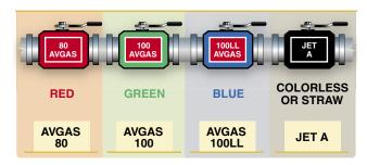
Figure 6-32. Aviation fuel color-coding system.
