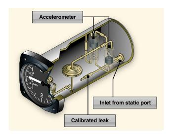
**Figure 7-6.** An IVSI incorporates accelerometers to help the instrument immediately indicate changes in vertical speed.
