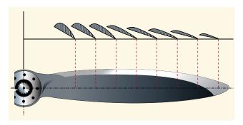
Figure 4-35. Airfoil sections of propeller blade.
