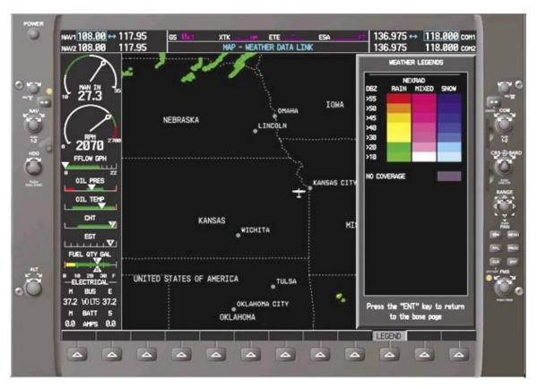
**Figure 12-25.** The AIRMET information box instructs the pilot to press the enter button to gain additional information on the selected area of weather. Once the enter soft key (ENT) is depressed, the specific textual information is displayed on the right side of the screen.
