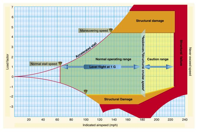
Figure 4-47. Typical Vg diagram.
