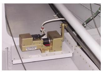
**Figure 5-24.** Basic autopilot system integrated into the flight control system.
