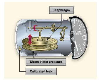
Figure 7-5. Vertical speed indicator (VSI).
