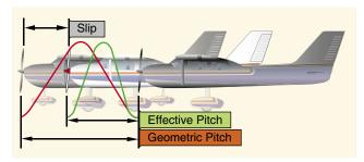
Figure 4-37. Propeller slippage.
