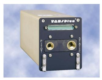
**Figure 7-15.** Teledyne's 90004 TAS/Plus Air Data Computer (ADC) computes air data information from the pitot-static pneumatic system, aircraft temperature probe, and barometric correction device to help create a clear picture of flight characteristics.
