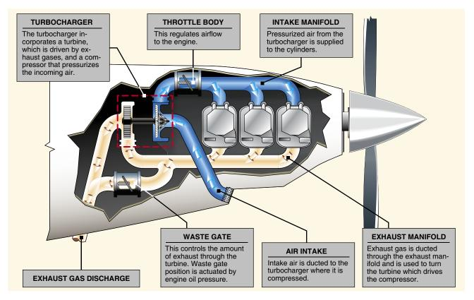
Figure 6-15. Turbocharger components.
