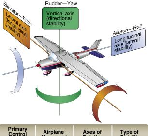
Type of Stability Control Movement Rotation Surface Aileron Roll Longitudinal Lateral Pitch Lateral Longitudinal Stabilator Rudder Yaw Vertical Directional
