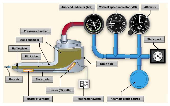
Figure 7-1. Pitot-static system and instruments.
