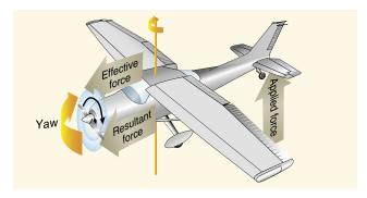
Figure 4-42. Raising tail produces gyroscopic precession.
