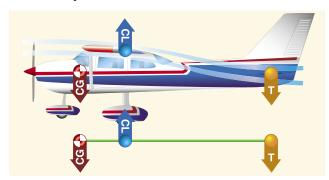
Figure 4-20. Longitudinal stability.
