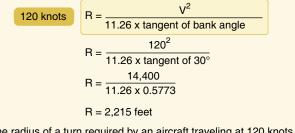
The radius of a turn required by an aircraft traveling at 120 knots and using a bank angle of  $30^{\circ}$  is 2,215 feet.
